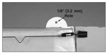
$\Box$  7. Drill two 1/8" [3.2 mm] holes in the mount. If not flying combat, use the two holes to route the antenna from the receiver.
