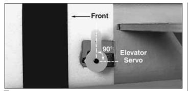
□ 4. Epoxy a servo into the bottom of the rear servo cutout from the left side of the plane. The output shaft should be toward the front of the fuselage. Center the servo with your radio and screw the extended arm onto the output shaft with the arm oriented straight up.
