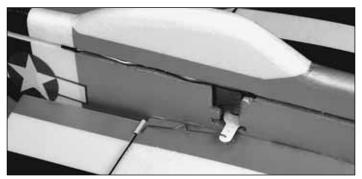
□ □ 1. Locate the two 2-3/4" [70 mm] prebent **aileron pushrods**. Slightly enlarge the outer hole on the aileron servo arm. Insert the Z-bend end of the pushrods into the outer hole on the aileron servo arm.
