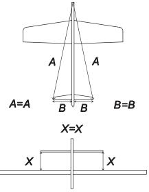
□ 1. Slide the stab into the slot in the rear of the fuselage. Center it as you did with the wing. Make sure the measurements shown in the sketches are equal. Glue the stab in place when satisfied with the fit.
