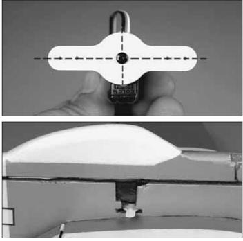
□ 6. Center your aileron servo with your radio and screw the extended double-sided arm onto the servo. When you glue the extended servo arm, be sure it is exactly centered as shown. Epoxy the aileron servo into the cutout in the fuselage.
