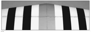
□ 3. Epoxy the foam inserts into the wing slot over the carbon joiner. Make sure they are fully seated against the joiner. The foam inserts may not be completely flush with the bottom of the wing.
