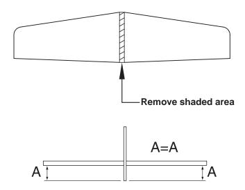
□ 3. Slide the wing out just enough to see the entire area covered by the fuselage. Remove the covering from the wing using a hobby knife 3/32" [2 mm] inside the marks you made. Apply a thin layer of epoxy and slide the wing into place. Use the marks from the previous step to align the wing. Clean up any excess glue with a paper towel. DO NOT use alcohol or any other solvent for cleanup as the paint finish will be affected.
