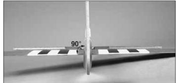
□ 4. Glue the fin and rudder to the fuselage with epoxy. Make sure that the fin remains perpendicular to the stab and centered on the fuselage.
