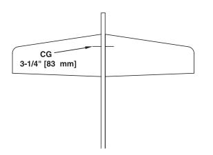
□ 1. Use a felt-tip pen or 1/8" [3 mm]-wide tape to accurately mark the C.G. on the top of the wing on both sides of the fuselage. The C.G. is located 3-1/4" [83 mm] back from the leading edge of the wing.
