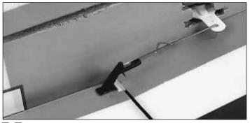
□ □ 6. Install a black nylon **snap keeper** onto the pushrod at the control horn.
