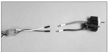
□ 1. Connect the output wires of your ESC to the motor. Check the direction of the motor before permanently installing it.
