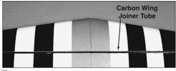
□ 2. Epoxy the 17-3/48" [451 mm] carbon wing joiner tube into the slot on the bottom of the wing. Make sure it is fully seated in the slot.
