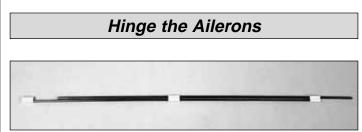
□ □ 1. Locate one of the carbon **wing hinge assemblies**. One of the carbon tubes is glued to the bearings; the other is free to rotate. Remove the loose carbon rod to prevent accidental gluing in the next steps.
