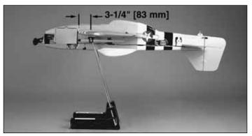
□ 2. With the wing attached to the fuselage and all parts of the model installed (ready to fly), place the model upside-down on a Great Planes CG Machine, or lift it upside-down at the balance point you marked.
