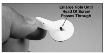
□ 1. Remove the screws and servo arms from all of your servos. Enlarge the hole in the center of the extender until the head of the servo screw fits through.
