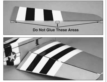
□ □ 4. Test fit an aileron onto the carbon rod as shown. If satisfied with the fit, glue the aileron to the carbon rod using CA. DO NOT glue the aileron to the bearings. The rod must freely rotate in the bearings, so the aileron must only be glued to the carbon rod.
