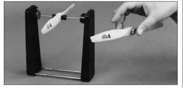
Carefully balance your propeller and spare propellers before you fly. An unbalanced prop can be the single most significant cause of vibration that can damage your model. Not only will motor mounting screws and bolts loosen, possibly with disastrous effect, but vibration may also damage your radio receiver and battery. When balancing the propeller that came with your Fun Force ARF, add tape to the light side of the propeller. Do not shave material away as is done with traditional propellers.
