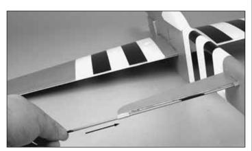
□ 2. Locate the 13.5" [343 mm] carbon **elevator rod**. Insert this rod into the preinstalled plastic bearings on the stab. DO NOT glue in place.
