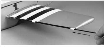
□ □ 3. Slide the loose carbon rod through the bearings.
