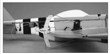
Use a Great Planes AccuThrow<sup>™</sup> (or a ruler) to accurately measure and set the control throw of each control surface as indicated in the chart that follows. If your radio does not have dual rates, we recommend setting the throws at the **low rate**, or sport rate setting.
