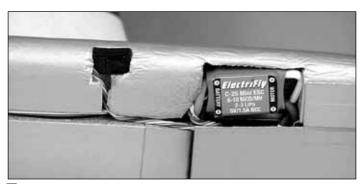
□ 2. Install the ESC as shown using a small section of hook and loop tape. Place the hard "hook" side in the provided cutout in the fuselage and the softer "loop" side on the back of the ESC. If your ESC has a BEC switch, install it in the provided cutout. For some electronic speed controls, it may be necessary to trim the foam slightly to allow for wire clearance and switch mounting.
