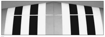
□ 1. Using epoxy, join the two **wing halves** together, making sure to align the root sections.
