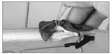
□ 2. Lay one end of a colored streamer over the mount. Insert one loop of the rubber band through the loop at the other end. Pull it tight to hold the streamer in place.
