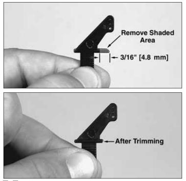
□ □ 3. Locate a black nylon **control horn**. Trim the small plastic section away as shown.
