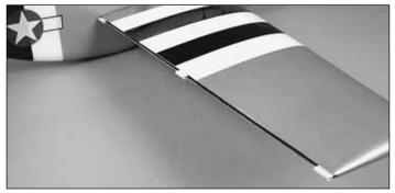
$\Box$  2. Test fit one of the wing hinges in the wing. The outer bearing should be flush with the wing tip. When satisfied with the fit, epoxy the hinge in place. Be careful to avoid getting epoxy into the open bearings.
