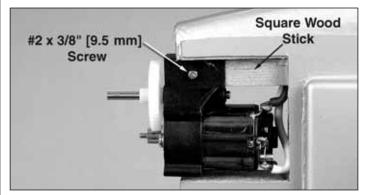
$\Box$  3. Slide the gearbox onto the square **wood stick** in the nose. Secure it with the supplied #2 x 3/8" [9.5 mm] screw.
