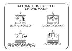
□ 3. Make certain that the control surfaces and the motor respond in the correct direction as shown in the diagram. If any of the controls respond in the wrong direction, use the servo reversing in the transmitter to reverse the servos connected to those controls. Be certain the control surfaces have remained centered. Adjust if necessary.
