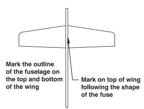
□ 2. Trace along the fuselage sides on the top and bottom of the wing with a felt-tip pen or a pencil.
