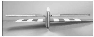
□ 3. Use foam-safe CA to glue one of the **elevator halves** to the carbon elevator rod. Then glue the other elevator to the carbon elevator rod. Be sure the two halves are even as shown.
