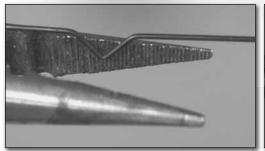
Secure the pushrod at the V bend with pliers.
