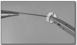
3. Twist the pliers holding the 90° bend in the proper direction to secure the pushrod to the control surface.
