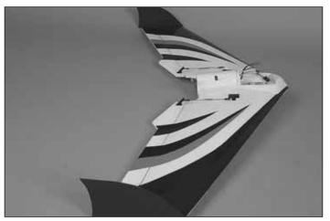
$\Box$  1. Use (4) #2 x 5/16" [8 mm] screws to attach the wing tips to the wing.
