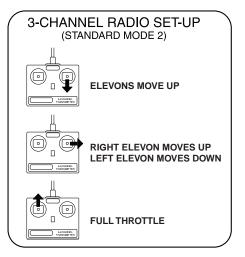
□ 3. Make certain that the control surfaces respond in the correct direction as shown in the diagram. If any of the controls respond in the wrong direction, use the servo reversing in the transmitter to reverse the servos connected to those controls. Be certain the control surfaces have remained centered. Adjust if necessary.
