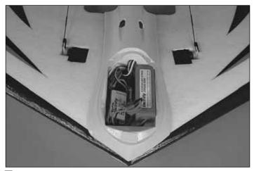
□ 3. Use the included hook and loop material to secure the battery pack, receiver, and ESC to the radio tray. You can also use optional double-sided servo tape. If using an auxiliary elevon mixer, place it into the tray at this time and check control surface operation with your radio. Computer radio systems equipped with an elevon function will not require a separate mixer to be installed.
