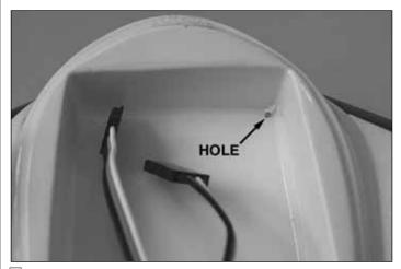
□ 3. Drill a 1.6 mm [1/16"] hole at an angle through the corner of the radio tray and out the bottom of the wing.
