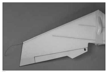
□ 5. Feed the receiver antenna through the hole and embed it in the slit. Cover the slit with transparent tape.
