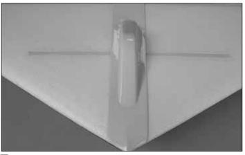
2. Install the sling handle on the underside of the wing in the same manner.
