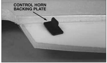
□ 3. Push the control horns through the cuts you made in the elevons. Press a **control horn backing plate** onto the underside of each control horn. Secure the backing plates and control horns to the elevons with foam safe CA glue.
