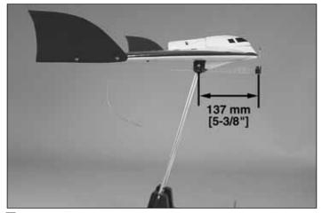
□ 2. With all of the parts of the model installed (ready to fly), place the model on a Great Planes CG Machine, or lift it at the balance point you marked.
