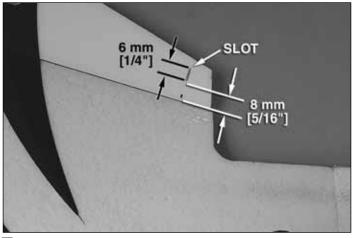
□ 2. Cut a 6 mm [1/4"] slot 8 mm [5/16"] aft of the hinge line for the **control horns**. Make the cuts so that the control horns will be **parallel** with the servo arms.
