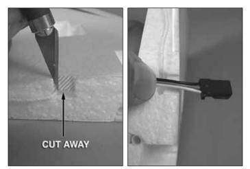
□ 2. Being careful not to sever the strings, cut away just enough foam above these channels at the wing roots to accommodate the thickness of the servo wires.
