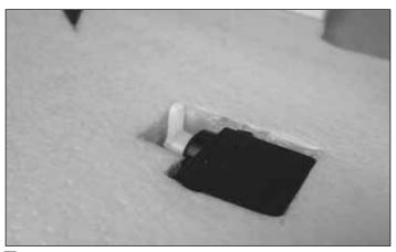
□ 7. Use epoxy to glue the servos into the servo bays. If you would like the servos to be easily removable from the Mini Slinger in the future, cover the servos in heat-shrink wrap (TRIC6074) prior to gluing. You will then be able to cut the heat-shrink to extract the servos from the wing with little damage.
