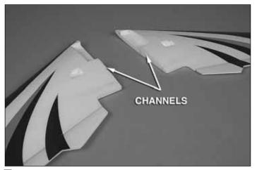
□ 1. Locate the channels in each **wing half** that contain the servo wire draw strings.
