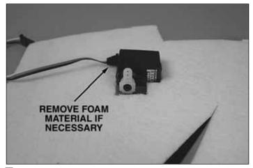
□ 5. Temporarily connect the servos to your radio system. Turn the transmitter on and center your trim levers. With the radio on, position the arms perpendicular to the servos. Make a left and a right servo. If the servo model you are using has the servo lead exiting from the side of the servo case as shown in the picture above, use a hobby knife to remove material from the servo bay in the wing until it fits properly.
