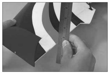
Use a ruler to accurately measure and set the control throw of each control surface as indicated in the chart that follows. If your radio does not have dual rates, we recommend setting the throws at the **low** rate setting.
