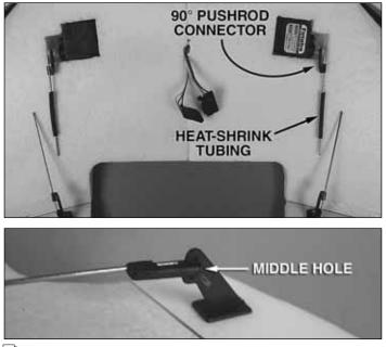
■ 4. Locate the four 2-1/2" [64mm] pushrods and two 1" [25mm] long pieces of heat shrink tubing. Using the 90° pushrod connectors, attach a pushrod to the outer hole of each servo horn and the middle hole of each control horn. If necessary, use a 1/16" [1.6mm] drill bit to enlarge the holes. Insert a piece of heat shrink tubing onto the two pushrods attached to the servo horns.
