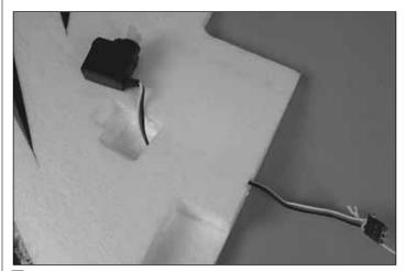
□ 6. Use the strings to pull the servo leads through the wing panels.
