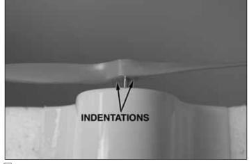
□ 2. Press the propeller onto the motor shaft. The two indentations at the center of the prop should face the model.
