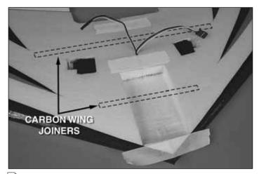
□ 2. When the epoxy has cured, mix another batch and coat the other ends of the carbon tubes and the roots of the wing panels. Slide the panels together making sure the servo leads exit on top of the wing and use tape to hold them tight while the epoxy cures. Wipe away any excess epoxy that squeezes out.
