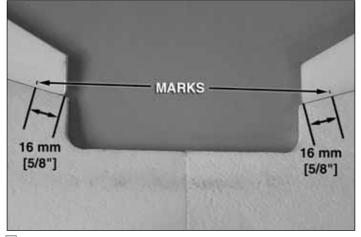
□ 1. Measure 16 mm [5/8"] from the inside edge of each **elevon** and make a mark as shown in the picture.
