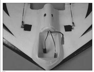
□ 1. Using rubbing alcohol, clean the area where the **radio tray** will be installed. Feed the servo wires through the hole in the hatch. Peel the paper backing from the tape on the underside of the radio tray hatch and press it into position. Be sure that the hatch is held securely in place by the tape.
