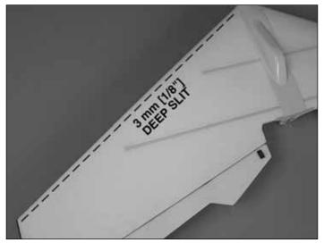
↓ 4. With a sharp hobby knife, cut a 3 mm [1/8"] deep slit on the underside of the wing from this hole to the end of the wing parallel with the leading edge.
