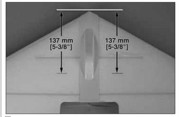
□ 1. Use a felt-tip pen or 3 mm [1/8"]-wide tape to accurately mark the C.G. on the bottom of the wing as shown. The C.G. is located 137 mm [5-3/8"] back from the leading edge of the wing.
