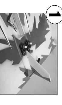
Glue the two servos in place with foam safe CA as shown.
