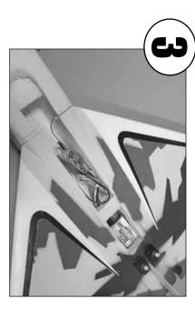
Make a small hole on the side of the fuselage and slide the receiver antenna through it. Tape the antenna to the leading edge of the wing.
