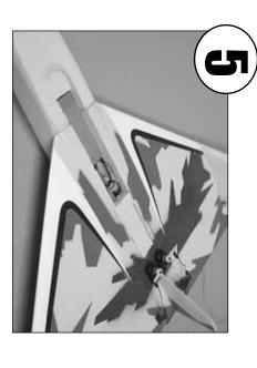
Install the motor battery, canopy and receiver hatch. Adjust the elevons' neutral point, the throws and the CG.
