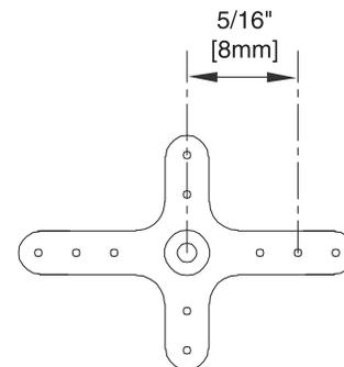
❑ 3. Same as when hooking up the elevator and rudder servos, and with the propeller off the motor, connect the aileron servo to the extension coming from the receiver and turn the system on. Make sure the aileron trim is centered and place the servo arm on the servo so it will be 90-degrees. Mount the two remaining screw-lock pushrod connectors to the servo arm—only this time mount them 5/16" [8mm] from the center of the arm to achieve the correct throw.
