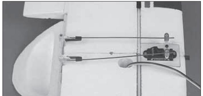
❑ 2. The same as you mounted the rudder and elevator servos in the fuse, mount the aileron servo in the wing—only this time use a drill **no larger** than a #58 (.042") [1.07mm] for the servo screw mounting holes. If you don’t have the right drill you could use the tip of a #11 blade to make the holes instead. If you do accidentally oversize the holes, they may be filled with medium CA and redrilled.
