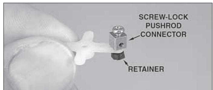
❑ 3. If necessary, use a hobby knife to carefully enlarge the hole in the elevator servo arm. Then connect a small, brass
