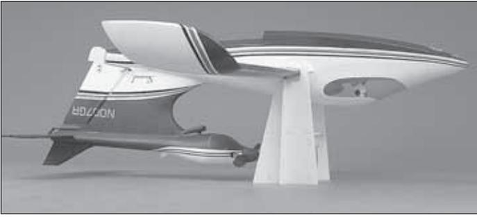
❑ 2. Place the model upside-down on the balance stand as shown. The leading edge of the wings should contact the vertical “stop” on the stand, thus supporting the wing on the correct C.G. location which is 1" [25mm] from the leading edge.
