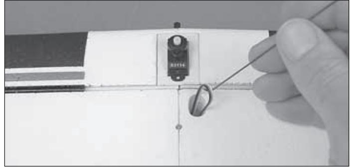
❑ 1. Use a brass tube sharpened on the end or a hobby knife to cut a hole in the bottom of the wing where shown for the aileron servo wire. Use one of the aileron pushrod wires with the 90° bend on the end to pull the servo wire up through.
