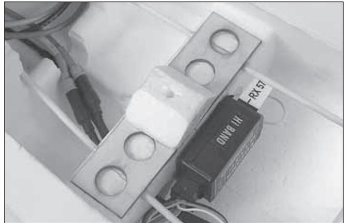
❑ 1. Test fit the wing to the fuse. If necessary, trim the foam block on top of the plywood wing bolt plate in the fuse so it doesn't interfere with the aileron pushrod wires when you mount the wing.
