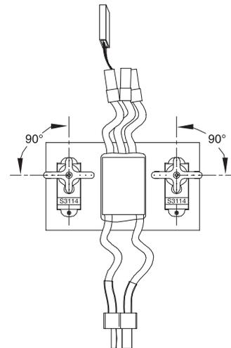
❑ 2. With the transmitter on, the trims centered and the motor battery connected to the receiver, fit the servo arms on the rudder and elevator servos so the arms will be 90-degrees (or as close as 90-degrees as possible) to the servos.
