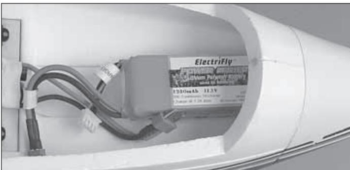
❑ 14. Mount the motor battery as far forward as possible in the fuse with one strip of the included Velcro on the battery and the opposing strip in the bottom of the fuse.
