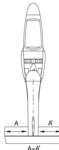
❑ 4. Taking accurate measurements, center the stab in the fuselage from side-to-side.
