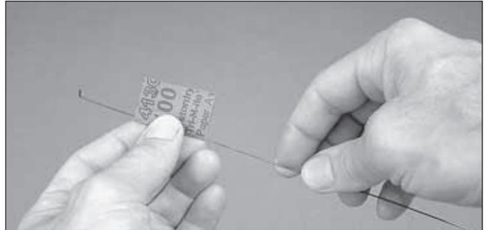
❑ 2. Use fine-grit sandpaper with household oil to clean any deposits or oxidation from both wires. This will allow the wires to move as freely as possible in the guide tubes.
