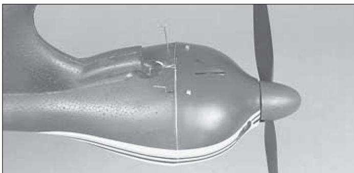
❑ 12. Drill the holes for the remaining two cowl mounting screws and insert the screws. Remove the pins.
