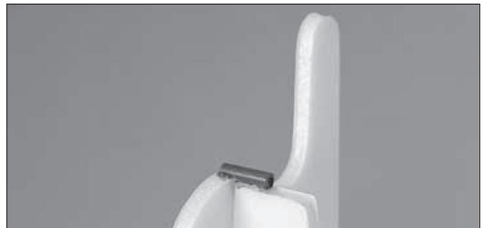
1. Glue together the balance stand as shown. Glue the 3mm carbon tubes to the top of the stand.
