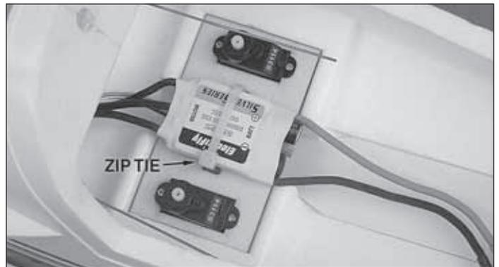
❑ 5. Test fit your elevator and rudder servos in the plywood servo tray. Drill small holes in the servo tray for the small wood screws supplied with this kit for mounting the servos. Any drill from a #60 (.040") [1mm] up to a #52 (1/16") [1.6mm] can be used, but drills nearer the smaller end of the size range will be best.
