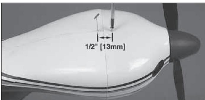
❑ 11. Drill a 1/16" [1.6mm] hole through the cowl and the cowl mounting block 1/2" [13mm] ahead of the pin in the top of the motor pod—this should put the screw hole right in the middle of the cowl mounting block. Screw in one of the three larger wood screws that came with this kit.
