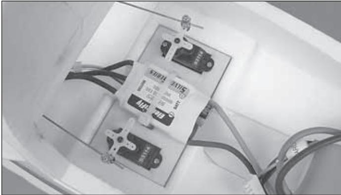
❑ 4. Slip the elevator pushrod into the connector on the servo arm. Then mount the servo arm to the elevator servo and secure it with the screw that came with the servo.
