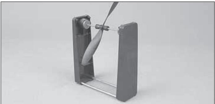
❑ 1. For optimum performance and motor efficiency balance the propeller using a Top Flite® Precision Magnetic Prop Balancer (TOPQ5700) or other suitable balancer. Use a hobby knife or sandpaper to sand the one side of the heavier blade until you can get the prop to balance.
