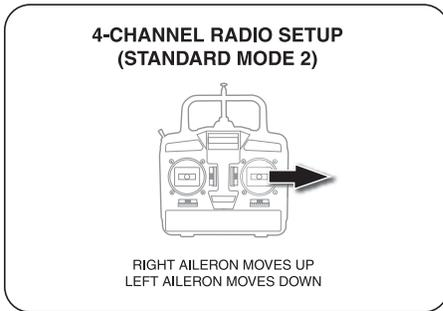
❑ 6. Use the transmitter to operate the ailerons to make sure they respond in the correct direction. You can set the control throws now, or wait until you get to the **“Set the Control Throws”** section on page 12.
