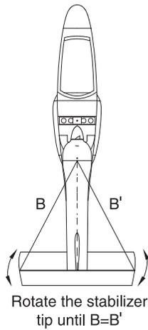
❑ 5. Square the stab with the centerline of the fuselage by taking accurate measurements from both tips to the seam between the two fuselage halves on the top of the motor pod behind the cowl. Rotate the stab as shown to equalize both sides. Make sure the stab has remained centered laterally.
