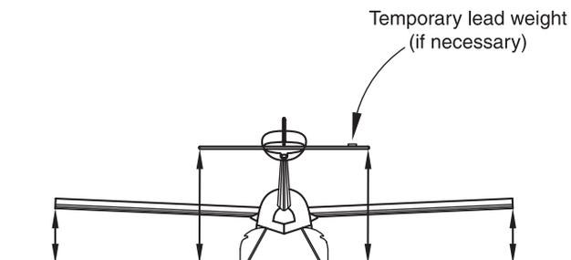
❑ 1. Temporarily mount the wing to the fuselage. With the plane resting in its building cradle, measure the distance from the bottom of both wing tips down to your workbench. Adjust the plane in the cradle until both distances are equal.
