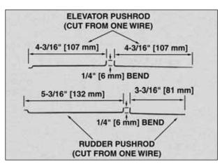
☐ 1. On page 11, step 2 below "Build the Pushrods" should read as follows: Cut the 8-7/8" [225 mm] elevator and rudder pushrods into the lengths shown in the picture above. Make a 1/4" [6 mm] long 90° bend at each end of the cuts. One 8-7/8" [225 mm] pushrod wire will remain uncut for the steerable nose gear.
