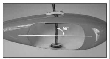
□ □ 7. Remove one of the screws from the landing gear strap and slide a round plywood wheel pant retainer onto the landing gear. Re-attach the landing gear strap. Align the axle of the landing gear so that it is perpendicular to the centerline of the wheel pant. Apply a thin coat of oil or petroleum jelly on the axle to prevent the epoxy from adhering. Roughen the inside of the wheel pant and glue the wheel pant retainer to the wheel pant with epoxy.
