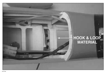
☐ 7. To prevent the battery from sliding around, glue a piece of hook-and-loop material to the battery tray between the former. Glue a corresponding piece of hook-and-loop material to the battery.
