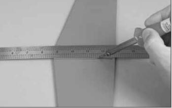
Use a 25 watt soldering iron to cut the covering from the stab. The tip of the soldering iron doesn't have to be sharp, but a fine tip does work best. Allow the iron to heat fully. Use a metal straightedge to guide the soldering iron at a rate that will just melt the covering and not burn into the wood. The hotter the soldering iron, the faster it must travel to melt a fine cut. Allow the heat to melt the covering. Do not apply much pressure or the wood may be damaged. Peel off the covering.
