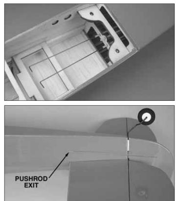
□ 1. Insert the two wire pushrods into the outer pushrod tubes inside the fuselage. Notice at the aft end of the fuselage
