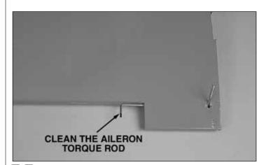
□ □ 5. Clean the aileron torque rod with denatured alcohol to remove any contaminants.
