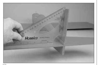
☐ 12. Glue the fin into position using epoxy. Use a builders square to make sure the fin is perpendicular to the stab. Wipe off the excess epoxy with a paper towel dampened with denatured alcohol. Masking tape can be used to hold the fin in position until the epoxy cures.
