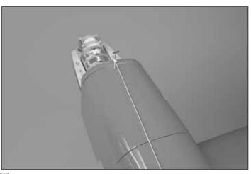
□ 3. Stick a T-pin into the center of the top of the firewall. Tie a small loop in one end of a 36" [910mm] piece of nonelastic string such as K&S #801 Kevlar thread. Slip the loop in the string over the T-pin.
