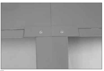
□ 2. Test fit the wing to the fuselage and bolt it into position with two 3x30mm machine screws and 3mm washers.
