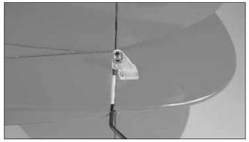
□ 5. Install the rudder control horn following the same procedure. Make sure that the control horn does not interfere with the elevator.
