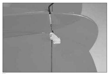
□ 3. Mark the two control horn mounting holes on the elevator. Remove the control horn and drill 5/64" [2mm] holes through the elevator at the marks. Mount the control horn with two 2x10mm machine screws and the nylon mounting plate on the top side of the elevator.
