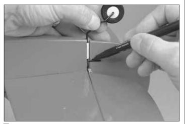
□ 18. Use epoxy to glue the tail gear wire bushing in the lower slot at the aft end of the fuselage. Temporarily install two CA hinges in the rudder and install the rudder on the fin. Mark the bend in the tail gear wire on the rudder.
