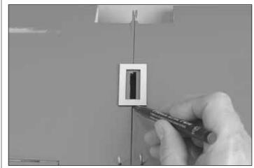
□ 4. Position the plywood aileron servo tray, centered over the opening in the top of the wing. Use a fine-tip marker to trace around the inside and outside of the tray.
