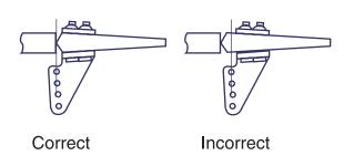
□ 2. Remove and reinstall the pushrods so that the L-bends are at the aft end of the fuselage. Install a nylon control horn on the end of each pushrod. Position the control horn so that the attachment holes are aligned with the hinge line of the elevator.
