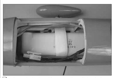
■ 6. Insert the hook-and-loop strap through the slot in one side of the battery tray and bring it out the slot in the other side of the tray. Adjust it so that the overlap is under the tray. Install the battery in the battery compartment and secure it with the hook-and-loop strap. Trim off the excess hook-and-loop material.
