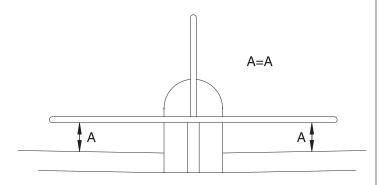
□ 5. View the stab from approximately 10' [3m] behind the plane. Check that the stab is parallel with the wing. If it is not, lightly sand the stab saddle until the stab is parallel with the wing.
