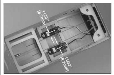
□ 1. Install servo arms on the rudder and elevator servos. The pushrod mounting holes should be approximately 11/32" [8.7mm] from the center of the servo arm. Install the rudder and elevator servos in the servo tray, aligning the hole in the servo arm with the pushrod wire. Use the hardware included with the servos to mount the servos to the tray. After installing the servo mounting screws, remove them, apply a drop of CA to each hole to harden the threads, then reinstall the screws.
