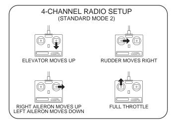
□ 3. Make certain that the control surfaces respond in the correct direction as shown in the diagram. If any of the controls respond in the wrong direction, use the servo reversing in the transmitter to reverse the servos connected to those controls. Be certain the control surfaces have remained centered. Adjust if necessary.
