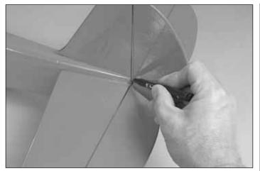
□ 16. Position the rudder at the trailing edge and mark the location where the elevator joiner wire passes through the leading edge of the rudder.
