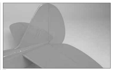
□ 20. Once satisfied with the fit of the tail gear wire in the rudder, apply epoxy in the tail gear wire hole in the leading edge of the rudder. Join the rudder to the fin using two CA hinges. Before the epoxy cures, use thin CA to glue the CA hinges in the rudder and fin following the same procedure used for the ailerons.
