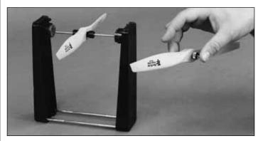
Carefully balance your propeller and spare propellers before you fly. An unbalanced prop can be the single most significant cause of vibration that can damage your model. Not only will motor mounting screws and bolts loosen, possibly with disastrous effect, but vibration may also damage your radio receiver and battery.
