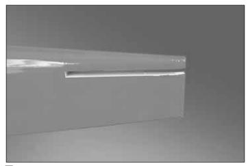
□ 1. Using a sharp hobby knife, remove the covering from the stabilizer slot at the aft end of the fuselage. Also remove the temporary balsa block.
