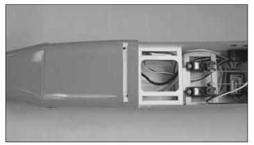
□ 1. Trim the covering from the main landing gear slot in the bottom of the fuselage.
