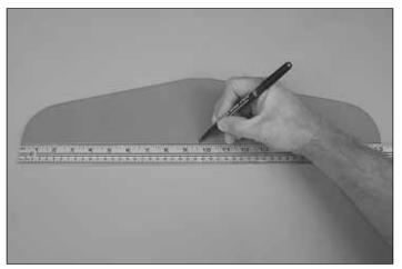
□ 2. Mark the center of the trailing edge of the stabilizer. Insert the stabilizer into the slot.
