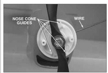
□ 4. In the side of the collet is a small hole. Insert the provided wire in the hole and tighten the prop nut. Make sure that the prop is centered between the two spinner nose cone guides.
