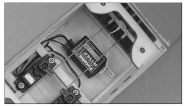
□ 2. Cut a piece of soft hook-and-loop material and use CA to glue it to the bottom of your receiver. Cut an opposite piece of the hook-and-loop material and glue it in the fuselage behind the servo tray. Insert the receiver antenna into the third pushrod tube and route it out the bottom of the fuselage. You will need to cut a slit in the covering material where the antenna exits the bottom of the fuselage. Plug the rudder and elevator servos into the receiver.
