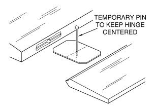
□ □ 4. Test fit the ailerons to the wing with the hinges. If the hinges don't stay centered, stick a pin through the middle of the hinges to hold them in position.
