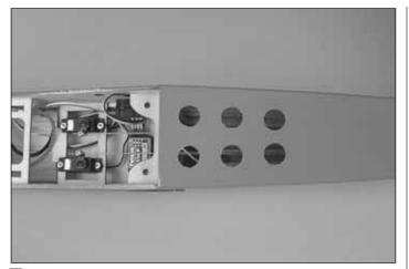
■ 8. To provide an exit for the cooling air, trim the covering from the six holes in the bottom of the fuselage, behind the wing saddle.
