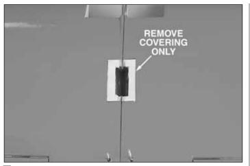
□ 5. Using a sharp hobby knife, cut the covering and balsa sheeting from the inside of the aileron servo tray area. Trim only the covering from the outer aileron servo tray area.
