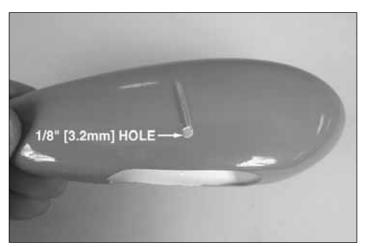
$\Box$  4. Starting with the left wheel pant, drill a 1/8" [3.2mm] hole in the wheel pant at the bottom of the mounting slot.
