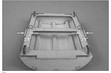
■ 2. Using a T-pin, make two small pilot holes in the base of the battery hatch cover 3/8" [9.5mm] from the edge. Screw the two eye hooks into the holes leaving enough space to attach rubber bands to the eye hooks.
