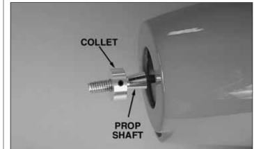
□ 2. Slide the prop shaft and collet onto the output shaft of the gear drive. The collet has a tapered hole through it. The side with the larger hole goes on first.
