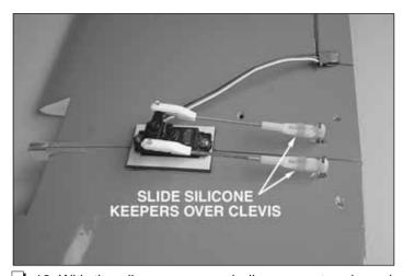
□ 12. With the aileron servo and ailerons centered, mark the aileron pushrods where they cross the aileron servo arm. Make a 90° bend at the marks and cut the pushrods 3/8" [10mm] past the bend. Attach the pushrods to the aileron servo arm with nylon snap keepers. Cut off the excess threads on the aileron torque rods.
