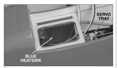
□ 3. Use CA to glue a 1-1/2" [40mm] piece of the "soft" hookand-loop material to the top of the ESC. The bottom of the ESC has the blue heat sink on it. The blue heat sink must not be covered so that it can dissipate the heat from the ESC. Glue a 1-1/2" [40mm] piece of the "hard" hook-and-loop material between the stringers on the side of the fuselage in front of the servo tray. Install the ESC in the fuselage.
