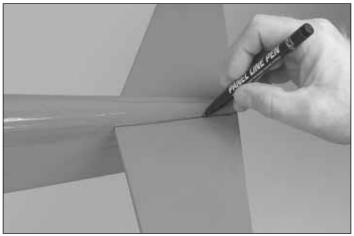
□ 6. Use a fine-point felt-tip pen to mark the outline of the fuselage onto the bottom and top of the stab.
