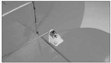
↓ 4. Connect the pushrod wire to the control horn with a 1.7mm wheel collar and 2.5mm set screw.
