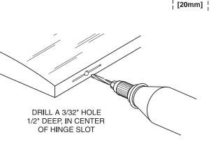
□ □ 2. Drill a 3/32" [2.4mm] hole, 1/2" [13mm] deep in the center of each hinge slot to allow the CA to "wick" in. Follow-up with a #11 blade to clean out the slots. **Hint:** If you have one, use a high-speed rotary tool to drill the holes.
