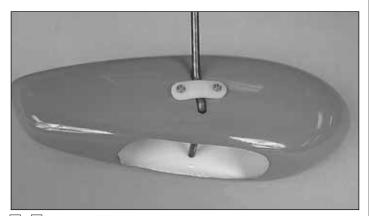
□ □ 6. Once the epoxy has cured, slide the wheel pant onto the main landing gear. Position a nylon landing gear strap over the main landing gear and drill 1/32" [.8mm] holes through the strap and the plywood mounting plate. Attach the landing gear strap to the wheel pant with two 2.5x8mm self-tapping screws. Harden the holes with thin CA.
