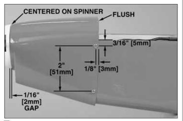
☐ 7. Drill four 1/16" [1.6mm] holes through both sides of the cowl and the fuselage where shown in the photo. Remove the cowl and enlarge the holes in the cowl only with a 3/32" [2.4mm] drill. Mount the cowl with four 3x10mm screws.
