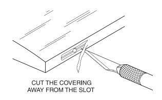
□ □ 3. Use a sharp #11 blade to cut a strip of covering from all the hinge slots in the wing half and aileron.
