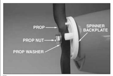
□ 3. Install the spinner backplate, prop, prop washer and prop nut on the prop shaft. The back of the prop has two indentations in the hub.
