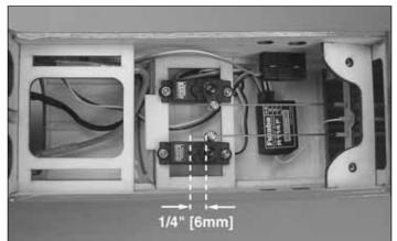
☐ 7. Center the elevator and rudder, then tighten the 3mm screws in the pushrod connectors. Trim off the excess pushrod wires 1/4" [6mm] past the pushrod connectors.
