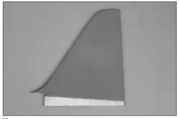
☐ 11. Fit the fin all the way into the fin slot. Again, use a felttip pen to mark the fuselage onto the fin. Remove the fin from the fuselage and remove the covering from the fin.
