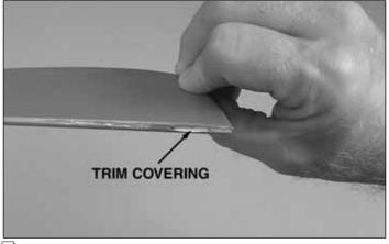
□ 13. Trim the covering from the elevator joiner wire slot in the leading edge of both elevator halves.
