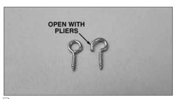
1. Use a needle-nose pliers to open the two eye hooks.
