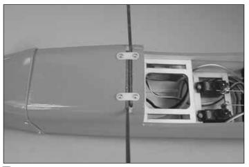
□ 3. Position two nylon landing gear straps over the landing gear. Drill a 1/16" [1.6mm] hole through each mounting hole in the landing gear strap and into the fuselage. Attach the landing gear straps to the fuselage with four 3x10mm self-tapping screws. Harden the holes with thin CA.
