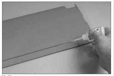
□ □ 7. Apply six drops of thin CA to the top and bottom of each hinge. Do not use CA accelerator. After the CA and epoxy have fully hardened, test the hinges by pulling on the ailerons.
