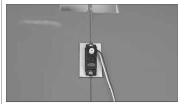
■ 8. Mount the aileron servo in the wing. Use CA to harden the threads. Plug a 6" [150mm] aileron servo extension into the receiver. Connect the aileron servo to the servo extension and switch on the transmitter and ESC. Center the aileron servo trim.
