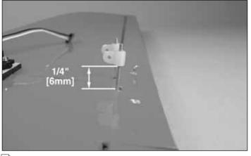
□ 10. Thread the two nylon torque rod horns onto the aileron torque rods. The bottom of the horn should be approximately 1/4" [6mm] from the wing.
