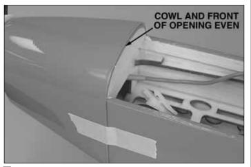
□ 6. Tape the cowl to the fuselage so that the aft edge is flush with the front of the battery hatch. Make certain there is an approximately 1/16" [2mm] gap between the spinner and cowl and the cowl is centered on the spinner.
