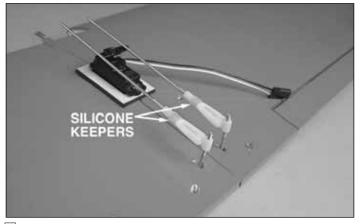
□ 11. Thread a nylon clevis 14 turns onto the end of the two  $2-56 \times 4"$  [100mm] aileron pushrods. Attach the clevises to the torque rod horns. Slide a silicone clevis keeper on each clevis.
