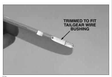
□ 19. Drill a 3/32" [2.4mm] hole into the leading edge of the rudder at the mark. Cut a slot in the leading edge of the rudder to clear the tail gear wire bushing.
