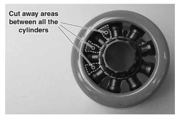
To prevent motor overheating when flying in warm weather we recommend that you cut the area away between the cylinders of the dummy engine. This is best accomplished by cutting the material with a hobby knife or Dremel Tool, cutting inside the cowl and cutting the material away from the back side of the dummy engine.
