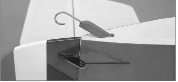
□ 4. Test fit the **tail skid** into the bottom of the fuselage. Note how the notch in the end of the skid should catch another notch in a plywood plate inside the fuselage. Once you see how the skid fits, remove the skid and glue it into position with medium CA.
