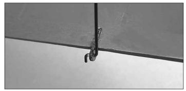
□ 2. Fit one aileron pushrod into the tab in the top aileron and another aileron pushrod into the tab in the bottom aileron on one side of the wing.
