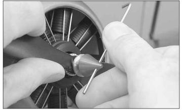
□ 2. Mount the propeller with the propeller washer and propeller nut. Tighten the nut with an 8mm or 5/16" wrench. Install the aluminum propeller cone and tighten with a piece of wire through the hole in the front.
