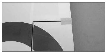
□ 5. Hold the aileron centered to the wing with a small piece of masking tape.
