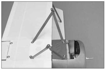
□ 1. Mount the front and rear landing gear struts to the bottom of the fuselage with six  $#2 \times 3/8"$  [10mm] flat-head Phillips screws. Do not tighten the screws all the way yet. The struts should be loose.
