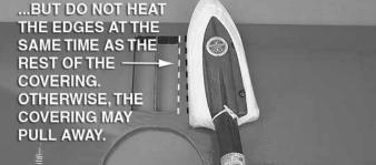
□ 1. Use a covering iron set to approximately 250 to 300 degrees F [120 to 150 degrees C] with a protective covering sock to remove any wrinkles and tighten the covering wherever it looks loose. Be careful along edges and seams-if an edge or seam is heated at the same time as the rest of the covering, it may pull away when it shrinks.
