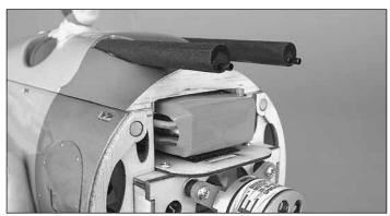
□ 5. Test fit the cockpit hatch to the fuselage to make sure it fits over the battery. Make any adjustments necessary.
