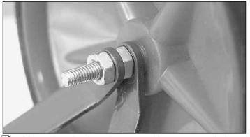
□ 2. Mount the wheels to the struts with a 3 x 25mm bolt and two 3mm nuts. Use threadlocker and tighten the nuts to the struts, but make sure the wheels can roll freely.
