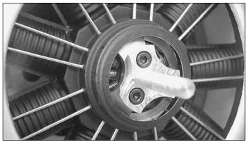
□ 7. Use a hobby knife or a rotary tool with a drum sander to enlarge the opening in the replica engine until it fits over the motor.
