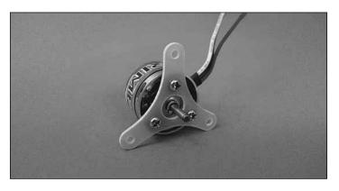
**Step 3.** Apply thread locking compound to the three **3 x 4mm** machine screws that came with your motor and use these to attach the Y-mount supplied with this ARF to the motor.
