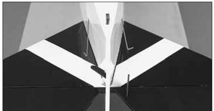
3. Insert the two 460mm [18"] wire pushrods into the outer pushrod tubes at the rear of the fuselage as shown.
