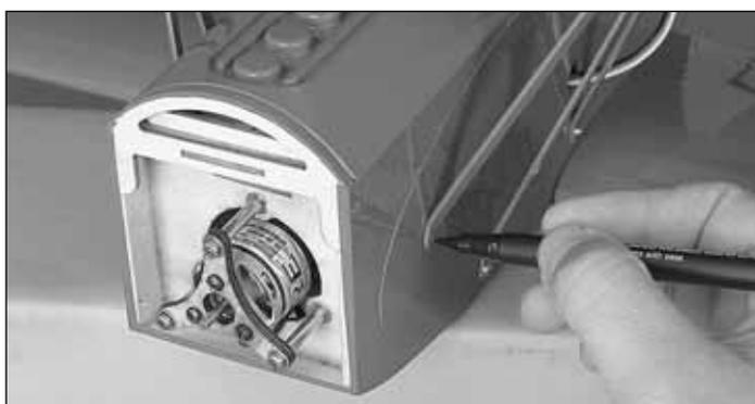
❑ 9. Glue the cheek vents in place as shown. You will need to remove the screw from the front of the "V" strut and slide the cheek in place. Use a felt-tip pen to make a mark to show where to drill. Once the hole is drilled, simply slide the cheek vent in place and re-install the 2mm x 7mm [5/64" x 9/32"] self-tapping washer head screw.
