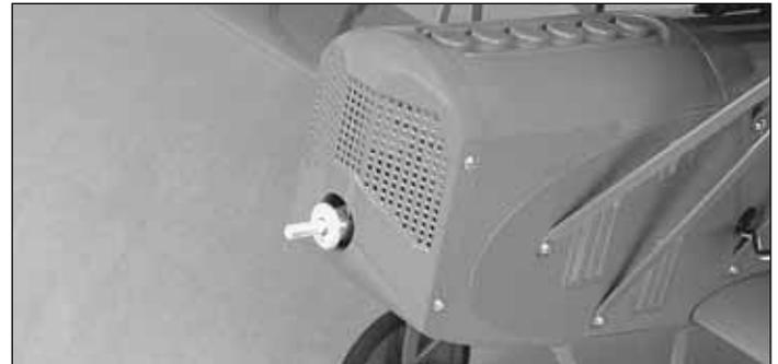
9. Slide the prop shaft and collet onto the motor shaft. The collet has a tapered hole through it.
