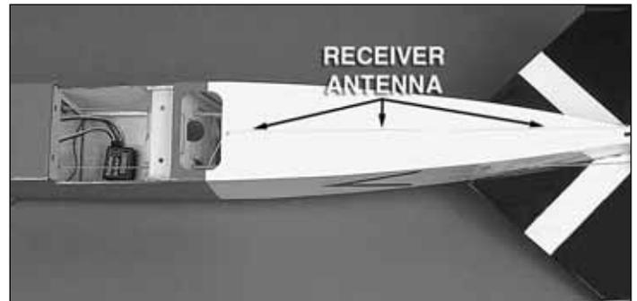
❑ 13. Make a small hole in the bottom sheeting. Route the antenna out of the hole and tape it to the bottom of the fuselage.
