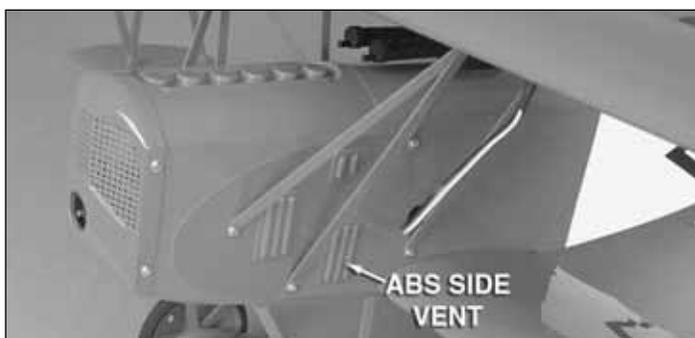
❑ 10. Use CA to glue one ABS side vent on each side of the fuselage as shown.
