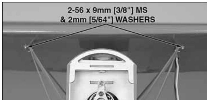
❑ 6. Attach the top wing to the center cabanes with two 2-56 x 9.5mm [3/8"] machine screws and two 2mm [5/64"] washers as shown.
