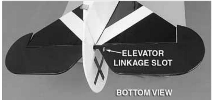
1. Use a sharp hobby knife to trim the covering from over the small rectangular holes towards the LE of the rudder and the bottom of the elevator as shown. Do not cut all the way through the rudder or elevator.
