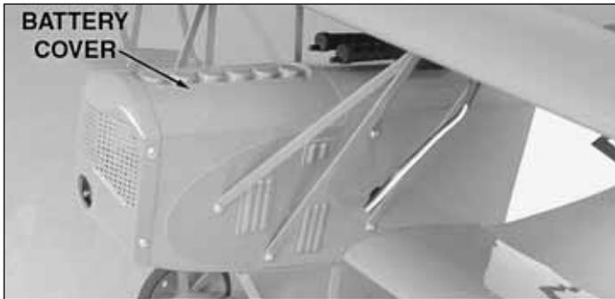
6. Put the battery cover in place. The battery cover has three very small but powerful magnets that will hold it in place.
