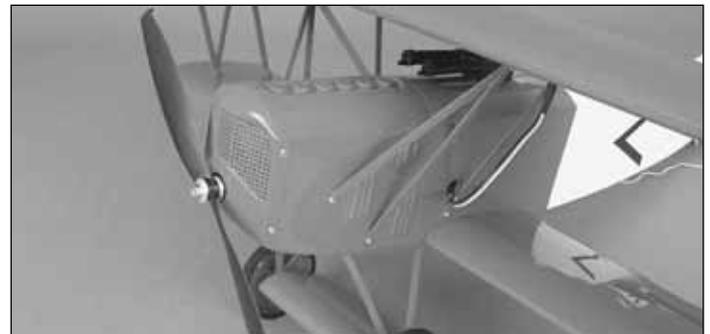
10. Install a 10x4.5 propeller. Install the prop washer and prop nut and tighten the nut securely.
