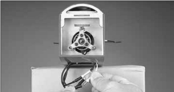
5. Install a 3.5mm [9/64"] Bullet (male) to 2mm [5/64"] Bullet (female) connector adapter (GPMM3122) on each of the motor leads. Connect the motor leads to the ESC. Push the wires up into the fuselage to prevent them from contacting the rotating motor case.
