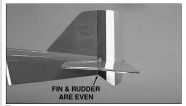
□ 13. Install three CA hinges in the rudder and test fit it on the fin. Adjust the position of the fin so that the bottom of the rudder is even with the bottom of the fuselage and the LE of the rudder and the TE of the fin are aligned.
