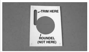
$\Box$   $\Box$  6. Trim the covering from over the pushrod exit on the aileron servo hatch.
