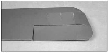
□ □ 2. Remove any pins you may have inserted into the hinges. Adjust the aileron so there is a very small gap between the LE of the aileron and the wing. The gap should be small – just enough to see light through or to slip a piece of paper through.
