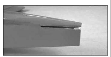
□ 1. Using a sharp hobby knife, remove the covering from the stabilizer slot at the aft end of the fuselage. Also remove the temporary balsa block.
