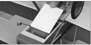
□ 8. Slide the battery hatch into position. Note that the lip slides under the front of the fuselage and the aft end is held on with two magnets.
