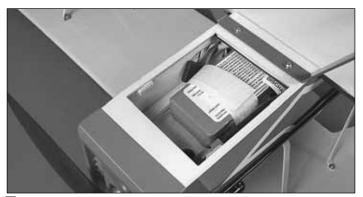
□ 7. Insert the battery in the battery compartment and secure it with the hook and loop material. Trim the excess hook and loop material.
