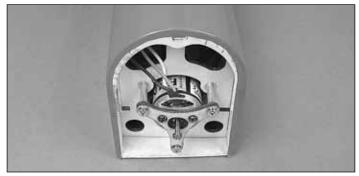
□ 4. Install a 3.5mm Bullet (male) to 2mm Bullet (female) connector adapter (GPMM3122) on each of the motor leads. Connect the motor leads to the ESC. Then, stuff the wires into the fuselage to prevent them from contacting the rotating motor case.
