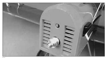
$\Box$  5. Slide the prop shaft and collet onto the output shaft of the gear-drive. The collet has a tapered hole through it. The side with the larger hole goes on first. Use clear tape to attach the radiator to the front of the fuselage so that the prop adapter is centered in the opening of the radiator.
