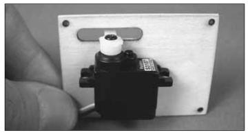
□ □ 8. Clean the servo case with denatured alcohol. Use CA to glue the aileron servo on the bottom of the aileron servo hatch so that the servo arm is centered in the opening. If you prefer, wrap electrical tape or heat-shrink tubing around the servo before gluing it to the servo hatch. This will allow the servo to be easily removed.
