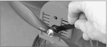
$\Box$  6. Remove the prop nut and washer and install the 10x4.5 propeller. Reinstall the washer and prop nut and tighten the nut securely.
