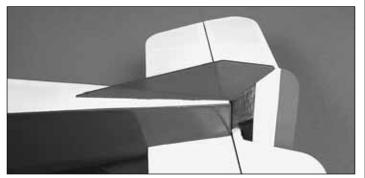
□ 18. Attach the tail skid to the bottom of the fuselage using thin CA.
