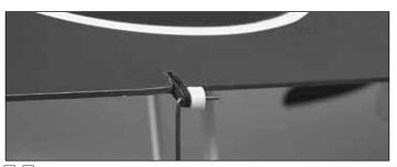
□ □ 13. Install the 100mm pushrod with the L-bend in the control horn of the top wing's aileron. Secure it with a white plastic retainer.
