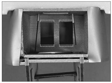
The existing servo cutouts are already wide enough to accommodate the 3114s, but the forward and aft edges must be trimmed approximately 1/16" [1.6mm].
