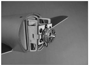
In addition to other servo options, there is another motor option too. The Great Planes Rimfire 300 (28-22-1380) Outrunner Brushless motor (GPMG4505) may be substituted for the Rimfire 250 recommended in the manual. No modifications are required. **NOTE:** Newer versions of this motor may have a bolt-on propeller adapter (instead of the prop-saver O-ring type shown). Still, no modifications will be required.
