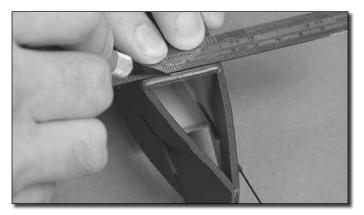
Use a straightedge and a sharp hobby knife to trim end of the fuselage top as necessary to close the gap—typically removing 1/16" to 3/32" [1.6–2.4mm] is suitable. This will bring the stab/fin assembly forward, eliminating the gap.
