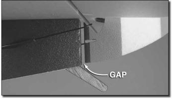
When test-fitting the stab/fin assembly to the fuselage as shown in step 2, check to see if there is a gap between the rudder and the fuselage. If a gap does not exist, proceed with assembly as instructed in the manual. If there is a gap, trim the top of the fuselage as described below.
