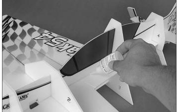
□ 7. Glue the two fuselage pieces together by gently sliding the vertical fuselage and applying foam safe CA glue to the seam between the two fuselage pieces. Be very careful when gluing around the jig pieces. **DO NOT** glue the jig pieces to the fuselage. Apply some foam safe accelerator to the seam, and allow a few moments for the glue to cure.
