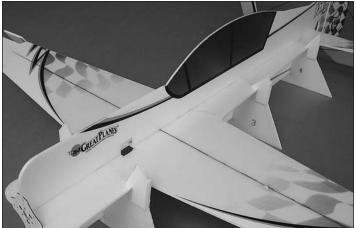
□ 17. Using a hobby knife, remove the top portion of assembly jig pieces 1, 2, and 4 that are close to the fuselage, as shown. There should still be a small amount of the top pieces left, to keep the jig attached to the fuselage.
