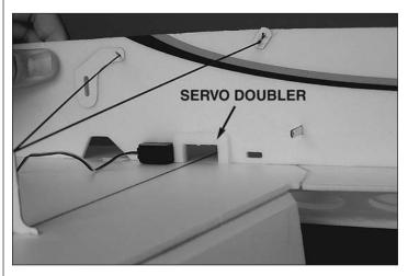
□ 7. Use some foam safe CA to glue the foam servo doubler around the rudder servo slot. **NOTE:** The rudder servo doubler should be glued on the opposite side of the fuselage from the elevator servo.
