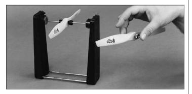
Carefully balance your propeller and spare propellers before you fly. An unbalanced prop can be the single most significant cause of vibration that can damage your model. Not only will motor mounting screws and bolts loosen, possibly with disastrous effect, but vibration may also damage your radio receiver and battery.
