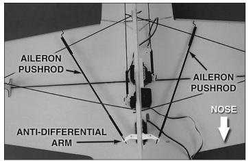
□ 17. Attach one end of each pre-assembled 2mm aileron pushrod to either end of the anti-differential arm, and place the servo arm onto the servo. Look closely at the picture to determine the correct direction of the anti-differential arm.
