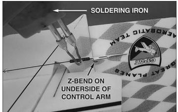
□ 11. Thread a z-bend through the control horn, so that the pushrod mounts to the underside of the control horn. Place one of the included pieces of heat shrink around the z-bend and pushrod. Secure them together by shrinking the tubing using a soldering iron. **BE VERY CAREFUL** when using the soldering iron when very close to the foam. The foam will melt if it is touched with a hot iron.
