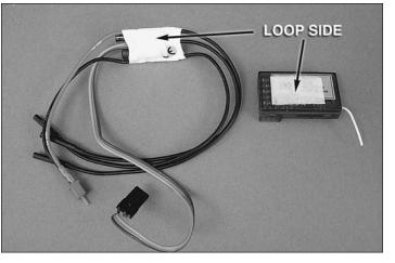
□ 7. Place a small amount of the loop side of the self adhesive hook and loop material to the back of the ESC and receiver that will be used.
