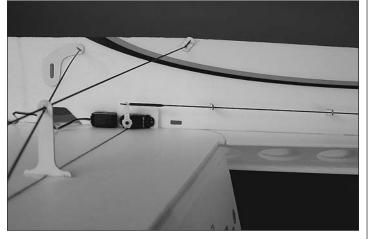
□ 9. Install the rudder servo using the same method that was used to install the elevator servo. **NOTE:** The rudder servo will be installed on the opposite side of the fuselage from the elevator servo.
