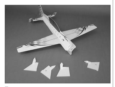
□ 19. At this point double check to make sure the motor mount is in the center of the airframe, and then glue it into position. Carefully remove the bottom pieces of the build jig by cutting or breaking them.
