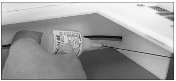
☐ 14. Turn the Yak back, right side up. Locate the two jig pieces marked with a "W" and place them under the wings in the location shown. With all the jig pieces in place, adjust the carbon rods, if necessary, to be certain the wing and horizontal stabilizer are level and straight. Once the wings and stab are aligned, glue the carbon rods to the fuselage, and glue the carbon brace doublers over the slits in the fuselage.
