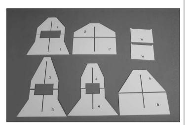
□ 2. Remove the twelve fuselage alignment jig pieces from their surrounding foam. Note: These pieces are labeled 1,2,3,4,6, and W. There are no pieces labeled 5.
