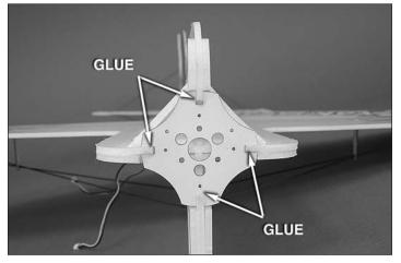
□ 3. This is a good time to reinforce the motor mount by adding some glue around the edges, and to the front of the ABS motor mount.
