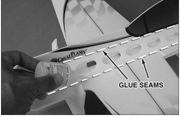
□ 18. Locate the two fuselage stringers. Very gently, so as to not twist the fuselage, glue the stringer at a 45 degree angle to the sides of the fuselage by applying a small amount of glue to the beveled portion of the stringers. Once the glue has had time to cure, reinforce the stringers by applying glue to the seam between the stringers and the fuse halves.
