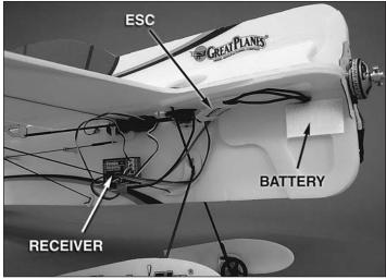
□ 8. Place the hook portion of the self adhesive hook and loop material on the Yak at the positions you wish to mount the receiver, ESC, and battery. One example of where to position the radio gear is shown above. These components may be placed anywhere on the fuselage, as long as they do not interfere with the action of the servos.
