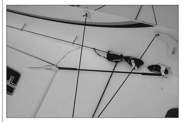
□ 18. Thread a control horn onto each end of the aileron pushrods and glue them into the slits in the ailerons using some CA glue.
