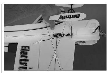
□ 2. With all parts of the model installed (ready to fly) lift the model upside-down at the balance point you desire.
