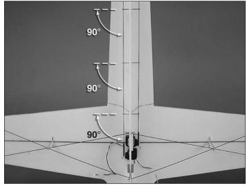
□ 13. Align the pushrod guides so that they are perpendicular to the fuselage and keep the pushrods as straight as possible. Then glue the pushrod guides to the fuselage using some foam safe CA.
