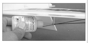
□ 15. Allow a few moments for the glue to cure and then glue the carbon rods in the wing to the carbon brace supports.
