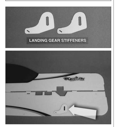
□ 1. Locate the two ABS landing gear stiffeners. Glue a landing gear stiffener to each side of the fuselage in the location shown.
