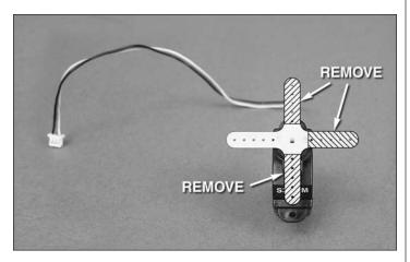
□ 2. Locate your elevator servo. Remove the servo screw from the servo output shaft. Install the larger arm onto the servo. Center the servo using your radio and, using some diagonal pliers, remove the three extra servo arms.
