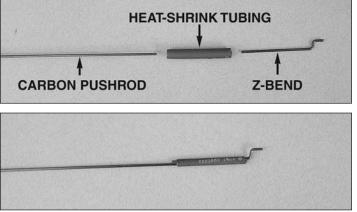
□ 6. Attach one of the included z-bends to the 21-11/16" x 3/64" [550 x 1mm] carbon rudder pushrod, using one of the provided 1" [25.4mm] lengths of heat shrink. Use a soldering iron or heat gun to shrink the pushrod to the z-bend.
