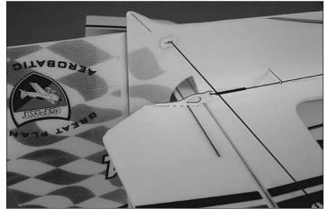
□ 5. Install the elevator control horn by first threading it onto the z-bend at the end of the elevator pushrod. Then place some foam safe CA glue onto the base of the control horn. Insert the pushrod into the slit in the elevator. The slit in the control horn should fit over the carbon elevator joiner. If the control horn will not fit over the carbon joiner, simply remove the excess glue from the slit to achieve a snug fit.
