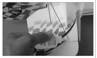
□ 16. Locate the two 7" [178mm] carbon rods. Slide these carbon rods through the slit in the top of the vertical stabilizer
