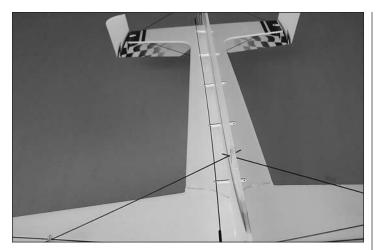
□ 1. Install the pre-assembled elevator pushrod by inserting the pushrod guides through the fuselage as shown. **DO NOT** glue the pushrod guides in place at this time.
