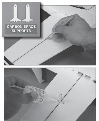
□ 10. Locate the two carbon brace supports. There is a slit located in the center of each wing. With the Yak on its back, glue the carbon brace supports into the slits on the underside of the wing. It is possible that, during manufacturing, some glue has gotten into the slit. If this is the case, **DO NOT FORCE** the carbon brace support into the slit. Simply clear the glue with a hobby knife.
