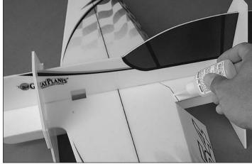
□ 8. Apply a thin bead of foam safe CA glue to the opposite side of the fuselage, and to the seam behind the wing. Activate this CA and allow a few moments for the glue to cure.
