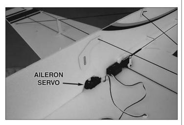
□ 16. Secure the aileron servo to the location shown using some foam-safe CA glue.
