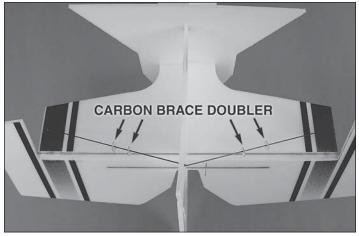
□ 13. Locate the two 6-3/16" [157mm]carbon rods. Thread two carbon brace doublers onto the rods. Place one end of each rod into the slot on the fuselage and the other end of the rod into the slot at the tip of the horizontal stabilizer. Glue the rod to the horizontal stabilizer. Slide one of the carbon brace doublers over the slit and glue it to the stabilizer. **DO NOT glue the carbon to the fuselage at this time.**
