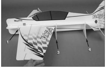
□ 4. On a flat, level work surface, place the base sections of alignment jig pieces number 1,3, and 4 underneath the fuselage in the locations shown.
