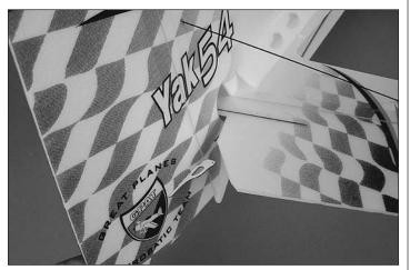
□ 10. Once the rudder servo has been installed and has been secured using some foam safe CA, locate a control horn and glue it into the slit in the rudder, on the same side as the rudder pushrod.
