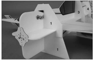
□ 5. Test fit the top sections of the alignment jig pieces onto their corresponding bases. Install the motor mount onto the front of the firewall, but **DO NOT** glue it in place at this time. Connect the top portions of the jig pieces to their bases by applying a small amount of foam safe CA glue to the tabs that overlap. **Be very careful to not glue the jig pieces to the fuselage.**
