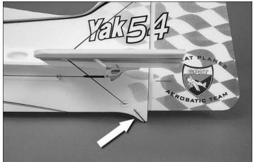
$\Box$  4. Locate the 1/8" x 3/64" x 1" [3 x 1 x 24.5mm] flat, carbon tail skid and glue it into the slit on the underside of the tail, as shown.
