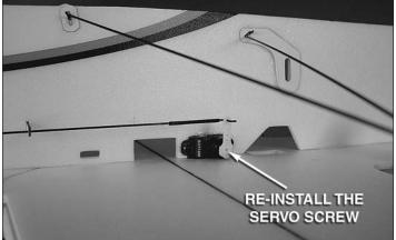
□ 4. Thread the z-bend onto the outer most hole of the servo arm. **Note:** If you are not using a computer radio, and do not wish to set your model up with 3D control throws, you may choose the hole that is most appropriate. When the servo arm is installed correctly the pushrod will exit closest to the fuselage, as shown. Finish the elevator servo installation by centering the servo, placing the servo arm onto the servo, and reinstalling the servo screw.
