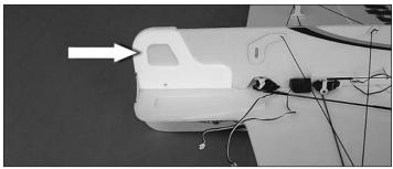
□ 1. Glue the horizontal and vertical fuselage doublers to the underside of the horizontal and vertical fuselage as shown.
