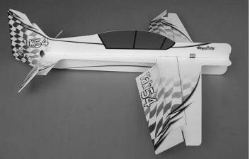
□ 3. Key the rear of the horizontal fuselage into the vertical fuselage. Then key the wing portion into the vertical fuselage.
