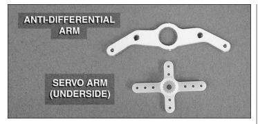
□ 14. Locate the anti-differential arm and your aileron servo arm. Place the anti-differential arm on the underside of the servo arm. If you are using Futaba servo arms, the holes in the servo arm and the holes in the anti-differential arm will align. If you are using another brand servo arm, you will need to use a #60 [1mm] drill bit to drill a pilot hole through the servo arm that will align the servo arm with the antidifferential arm.
