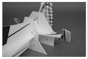
□ 6. Place the base section of jig piece 2 under the wing, and place base jig piece 6 under the horizontal stabilizer. Slide the corresponding top sections over the fuse, as pictured.
