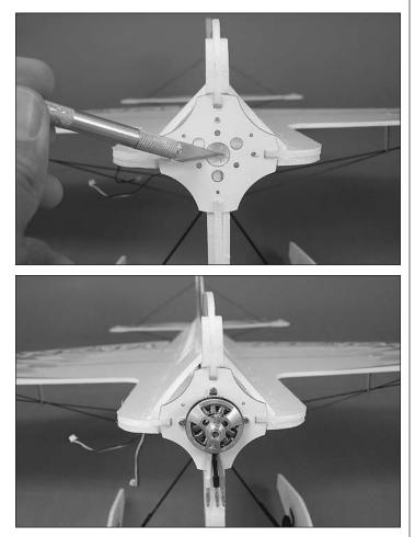
□ 6. Use a hobby knife to remove the foam that sits behind the center hole of the motor mount, so that it does not interfere with the operation of the motor. Install the motor to the motor mount using the screws provided with the motor, or using the  $3/8" \times 5/64"$  [10 x 2mm] self tapping screws provided with the Yak.
