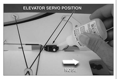
□ 3. Install the elevator servo, without the servo arm, by placing it into the middle servo mount in the fuselage, with the output shaft on the forward side as shown. **NOTE:** Pay carefull attention to the servo position in this picture. Glue the servo in place using some foam-safe CA glue. Be careful to not get any glue inside the servo case. This could ruin your servo.
