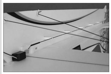
□ 8. Starting from the nose of the airframe, thread the rudder pushrod you have partially assembled through the 5 pushrod supports. The z-bend you have applied should end up at the servo mount.
