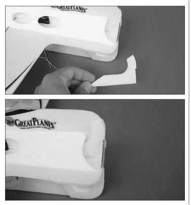
□ 2. Glue the upper horizontal fuselage doubler to either side of the upper horizontal fuselage as shown.
