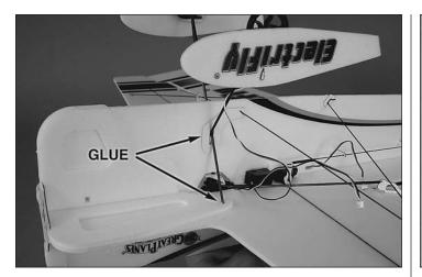
□ 5. Locate the landing gear. Remove the tape holding them in place and thread them through the vertical fuselage and into the horizontal fuselage. Be careful, **DO NOT** press the landing gear all the way through the horizontal fuselage. Glue the landing gear in place using some foam-safe CA glue.
