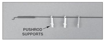
□ □ 1. Using a 1 x 560mm carbon pushrod, one metal **Z-bend**, and one piece of 25mm **heat shrink tubing**, build one end of the **rudder pushrod**. Slide three pushrod supports onto the pushrod. Do not assemble the other end of the pushrod yet.
