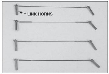
□ 2. Locate eight **aileron link horns**. Fit them to the four aileron links that you made.
