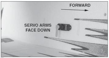
□ 4. Locate the longest servo arms that came with your servos. Since we used Futaba 3114 micro servos, we chose the optional five-hole "X" arms that Futaba supplied with each servo. With the elevator and rudder servos centered, test fit the servo arm to find the long arm that aligns perpendicular with the servo case. Clip off the other unused arms and temporarily fit each arm to each servo with the arm facing down. Do not install the servo arm screw yet.
