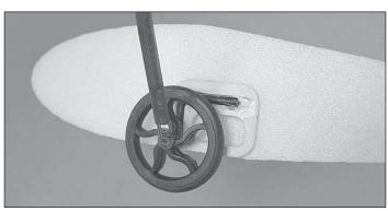
□ 6. Use medium or thick foam-safe CA to attach the wheel pants to the landing gear legs.
