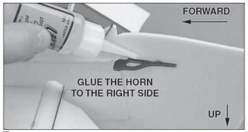
□ 2. Install the other control horn to the right side of the rudder as shown. Apply a bead of thin foam-safe CA around the base of the control horn.
