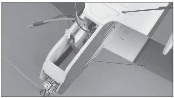
□ 1. Place the battery pack in the plane. **Do not** connect the battery to the ESC.
