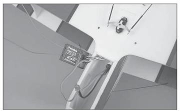
□ 1. Plug your elevator, aileron, and rudder servos into their proper channels. Plug the ESC signal lead into the receiver.
