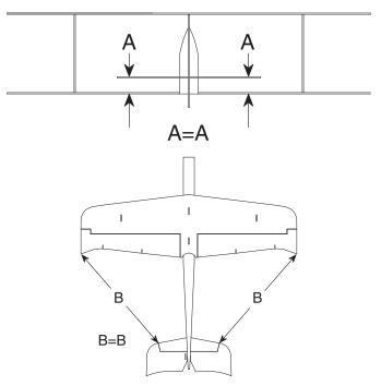
$\Box$  2. Align the stab vertically and horizontally as shown in the sketches above. If the stab doesn't sit parallel with the plane
