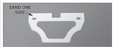
□ 3. Locate the landing gear doubler plate. Roughen one surface of the doubler plate using 150-grit sandpaper.
