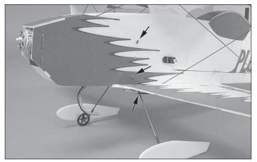
□ 7. Slide each landing gear leg though the holes provided in the wing. They will go through the wing holes first, then the fuselage side, and then cross over to the opposite fuselage side. Rotate the landing gear rod until the wheels point straight ahead. Glue the landing gear in place.
