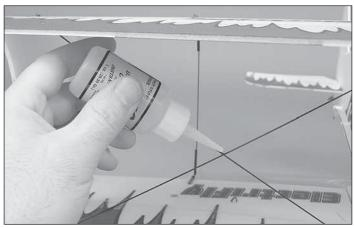
□ 5. With the wings square, place a drop of thick foam-safe CA at the junction of the main wing braces. CA accelerator is helpful here.
