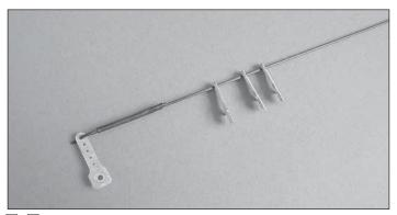
□ □ 2. Remove the servo arm that you temporarily fitted to your rudder servo. Use a #57 [1mm] drill bit to enlarge the outermost servo arm hole. Fit the rudder pushrod to the outermost hole. **Note:** If you don't have a #57 drill bit, carefully use your hobby knife to enlarge the hole.
