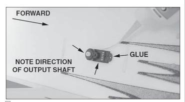
□ 2. Place one drop of foam-safe CA on the bottom of the servo mounting tabs. Install the **rudder servo** on the right side of the fuselage with the **output shaft facing aft**. Guide the servo leads forward through the fuselage and apply a bead of CA along the side of the servo case where it meets the fuselage.
