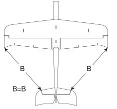
$\Box$  4. Locate the two 1 x 145mm front wing supports. Route each through its respective hole in the LE of the upper wing and into the holes in the forward fuselage. Before you glue them in place, check to see that the upper wing is still aligned with the horizontal stab. When you're satisfied, glue the front supports in place.
