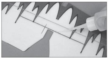
□ 2. Apply a bead of thin foam-safe CA to both sides of the140mm carbon fiber elevator joiner.
