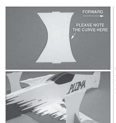
□ 2. Glue the interplane struts to the bottom wings using thin foam-safe CA. Use a 90° builder's square or the template provided in the back of this manual to properly align the interplane struts vertically. **Note:** The front edge of the interplane struts has less curvature than the aft edge.
