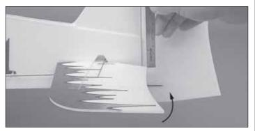
Use a ruler or the templates provided in the back of this manual to accurately measure and set the control throw of each control surface as indicated in the chart that follows. If your radio does not have dual rates, we recommend setting the throws at the **low rate** setting. **Note:** The throws are measured at the **widest part** (inboard or lowest part) of the elevators, ailerons, and rudder.
