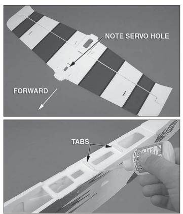
□ 1. Glue the bottom wing to the bottom of the fuselage. Apply a bead of medium or thick foam-safe CA to the wing saddle and the two fuselage former tabs and mount the wing. **Note:** The bottom wing can be identified by the servo hole and the protruding LE stop.
