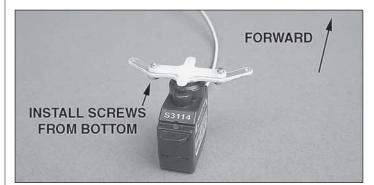
□ 3. Locate the plastic servo arm provided in the kit. Remove the servo arm from your servo. Mount the servo arm to your standard servo arm with the arms swept forward. Use the supplied  $1.5 \times 4$ mm self-tapping screws to install the extended arm to the standard servo arm. Install the screws from the bottom so that the heads of the screws face the body of the servo. **Note:** The output shaft of the servo will face toward the front of the model.
