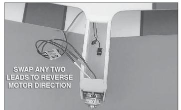
□ 5. Route the motor wires through the firewall and connect them to the ESC. Use your radio to test the direction of motor rotation. If the motor rotates in the wrong direction, swap the position of any two of the three motor leads and re-check the direction of rotation. It's easier to do this now than to find out you have to swap the leads later after everything is mounted and tucked away.
