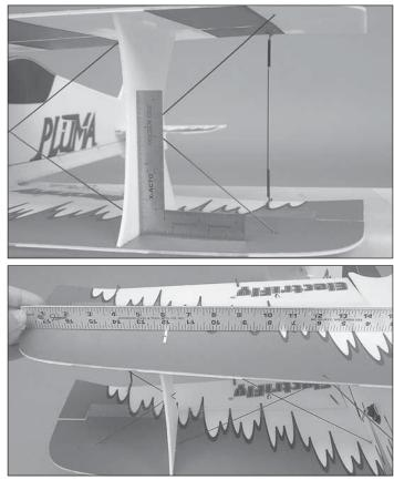
$\Box$  3. Locate the four 1 x 135mm outer wing braces. Two will be used for the left wing and two for the right wing. With the braces fitted and the lower wing still flat on the table, hold a straightedged ruler against the top wing. Align the wings and glue the braces in place.
