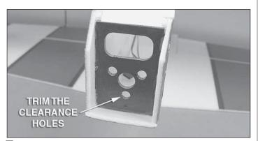
□ 2. Test fit your motor by holding it in place up against the firewall. Make sure that the Y-mount screws fit inside of the clearance holes in the firewall. If it is necessary, carefully enlarge the holes using a Dremel<sup>®</sup> tool or a sharp hobby knife.
