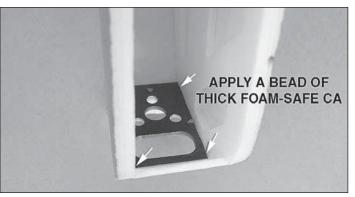
□ 3. If you are installing the more powerful RimFire motor, apply a bead of thick foam-safe CA to the fuselage-to-firewall joint.
