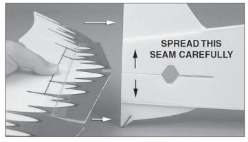
□ 1. Test fit the horizontal stab to the fuselage, installing it from the rear. You'll need to spread the fuselage seam apart a bit to get the stab in, so use care.
