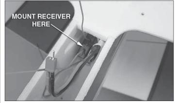
□ 2. Cut a 1" [25mm] long piece of hook and loop material. Stick the hook side (fuzzy side) to the back side of your receiver. Mount the receiver just ahead of the LE of the lower wing.
