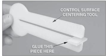
□ 3. Locate the foam parts shown above and build two control surface alignment tools. **Note:** Setting the rectangular pad at 90 degrees is not critical.
