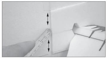
□ 3. Apply the 70mm piece to the center section of the rudder, making sure that you press the tape tightly into the crease. A straightedge is helpful here.
