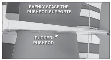
□ □ 5. With the pushrod straight, cut 2mm wide slots in the fuselage for the pushrod supports using a hobby knife. Cut the first slot so that it is 5-1/2" [140mm] from the Z-bend. Space the next slot 5-1/2" [140mm] from that and so on. Ensure that the pushrod is completely straight and use foamsafe CA to glue the supports into the fuselage.
