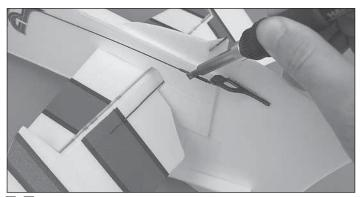
□ □ 4. Fit the servo arm onto the rudder servo and extend the pushrod all the way back to the rudder control horn. Fit a Z-bend to the rudder control horn. Attach the Z-bend to the rudder pushrod using a 25mm piece of heat shrink tubing. Shrink the tubing with a hot soldering iron. **Note: DO NOT attempt to use a torch, cigarette lighter or heat gun near the foam!** It is nearly impossible to use these without melting the foam.
