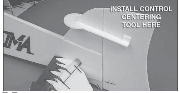
□ □ 3. Install one control alignment tool onto the vertical stabilizer to hold the rudder straight.
