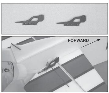
□ 1. Locate two control horns. Turn your model over and install one control horn to the bottom of the left elevator. Apply a bead of thin foam-safe CA around the base of the control horn.
