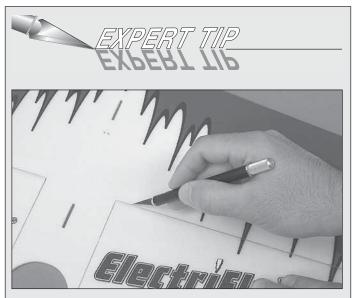
If you ever need to remove a control surface DO NOT attempt to pull the hinge tape off – this damages the skinned layer of the foam – use a hobby knife to cut the hinge tape along the hinge line. Replacement hinge tape is available from your local hobby shop. Order Dubro Electric Flyer Hinge Tape (DUBQ0916).
