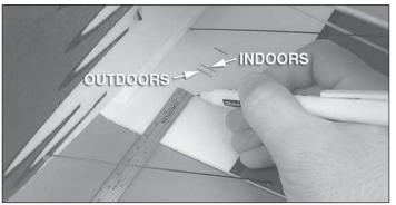
□ 2. Use a felt-tip pen or 1/8" [3mm]-wide tape to accurately mark the C.G. on the bottom of the upper wing on both sides of the center cabane strut. If you are flying indoors primarily, make two marks that are 2-5/8" [67mm] from the LE of the upper wing. If you are flying outdoors, make two C.G. marks that are 2-1/2" [63mm] from the LE of the upper wing. The total C.G. range is from 1-3/4" [44mm] forward to 3-5/16" [85mm] aft. Do not fly your model outside of this range.
