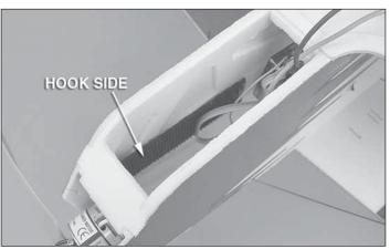
□ 9. With the hook and loop material that you have left over, separate the hook side from the loop side and stick the hook side (bristly side) inside the fuselage. Apply the remaining loop material to your battery packs.
