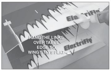
□ □ 4. Set your model down on a flat work surface with the TE of the aileron hanging over the edge. Working with one wing at a time, fit the alignment tools to the top aileron. Test fit two aileron link rods by inserting the link horns into the slots in the upper and lower ailerons. Adjust the position of the link
