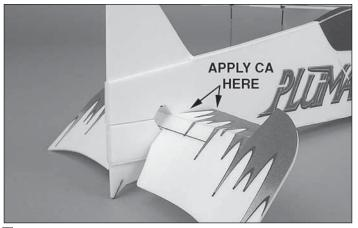
□ 3. When you're satisfied with the fit of the horizontal stab, run a generous bead of thin foam-safe CA down the left and right stab to the fuselage joints. Turn the model over and glue the bottom of each joint as well.
