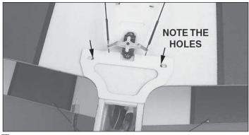
□ 4. Apply several generous beads of medium or thick foamsafe CA to the back side of the landing gear doubler (the side you just sanded). Center the doubler over the holes in the bottom of the lower wing and glue it in place.
