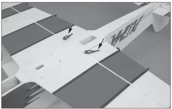
□ 1. Turn the model over. Locate the two remaining control horns. Glue them into the slots provided in the bottom of each lower aileron.
