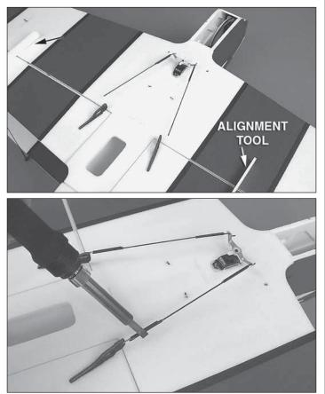
□ 7. Fit the pushrods to the servo arm. Fit the remaining Z-bends to the aileron control horns and slide a piece of heat shrink tubing onto the carbon rods. Shrink the tubing with a hot soldering iron, making sure that your ailerons stay centered in the process.
