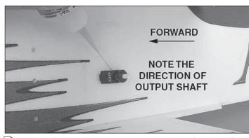
□ 3. Install the **elevator servo** on the left side of the fuselage with the output shaft facing aft. Guide the servo leads forward through the fuselage. **Note:** The aileron servo will be installed later.
