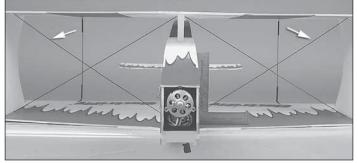
$\Box$  2. Install the 1 x 296mm carbon rods in the wings as shown. Square the fuselage with the wing and glue the wing braces in place.
