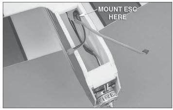
□ 6. Cut a 1" [25mm] strip from the supplied adhesivebacked hook and loop material. Peel the backing paper off and stick the loop side (fuzzy side) onto the back of your ESC. Peel the backing paper off of the hook side and place a few thin beads of thin foam-safe CA on the sticky backing. Mount it in the plane in the location shown.
