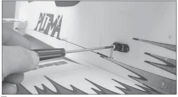
□ 7. Install the servo arm screws.
