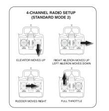
□ 3. Make certain that the control surfaces and the motor respond in the correct direction as shown in the diagram. If any of the controls respond in the wrong direction, use the servo reversing in the transmitter to reverse the servos connected to those controls. Be certain the control surfaces have remained centered. Adjust if necessary.
