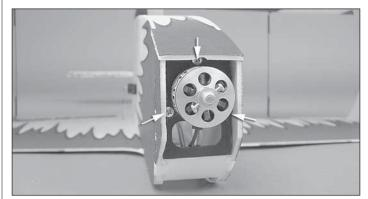
$\Box$  4. Install the motor using three 2.5 x 8mm self-tapping screws. Remove the screws and the motor and harden the screw holes with one drop of thin regular CA. Be careful not to drip any regular CA onto the foam.
