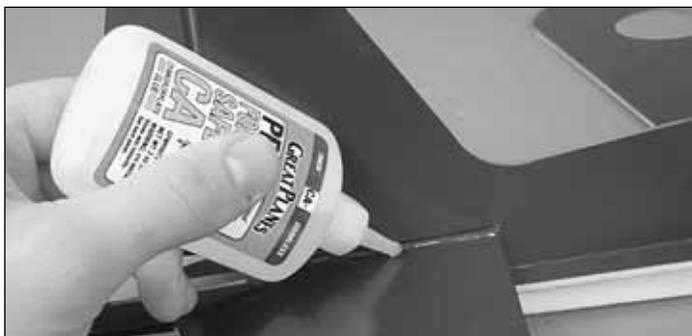
❑ 3. When satisfied, run a bead of thick CA glue along the top and bottom of the stab where it meets the fuse on both sides.
