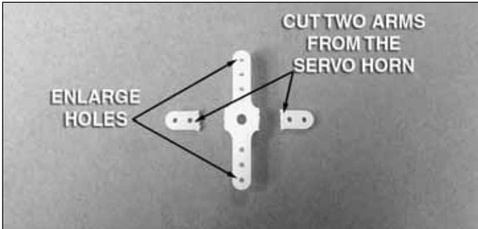
2. Cut two arms from a four-arm servo horn as shown. Enlarge the outer holes in the remaining servo arms with a 3/64" [1.2mm] drill bit.
