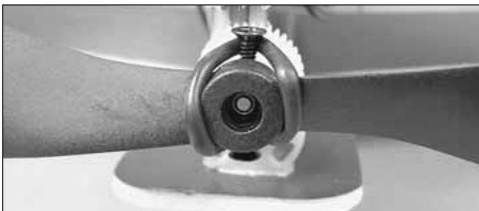
❑ 5. Attach the **prop saver** by tightening the two screws against the flat spots on the prop shaft.
