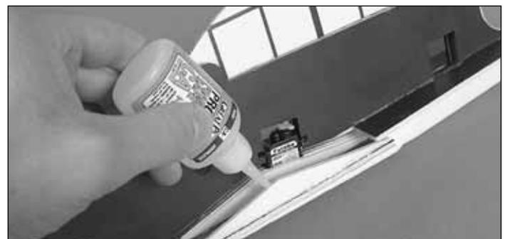
2. Apply a bead of thick CA glue to the tops of the wing supports on the left side of the fuselage. We recommend using CA accelerator to speed assembly time.
