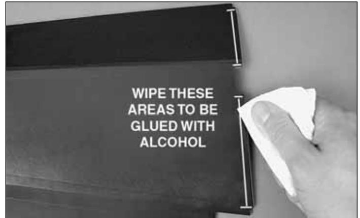
1. For the best adhesion on the painted surfaces, we recommend roughing up the painted surfaces to be glued with fine grit sandpaper such as 320-grit. Wiping the areas to be glued with a paper towel dampened with denatured alcohol will reduce the gloss of the paint and also improve adhesion. If using alcohol, we recommend only making one pass with the towel. Excessive wiping will completely remove the paint from the foam.
