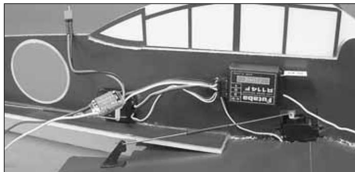
❑ 1. Cut a piece of the included double-sided tape to fit your receiver and stick it to the underside of the receiver case. Connect the ESC, aileron, rudder, and elevator servos to the receiver. Peel the backing from the double-sided tape and secure the receiver to the fuselage in the location shown in the photo. Be sure that you have the servo wires positioned so that they do not interfere with the pushrods.
