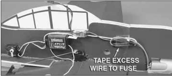
❑ 2. Connect the ESC motor leads to the banana plugs on the motor. Secure the ESC to the fuse with double-sided tape as far forward as the wires will allow. Use a piece of clear tape (not included) to hold the excess motor lead wires against the fuse. Use alcohol to dull the painted surfaces where the tape will be applied.
