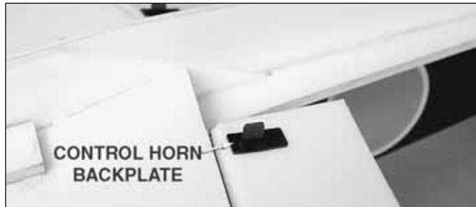
2. Press the control horn backplates onto the tabs to secure the control horns to the ailerons. Glue the backplates to the control horn tabs with a drop of CA.
