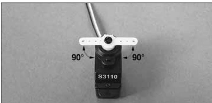
3. Install the servo horn perpendicular to the servo case.
