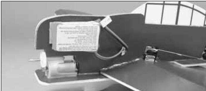
❑ 3. In order to balance the FlatOuts Zero ARF without the addition of weight, the battery pack must be secured above the motor. Use the included **hook and loop material** to do so with the "loop" side on the battery. Applying the "loop" side of the hook and loop material to the front side of the battery will allow the battery discharge leads to reach the ESC battery connectors. The discharge leads will pass through the hole in the fuse to connect to the ESC.
