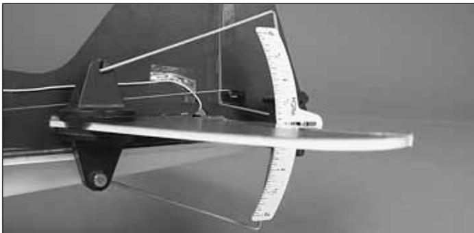
Use a Great Planes AccuThrow (or a ruler) to accurately measure and set the control throw of each control surface as indicated in the chart that follows. If your radio does not have dual rates, we recommend setting the throws at the **low rate** setting.
