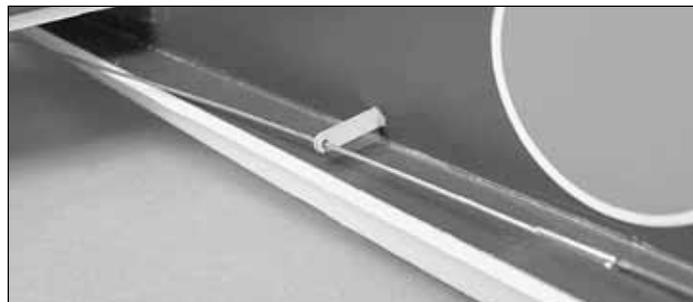
❑ 5. Position the **pushrod supports** in the middle of the pushrods and lightly press them into the fuselage, creating indentations in the foam. Be sure that the pushrod support location will not create any binding in the pushrod. Use a sharp hobby knife to cut a hole in the foam at the indentations you made. Insert the pushrod supports into the holes and glue them in place.
