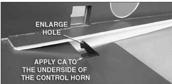
1. Enlarge the outer holes of the two control horns with a 3/64" [1.2mm] drill bit. Apply a couple drops of CA glue to the underside of the control horn backplates. Push the control horn tabs through the slots in the ailerons as shown.
