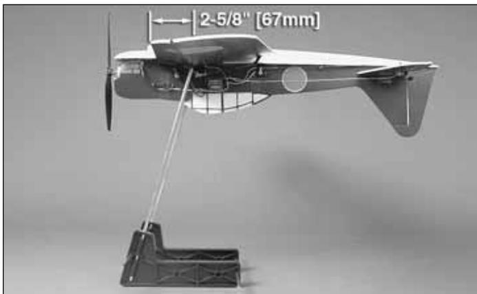
❑ 2. With all parts of the model installed (ready to fly), place the model upside-down on a Great Planes CG Machine, or lift it upside-down at the balance point you marked .
