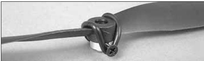
❑ 4. Loop the **prop saver O-ring** around one of the screws and over the **prop hub**. Hook the O-ring onto the other screw to secure the propeller to the prop saver. Long nose pliers may make it easier to stretch the O-ring onto the screws.
