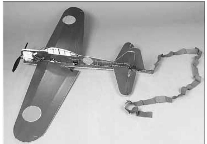
❑ 1. Damage to your plane is inevitable during this kind of combat. However, the simplicity of this model allows it to be repaired quickly at the flying site. Be sure to put some thick foam-safe CA glue and CA activator in your field box, and you will be able to be back in flight in a matter of minutes should repair be necessary.
