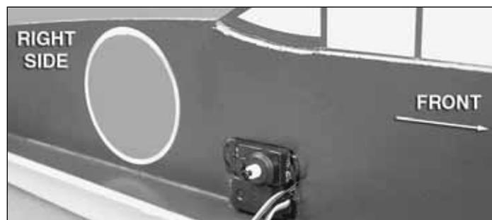
❑ 1. Glue the rudder and elevator servos into the cutout in the fuse with the output splines both facing the front of the plane. The servo in the bottom of the slot is the rudder servo and should be installed with the splines on the **left side** of the fuse. The servo in the top of the slot is the elevator servo and should be installed with the splines on the **right side** of the fuse. Both servo leads should exit out of the right side.
