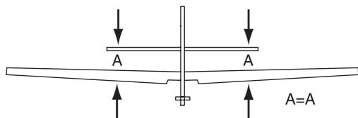
❑ 2. Center the stab left and right in the fuse. Make sure the stab is square to the fuse by measuring the distance between the wing tips and stab tips and setting them equal to each other as shown in the photo. Before gluing, stand back several feet and view the model from behind. The stab should be parallel to the wing. If not, you will need to hold the stab in the correct position as you glue it to the fuse.
