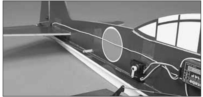
❑ 6. The receiver antenna can be taped to the side of the fuse. However, be sure not to let excess wire hang free of this airplane if you plan to fly combat. Use alcohol to dull the painted surfaces where the tape will be applied. Wrap the excess wire through the elevator joiner tube cutout and tape it to the other side of the fuse. For a cleaner look, you can also cut a slit in the fuse and embed the antenna out of sight.
