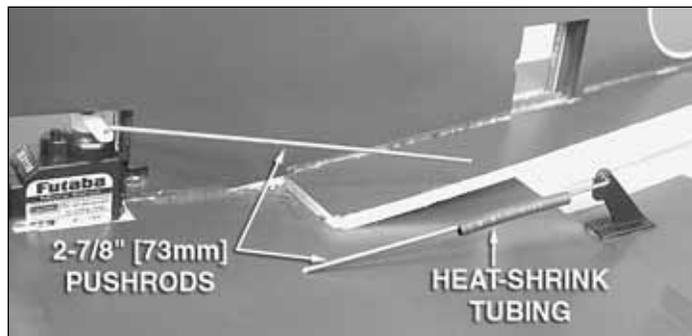
3. Locate the four 2-7/8" [73mm] **pushrods** and hook the Z-bends into the outer holes of the servo horn and the outer holes of the control horns. Slide a piece of 1" [25mm] heat-shrink tubing onto one of the pushrods for each wing panel.
