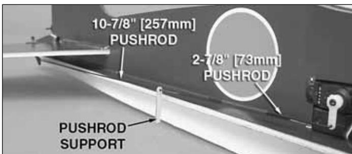
❑ 4. Hook the remaining two 2-7/8" [73mm] pushrods onto the elevator and rudder servo horns. Connect the 10-1/8" [257mm]
