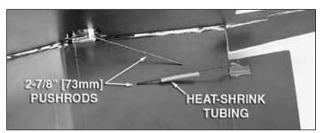
□ 3. Locate the four 2-7/8" [73mm] pushrods and hook the Z-bends into the outer holes of the servo horn and the outer holes in the control horns. Slide a piece of 1" [25mm] heat-shrink tubing onto one of the pushrods for each wing panel.
