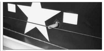
□ 5. Position the pushrod supports in the middle of the pushrods and lightly press them into the fuse creating indentations in the foam. Use a sharp hobby knife to cut a hole in the foam at the indentations you made. Insert the pushrod supports into the holes and glue them in place. Be sure that the position of the pushrod supports do not cause the pushrods to bind.
