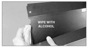
□ □ 1. For the best adhesion on the painted surfaces,we recommend roughing up the painted surfaces to be glued with fine grit sandpaper such as 320-grit. Wiping the areas to be glued with a paper towel dampened with denatured alcohol will reduce the gloss of the paint and also improve adhesion. If using alcohol, we recommend only making one pass with the towel. Excessive wiping will completely remove the paint from the foam.
