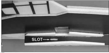
↓ 4. Cut a slot in the fuse on the right side large enough to accommodate the servo connector in the location shown in the picture. The exact placement will depend on the servo manufacturer and where the servo lead wire exits out of the aileron servo being used.
