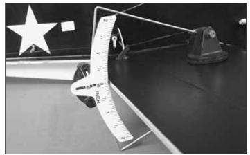
Use a Great Planes AccuThrow (or a ruler) to accurately measure and set the control throw of each control surface as indicated in the chart that follows. If your radio does not have dual rates, we recommend setting the throws at the **low rate** setting.
