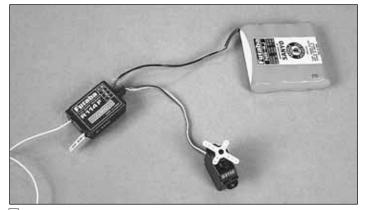
□ 1. Connect the aileron servo to the receiver. Use your ESC or a receiver pack to power the receiver. Turn on your transmitter and center the aileron servo. Do not skip this step, as the aileron servo must be installed into the **fuselage** with the servo horn attached to it.
