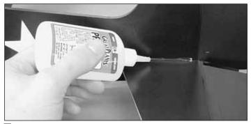
□ 3. When satisfied, run a bead of thick foam safe CA glue along the top and bottom of the stabilizer where it meets the fuse on both sides.
