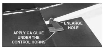
□ 1. Enlarge the outer holes of two **control horns** with a 3/64" [1.2mm] drill bit. Apply a couple drops of CA glue to the underside of the **control horn backplates**. Push the control horn tabs through the slots in the ailerons as shown.
