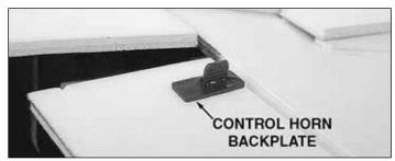
□ 2. Press the control horn backplates onto the tabs to secure the control horns to the ailerons. Glue the backplates to the control horn tabs with a drop of CA.
