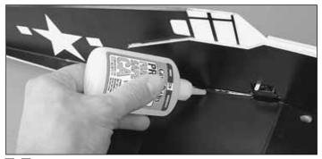
□ □ 4. Apply a bead of CA around the joint between the wing and the fuse on both the top and bottom of the wing.
