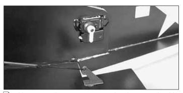
□ 3. Use your radio system to center the elevator and rudder servos. Cut three arms from two four-arm servo horns and install them onto the elevator and rudder servos, both pointing downward. Enlarge the outer holes of the servo horns with a 3/64" [1.2mm] drill bit.
