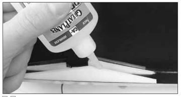
□ □ 2. Apply a bead of thick CA glue to the tops of the **wing supports** on the right side of the fuse. We recommend using CA accelerator to speed the assembly time.
