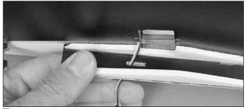
□ 5. Feed the aileron servo lead through the slot you cut into the fuse.
