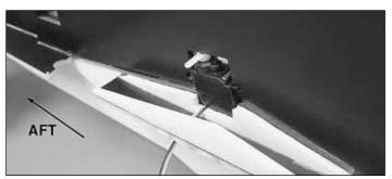
□ 6. Fit the aileron servo into the **aileron servo bay** with the servo spline towards the aft end of the plane.
