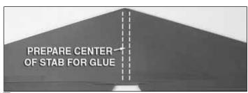
□ 1. Roughen a 1/8" [3mm] strip down the center of the top and bottom of the **horizontal stabilizer**. Use alcohol to dull the paint at the area to be glued. Do the same to the area around the horizontal stabilizer slot in the fuse.
