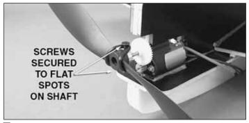
□ 5. Attach the **prop saver** by tightening the two screws against the flat spots on the prop shaft.
