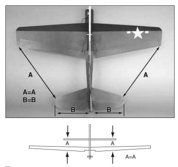
□ 2. Slide stabilizer the into the slot at the TE. Center the stabilizer left and right in the fuse. Make sure that the stabilizer
