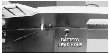
□ 3. A hole is precut on the right wing panel. This can be used for routing the battery leads to the ESC if short wire length makes this necessary. Use the hole as a guide to cut another hole through the horizontal fuselage below it.
