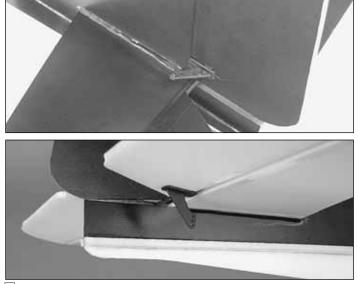
□ 2. Enlarge the outer hole of a control horn using a 3/64" [1.2mm] drill bit. Install this control horn onto the left side of the **rudder**. Enlarge the **inner** hole (closest to the control horn base) of another control horn and install it on the bottom of the right **elevator half**.
