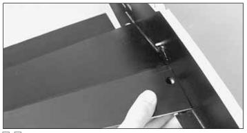
□ □ 3. Insert the **right wing panel** into the slot. The notch at the inside LE of the wing panel will contact the fuse when fully seated. The TE of the wing panel must be aligned with the center of the fuse.
