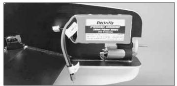
□ 2. In order to balance the FlatOuts Hellcat ARF without the addition of weight, the battery pack must be secured above the motor. Use the included hook and loop material to do so with the "loop" side on the battery. Before applying the "hook" side to the fuse, wipe the area above the motor with alcohol to improve adhesion.
