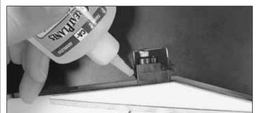
□ 7. With the servo centered in the aileron servo bay, apply a couple of drops of thick foam safe CA glue to each servo case tab, securing the servo to the fuse. Add a couple of drops of CA glue near the base of the servo case as well. It does not require much CA glue to secure the servo to the fuse. Excess glue will simply make it difficult to remove the servo in the future.
