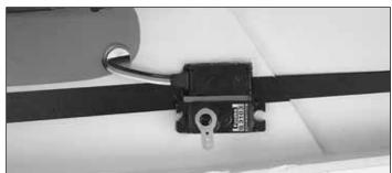
□ 3. Use your radio system to center the elevator and rudder servos. Cut three arms from two four-arm servo horns and install them onto the elevator and rudder servos, both pointing downward. Enlarge the outer holes of the servo horns with a 3/64" [1.2mm] drill bit. Enlarge the **inner hole** of the control horns (closest to the elevator and rudder) with the same size bit.
