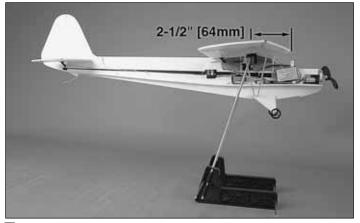
□ 2. With all parts of the model installed (ready to fly), place the model upside-down on a Great Planes CG Machine, or lift it at the balance point you marked.
