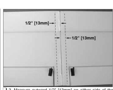
□ 3. Measure outward 1/2" [13mm] on either side of the wing joint. Lightly sand the tape and the foam to scuff it slightly, giving a better gluing surface for joining the wing to the fuselage.
