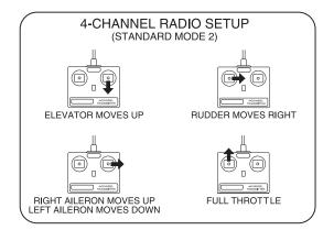
$\Box$  3. Make certain that the control surfaces and the throttle respond in the correct direction as shown in the diagram. If any of the controls respond in the wrong direction, use the servo reversing in the transmitter to reverse the servos connected to those controls. Be certain the control surfaces have remained centered.
