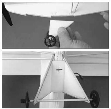
$\Box$  2. Slide the landing gear onto the fuselage. Hold it in place by sliding a T-pin through the bottom of the landing gear and into the fuselage.
