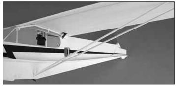
□ □ 3. Install a **strut** into the holes. **DO NOT** glue them in place at this time.
