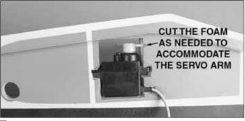
□ 4. Position the servo in the fuselage making sure that the servo arm is positioned as shown. Push the aileron downward into the servo bay until it is firmly seated in position. Center the servo in the fuselage. Cut the foam as needed to accommodate the servo arm.
