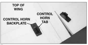
□ 2. Press the control horn backplates onto the tabs to secure the **control horns** to the ailerons. Glue the backplates to the control horn tabs with a drop of CA.
