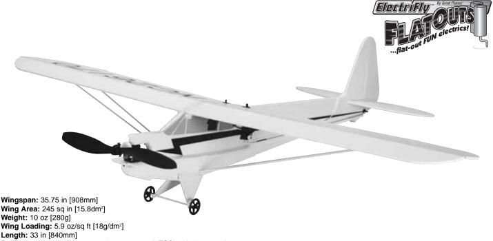
Radio: 4-channel minimum, 3 micro servos, 7A ESC and micro receiver
