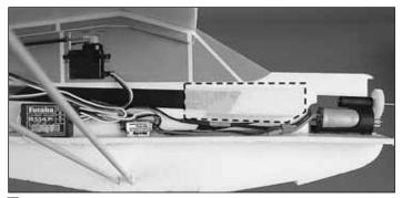
▲ 4. Wipe the area where the hook and loop material will be installed as shown with alcohol as described in step 1. Apply the "hook" side of the hook and loop material to the fuse.
