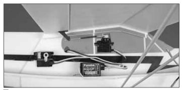
☐ 1. Determine the location of the receiver. Wipe the area with denatured alcohol only once or twice. Excessive wiping will remove the paint. Cut a piece of double-sided tape to fit your receiver and stick it to the underside. Connect the aileron, rudder, and elevator servos to the receiver. Peel the backing from the double-sided tape and secure the receiver to the fuselage in the location shown in the picture. For a tidy installation you may wish to tape the servo leads to the fuselage.
