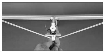
□ 5. Look at the wing to be sure the wing is straight, without any twist. The wing should be flat without any dihedral. When you are satisfied with the wing, glue the struts in place with medium foam safe CA. Be sure to get a good bond between the struts, the wing and the fuselage. The struts are a functional, structural part of the construction of the plane and it is important that they are secured well.
