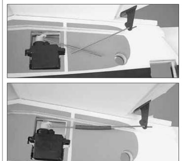
$\Box$  5. Locate the four 2-1/4" [57mm] **pushrods** and hook the Z-bends into the outer holes of the servo horn and the outer
