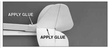
□ 3. Glue the vertical stabilizer/rudder into the slot in the fuselage and the top of the horizontal stabilizer. Hold it in place until the glue hardens.
