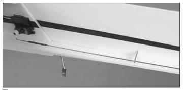
□ 5. Position the pushrod supports in the middle of the pushrods and lightly press them into the fuselage creating indentations in the foam. Use a sharp hobby knife to cut a hole in the foam at the indentations you made. Insert the pushrod supports into the holes and glue them in place.
