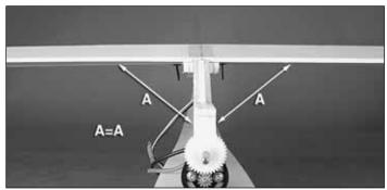
$\Box$  4. Center the wing with the top of the fuselage. Glue the wing to the top of the fuselage with medium or thick foam safe CA glue making sure that the wing is perpendicular to the sides of the fuselage.
