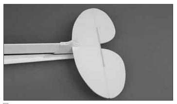
□ 2. Lightly scuff the surface of the stab using sandpaper 5/64" [2mm] on both sides of the line drawn in step 1. Wipe the area with denatured alcohol. Do this on both the top and bottom of the stab. Position the stab onto the back of the fuselage. Using the line drawn in step 1 as a reference, position the stab making sure the stab is parallel to the wing. When you are satisfied with the fit, glue the stab to the fuselage.
