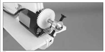
□ 6. Attach the **prop saver** by tightening the two screws against the flat spots on the prop shaft.
