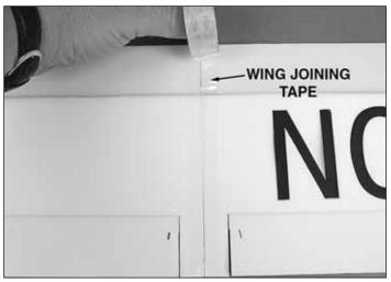
□ 2. Apply the included **wing joining tape** to the bottom and the top of the wing at the wing joint. Press the tape firmly to the surface of the wing.
