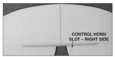
□ 1. Draw a line on the center of the **top and bottom** of the **horizontal stabilizer**. The top of stab has the control horn slot on the right side of the elevator.
