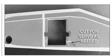
□ 3. Cut a slot in the fuselage on the **right side** large enough to accommodate the servo connector in the locations shown in the picture. Their exact placement will depend on where the servo lead wires exit out of the aileron servo being used.
