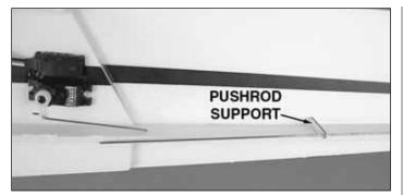
□ 4. Hook the remaining two 2-1/4" [57mm] pushrods into the outer hole of the elevator and rudder control horns. Connect the 16-1/4" [413mm] pushrods onto the inner hole of the elevator and rudder servo horns. Slide a **pushrod support** onto the elevator and rudder pushrods. Join the pushrod wires together with a 1" [25mm] piece of heatshrink tubing while centering the control surfaces. Apply a drop of CA to the ends of the heat-shrink tubing after shrinking the tubing with a soldering iron.
