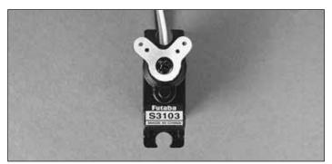
□ 2. Connect the aileron servo to the receiver. Use your ESC or a receiver pack to power the receiver. Turn on your transmitter and center the aileron servo. Do not skip this step as the aileron servo must be installed into the **fuselage** with the servo horn installed as shown.
