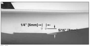
□ □ 1. From the bottom of the fuselage measure up 5/16" [8mm] and make a mark. Measure forward from the mark 1/4" [6mm] and make another mark. On each of these marks drill a 1/8" [3mm] hole at a 30° upward angle to the fuselage. Do not use a electric drill to make the holes. Just twist the drill bit using your fingers. You do not want to drill all the way through the fuselage. Just drill in far enough so the drill bit just makes contact with the skin on the opposite side of the fuselage.
