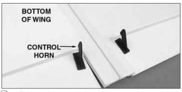
□ 1. Enlarge the outer holes of the control horns with a 3/64" [1.2mm] drill bit. Apply a couple drops of CA glue to the underside of the **control horn backplates**. Push the control horn tabs through the slots in the ailerons as shown.
