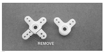
□ 1. Remove two of the arms so that it matches the horn shown on the right. Each of the arms should have two holes. Enlarge the outer holes in the remaining servo arms with a 3/64" [1.2mm] drill bit. **Note:** The purpose for this configuration is to provide mechanical differential to the **ailerons**. In our test flying we determined the plane performs best with some differential in the ailerons.
