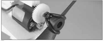
□ 7. Loop the prop saver O-ring around one of the screws and over the prop hub. Hook the O-ring onto the other screw to secure the propeller to the prop saver. Long nose pliers may make it easier to stretch the O-ring onto the screws.
