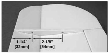
$\Box$  2. On the inside of the **wing rib** measuring from the front of the rib, make a mark 1-1/4" [32mm] back from the
