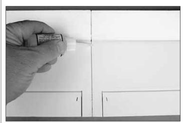
□ 1. Locate the **left** and **right wing panels**. Place them upside-down on the bench. Apply a bead of thick foam safe CA
