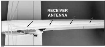
□ 2. Tape the receiver antenna to the bottom of the fuselage longeron as shown. Be sure that none of the antenna is exposed on the underside of the airplane, as it could become damaged on landing.
