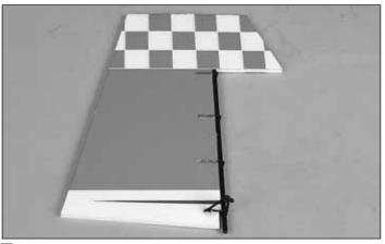
9. Using the technique described in the previous *Expert Tip*, glue three C2 clip hinges and a C1 clip hinge control horn to the **rudder**, using the 3 x 118mm [1/8" x 4-5/8"] **rudder post tube** as a guide.
