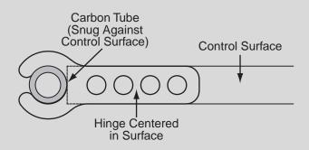
**C.** One at a time, coat the sides of each hinge and glue them into the slots.
