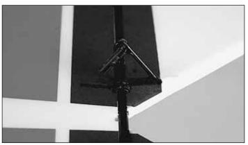
10. Coat the gluing area on the control horn with glue and rotate it down into the precut slot.
