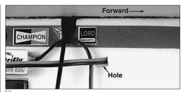
■ 8. Connect your speed control to the motor and receiver. Mount the speed control to the bottom of the left horizontal fuselage with double-sided foam tape. Cut a small hole for the ESC's battery wire to cross to the right side of the fuselage.
