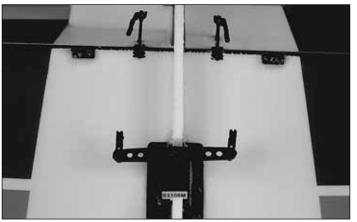
☐ 6. Use your radio to center the aileron servo. Mount the double-sided servo arm to the aileron servo.
