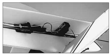
12. Connect all three servos to the receiver. Mount the receiver to the bottom of the right horizontal fuselage with double-sided foam tape. Make sure the receiver is far enough forward so that it does not interfere with aileron motion.
