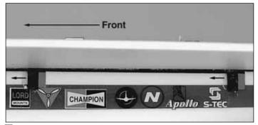
4. Installing them from the **left** side, glue two more supports into the slots in the fuselage. Note that these first two supports should be positioned **forward** in the slots, and that the holes in the supports should be angled downward and outward (again, to accommodate the angles of the landing gear and the struts).
