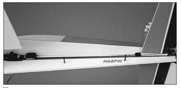
☐ 10. Using the pushrod as a guide, drill two evenly spaced, 2.5mm [3/32"] holes in the fuselage. Glue the bases of the pushrod guides into these holes.
