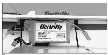
1. Attach the "loop" side of the hook-and-loop material to the battery. Mount the battery to the fuselage.
