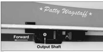
1. Glue the elevator servo into the **front** servo mount in the left side of the fuselage. The output shaft should be forward.
