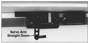
■ 8. Select two single-sided servo arms to fit the elevator and rudder servos you are using. Insert an A1 Z-bend clevis into the outer hole of each arm. Use your radio to center the servos, and mount the servo arms so that they point straight down with the servos centered.
