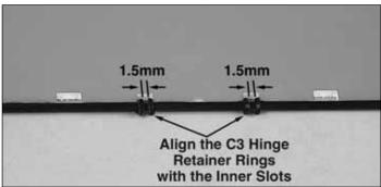
□ 2. Slide four C3 hinge retainer rings onto the 3 x 900mm [1/8" x 35-7/16"] wing trailing edge tube. Position the rings so that they align with the inner slots in the TE of the foam wing. Secure the retainers with a drop of glue each on the outside of the gap. Glue the trailing edge tube to the TE of the wing.
