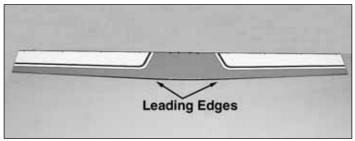
☐ 3. Glue one 3 x 900mm [1/8" x 35-7/16"] wing leading edge tube to the LE of the wing.
