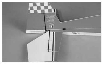
☐ 12. Snap the rudder onto the rudder post.
