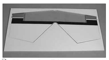
■ 5. Following the *Expert Tip* below, permanently join the elevator halves by gluing in the elevator joiner tube.
