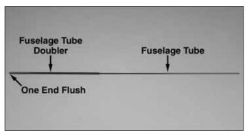
$\square$  2. Glue the 5.5 x 250mm [7/32" x 9-7/8"] **fuselage tube doubler** over the 3 x 649mm [1/8" x 25-1/2"] **fuselage tube**. One end should be flush. From now on, this assembly will be referred to as the fuselage tube.
