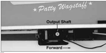
2. Glue the rudder servo into the **rear** servo mount in the right side of the fuselage. The output shaft should be forward.
