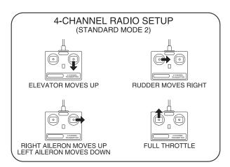
5. Make certain that the control surfaces and the motor respond in the correct direction as shown in the diagram. To operate the motor, you may have to "arm" your ESC. Follow the instructions that came with your ESC to do this. If any of the controls respond in the wrong direction, use the servo reversing in the transmitter to reverse the servos connected to those controls. Be certain the control surfaces have remained centered. Adjust if necessary.
