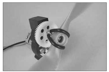
7. Secure the prop to the prop saver with one of the included O-rings.
