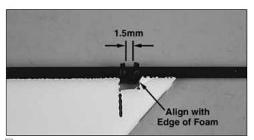
4. Without removing the elevator halves from the foam sheet, slide two **C3 hinge retainer rings** onto the **elevator joiner tube**. Align the rings with the cutout in the left elevator half. There should be a 1.5mm [1/16"] gap between the two rings. Secure each ring with a drop of glue on the outside of the gap. Avoid getting glue between the rings.
