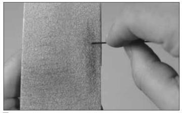
□ 5. Using a 220-grit sanding block, sharpen the ends of all the 1mm [0.40"] carbon **pushrods**. This will make it much easier to install them through the Z-bend clevises.
