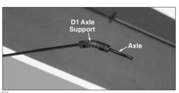
■ 1. Install a 2 x 17mm [5/64" x 5/8"] **axle** and **D1 axle support** onto each landing gear leg. Position the axles so that they are perpendicular to the centerline. Secure the axles and supports with a drop of glue through the holes in both sides of the axle supports.
