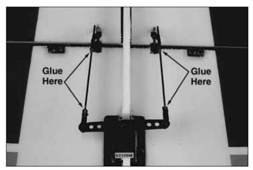
7. Slide a 1 x 55mm [.040" x 2-3/16"] aileron pushrod through the clevises in the aileron horns and servo arms. Adjust the clevises until the ailerons are centered with the servo centered. When you have the alignment correct, secure the pushrod with a drop of glue where the pushrod enters the clevis. Keep glue away from the end of the clevis where it pivots in the arm or horn.
