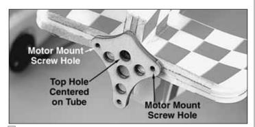
4. If installing an ElectriFly RimFire motor, glue the included 3mm [1/8"] plywood firewall to the nose so that the two pilot holes on the sides of the firewall are centered on the horizontal fuselage, and the top hole is centered on the fuselage tube.
