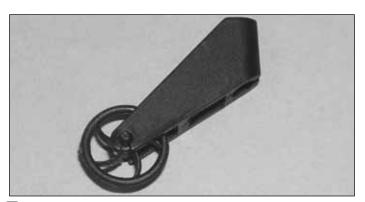
4. Snap the D5 tailwheel into the D4 tailwheel bracket.
