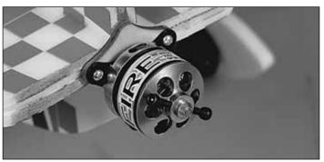
5. Mount the motor to the firewall using the hardware supplied with your motor.
