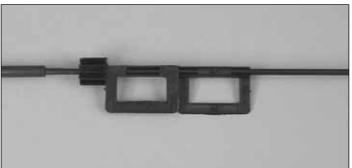
■ 3. Slide an **E2 fuselage joiner**, two **F3 fuselage servo mounts**, and another fuselage joiner onto the fuselage tube. With the tube doubler forward, and the servo mounts hanging down, the front servo mount should have its flat face on the left, and the rear servo mount should have its flat face on the right.
