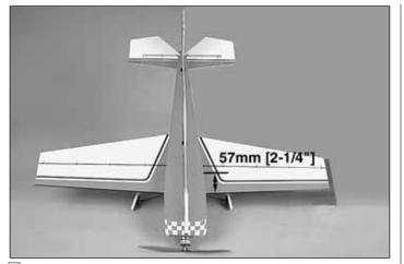
☐ 1. Use a felt-tip pen or 3mm [1/8"]-wide tape to accurately mark the C.G. on the top of the wing on both sides of the fuselage. The C.G. is located 57mm [2-1/4"] back from the leading edge of the wing at the fuselage.
