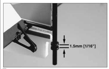
☐ 11. Slide two C3 hinge retainer rings onto the bottom of the rudder post. Align the top ring with the point where the foam meets the rudder post tube. Position the bottom ring 1.5mm [1/16"] below the top one. Secure each ring with a drop of glue on the outside of the gap. Avoid getting glue between the rings.
