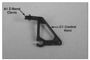
□ 8. Insert an A1 Z-bend clevis into a C1 clip-hinge control horn.
