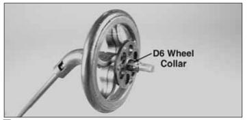
■ 2. Slide the **wheels** onto the axles, and secure them with a **D6 wheel collar**. The flat side of the wheel collar should be toward the wheel. Secure the wheel collar with a drop of glue in the *teeth* opposite the wheels.
