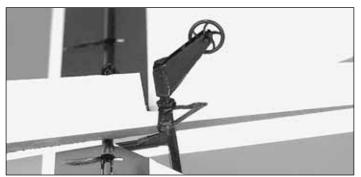
□ 5. Slide the tailwheel bracket over the rudder and rudder post. Glue the bracket to the rudder and *not to the rudder post*. The bracket needs to pivot on the rudder post.
