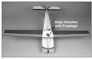
☐ 1. Glue the aileron servo into the F2 wing servo mount, and glue the servo mount into the precut opening in the wing. Slide the wing into the slot in the bottom of the vertical fuselage. Center the wing using the notches in the LE and TE as a guide. Once centered, glue the wing in place with a bead of glue on both sides of the joint.
