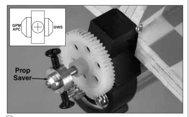
☐ 5. If using the included propeller, install the **prop saver** onto the gearbox shaft with the large-diameter cone forward. If using a GWS prop, install the prop saver with the small-diameter cone forward. Tighten the screws, making sure they engage the flat spots on the shaft.
