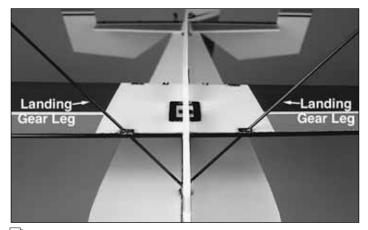
■ 6. Slide the 2 x 170mm [5/64" x 6-11/16"] landing gear legs through the landing gear supports in the front of the wing and fuselage. Ensure that the wing is parallel with the stab and horizontal fuselage and perpendicular to the vertical fuselage. Once you are satisfied with alignment, secure the landing gear legs with a drop of glue on both sides of each joint.
