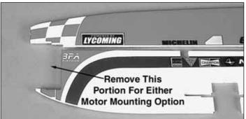
☐ 1. Cut the upper and lower vertical fuselage parts and the right and left horizontal fuselage parts free from their foam sheets. If using the gearbox included with this kit, or any other type of "stick-mount" gearbox, cut out all four sections from the fuselage parts. If using a firewall-mounted, brushless outrunner motor, cut out only the section from the lower vertical fuselage.
