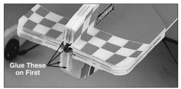
2. Glue the doublers for the vertical fuselage into position first, then glue the doublers for the horizontal fuselage into position.
