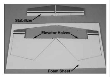
1. Cut the **stabilizer** free from the foam sheet with a *sharp* #11 hobby knife. **DO NOT** cut the **elevator halves** free at this time.
