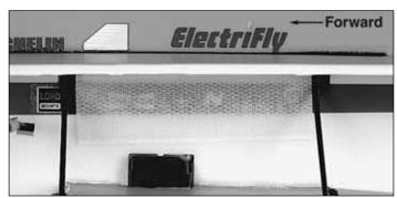
9. Install the "hook" side of the included hook-and-loop material to the left side of the fuselage where shown. This is where you will mount your battery.
