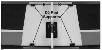
☐ 3. Installing them up through the bottom, glue four supports into the slots in both sides of the wing. Two of the supports are at the leading edge (for the landing gear) and two are at the trailing edge (for the wing struts). **IMPORTANT:** The holes in the supports must be angled **downward** and **outward** (matching the angle of the landing gear and the wing struts).
