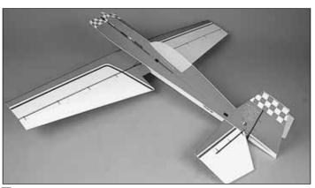
8. Snap the ailerons onto the wing trailing edge tube.
