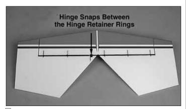
☐ 7. Join the elevators to the stab by snapping the clip hinges to the joiner tube.
