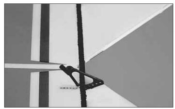
9. Clip the control horn onto the joiner tube aligned with the precut slot.
