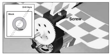
4. Drill a 1.5mm [1/16"] pilot hole at an angle from the top of the gearbox through the balsa block and carbon tubes. Make sure the motor mount block does not rotate while drilling. Secure the gearbox and block with a 2mm wood screw.
