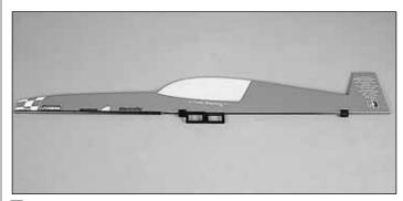
4. Position the servo mounts and fuse joiners so that they align with the precut slots in the upper vertical fuselage.
