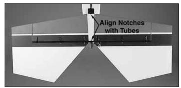
7. Glue the stabilizer into position on the bottom of the horizontal fuselage halves. Use the notches in the LE and TE of the stab to align it with the fuselage tube.
