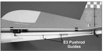
9. Slide two **E3 pushrod guides** onto the 1 x 355mm [.040" x 14"] **elevator pushrod** and slide the pushrod through the clevises on the elevator servo arm and control horn. Adjust the clevises until the elevator is centered with the servo centered. Secure the clevises with a drop of glue on each clevis where the pushrod enters it.
