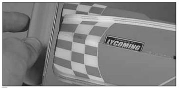
3. Use a 220-grit sanding block to sand the front of the fuselage smooth. Be careful not to change the built-in thrust angles.
