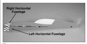
☐ 6. Glue the left and right horizontal fuselage halves to the fuselage tube. Make sure they are perpendicular to the vertical fuselage.
