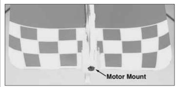
☐ 2. Without using any glue, slide the motor mount block over the fuselage tube. Be certain the block is in the correct position so there will be up and right thrust. Do not glue the motor mount block onto the fuselage tube.
