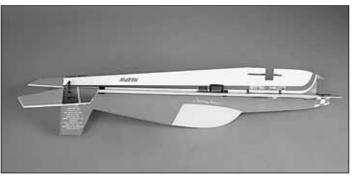
■ 8. Glue the **bottom vertical fuselage half** to the fuselage tube. Make sure to keep it parallel with the top half and perpendicular to the horizontal fuselage. Glue the backs of the servo mounts to the bottom vertical fuselage half.
