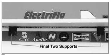
☐ 5. Glue the remaining two supports into the right side of the fuselage. Be certain that the holes are angled correctly.
