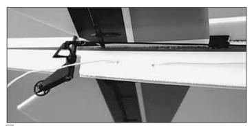
☐ 13. Drill two 1.5mm [1/16"] holes in the tail of the airplane. "Stitch" the receiver antenna through these holes.
