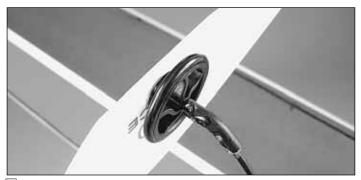
■ 3. Make two wheel pants by gluing the **inner** and **outer** wheel pant parts together. Be sure to make a **right** and a **left**. Glue the inside of both wheel pants to the wheel collars.
