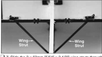
7. Slide the 2 x 63mm [5/64" x 2-1/2"] wing struts through both sets of supports on the back of the wing and fuselage. Make sure that the TE of the wing is aligned with the LE, and secure the struts with a drop of glue on both sides of each joint.
