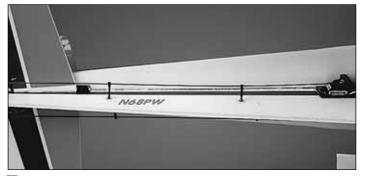
11. Install the 1 x 323mm [.040" x 12-11/16"] **rudder pushrod** the same way.
