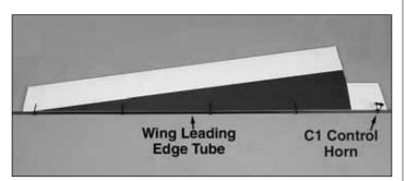
□ 1. Insert A1 Z-bend clevises into opposite sides of two C1 clip-hinge control horns. Following the *Expert Tip* previously described, glue four hinges and a control horn into each of the ailerons, using a 3 x 900mm [1/8" x 18"] wing leading edge tube as a guide. The control horns should protrude from the bottom of the ailerons (red and white side), and the A1 Z-bend clevises should be on the outboard side of the horns. Remove the tube once the glue has set.
