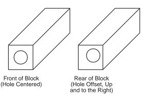
☐ 1. The 10 x 10 x 22mm hardwood motor mount block must be mounted in the correct orientation to insure the proper right thrust. Identify the top, aft end of the block as shown in the sketch so you will know how it is to be installed.
