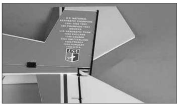
10. Remove the rudder post tube from the rudder. Glue the rudder post tube to the TE of the vertical fin and vertical fuselage halves.
