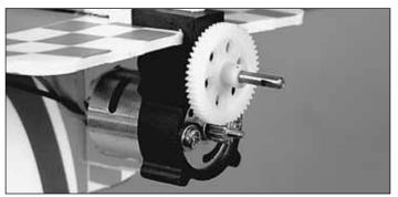
☐ 3. Slide the **motor/gearbox assembly** over the motor mount block.
