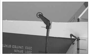
□ 5. Slide the tailwheel bracket over the rudder and rudder post. Glue the bracket to the rudder **only**. **Do not** glue the bracket to the rudder post.
