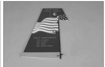
□ 10. Using the 3 x 154mm [1/8" x 6"] **rudder post tube** as a guide, glue three clip hinges and a clip hinge control horn to the **rudder**.
