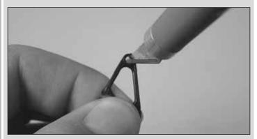
**A.** Using a sharp #11 hobby knife, remove any flashing from the inside of the hole you are installing the Z-bend clevis into. Do this by rotating the blade in the hole while applying gentle pressure. Be careful not to remove too much material–your goal here is to remove small ridges of flashing, not to make the hole larger.
