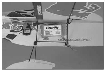
□ 1. Attach the "loop" side of the hook-and-loop material to the battery. Mount the battery to the fuselage.
