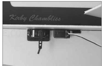
■ 8. Select two single-sided servo arms to fit the elevator and rudder servos you are using. Insert a Z-bend clevis into the outer hole of each arm. Mount the servo arms so that they point straight down with the servos centered. Cut a small hole in the fuselage to allow the elevator servo wire to pass through to the right side of the fuselage.
