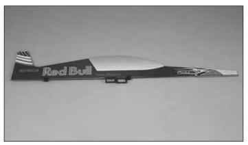
□ 4. Position the servo mounts and fuselage joiners so that they align with the precut slots in the upper vertical fuselage half.
