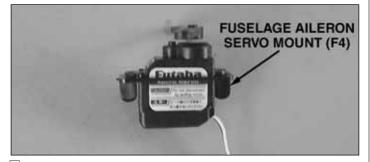
↓ 4. Install the servo arm on the aileron servo in the position shown. Both arms should be offset forward by the same angle. Glue the aileron servo into a **fuselage aileron** servo mount (F4).
