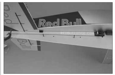
$\Box$  13. Install the 1 x 315mm [3/64" x 12-3/8"] rudder pushrod the same way.
