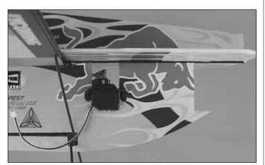
$\Box$  5. With the output shaft aft, glue the aileron servo into the cutout under the wing.
