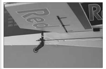
□ 15. Drill two 1.5mm [1/16"] holes through the fuselage where shown. "Stitch" the receiver antenna through these holes.
