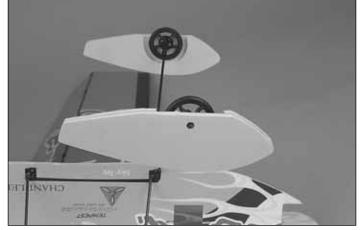
□ 3. Make two wheel pants by gluing the **inner** and **outer** wheel pant parts together. Be sure to make a **right** and a left. Glue the inside of both wheel pants to the wheel collars.
