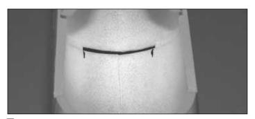
☐ 3. Remove the landing gear former. Cut a slot, centered in the groove, from one mark to the other. Keep the piece of foam that was removed from the slot you cut, so it can be glued back into position after the former and the landing gear have been installed.
