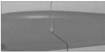
□ 9. After the epoxy from the previous step has hardened, glue the main landing gear wire and the plywood **retainer** (5) into position. Before the epoxy hardens, fit the section of foam that you removed back into the slot in the fuse.
