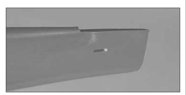
1. Using the indentations in the aft end of the fuselage as a guide, cut the slots for the elevator and rudder pushrods.
