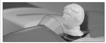
☐ 6. Test fit the clear plastic windscreen to the front of the fuselage. Use a hobby knife with a #11 blade to make three
