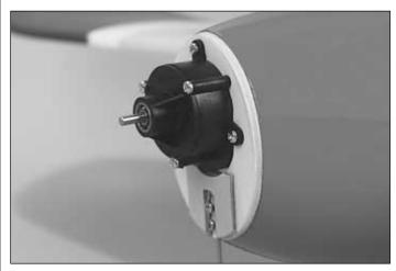
☐ 12. Remove the propeller from the gearbox. Position the motor and gearbox on the firewall. Using the holes in the mounting tabs on the gearbox as a guide, drill three 1/16" holes through the firewall for the mounting screws. Mount the gearbox to the firewall with three wood screws.
