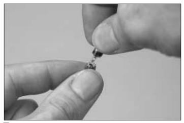
5. Remove the pinion gear from the motor. Add a small drop of gear cement to the hole in the end of the gear that goes on the shaft. Install the gear until the end is even with the end of the shaft. Allow the cement to harden for a few minutes.
