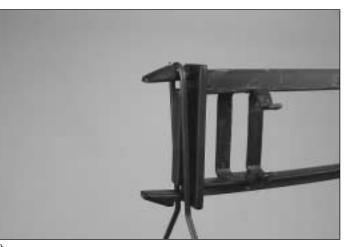
4. Fit the main landing gear wire onto the **front** of the battery holder. Then, mount the battery holder to the battery holder mounts previously installed on the fuselage.
