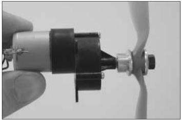
7. Reinstall the motor into the gearbox up to the line. Fit the prop adapter to the gearbox. Mount the prop to the adapter using the appropriate spacer ring and the prop washer and prop nut. Tighten the prop nut with an 8mm wrench. If necessary, protecting the drive washer with a cloth, use pliers to hold the drive washer while tightening the nut.
