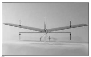
□ 5. View the model from the rear. Using the stab as an alignment cue, make sure both wings are at the same angle when compared to the stab. If necessary, adjust the wing mounts to get both wings the same.
