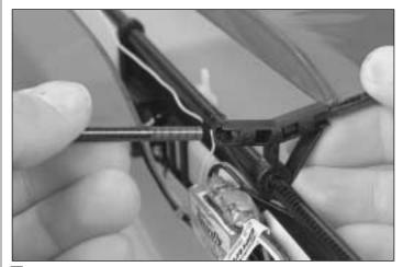
2. Mount the wings to the fuselage boom by fitting them into the wing mounts.
