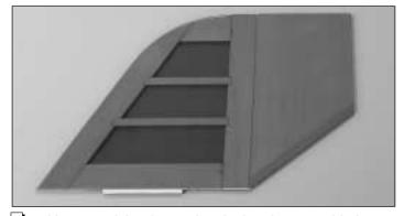
□ 1. Use a straightedge and a single-edge razor blade or a #11 hobby blade to cut the covering from the **left** side of the **fin** across the top of the tab as shown in the photo. Use a light touch to cut **only into the covering** and not into the wood. Also be sure to use a new blade–if the blade is dull it will cause you to apply more pressure, thus cutting into the wood.
