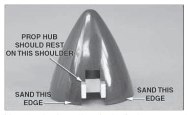
If the spinner interferes with the fuselage/cowl, you may need to sand the rear edge of the spinner to make it fit. It may be necessary to remove some material from the rear edge of the spinner before it fits without contacting the fuselage. The spinner is correctly mounted when the "shoulder" of each cutout rests on the prop hub AND the rear edge does not contact the fuselage at any point when the propeller is rotated.
