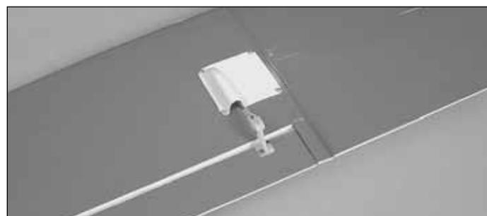
5. Align the holes in the control horn with the hinge line, keeping the pushrod aligned with the servo arm. Mount the
