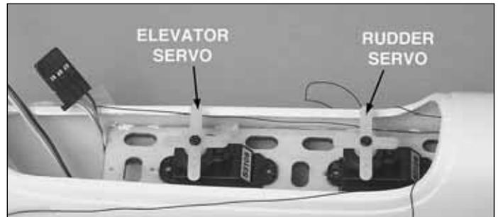
❑ 5. Mount the servos to the servo tray. **Optional:** To keep the weight low, use a drop of medium CA through each servo screw hole instead of the servo screws.
