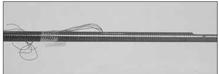
❑ 2. Move the tape holding the pushrod strings forward of the pushrod exits. This will minimize the chance of gluing the pushrod strings to the fuse while gluing the tail in place.
