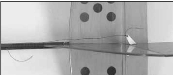
❑ 2. Tie the pushrod string from the pushrod exit on the right side of the fuselage to the right side of the rudder control horn as shown in the sketch.
