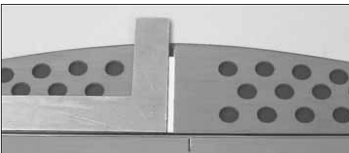
❑ 2. Use a small square and a single-edge razor blade or a #11 hobby blade to cut a strip of covering from the bottom and top of the stab aligned with the fin slot and perpendicular to the hinge line. Use a light touch to cut **only into the covering** and not into the wood. Also be sure to use a new blade—if the blade is dull it will cause you to apply more pressure, thus cutting into the wood.
