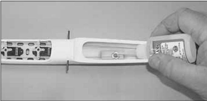
1. Secure the **tow hook** with a couple of drops of thin CA applied to the threads from the inside of the plane. **Note:** Do not glue the pushrod strings together.
