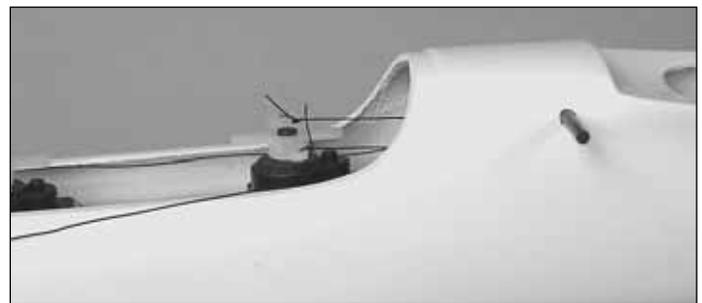
❑ 7. Tie the rudder pushrod strings to rudder servo arm. Tie a single knot first.
