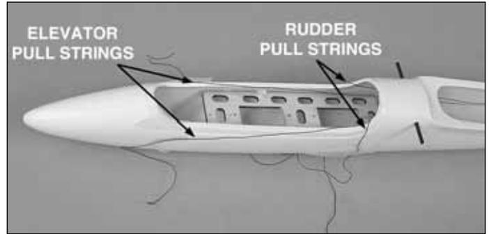
❑ 4. Pull on each string to see what control surface it moves. Tape the four strings to the fuse side as shown. **Note:** Take your time to make sure the strings don't interfere with each other.
