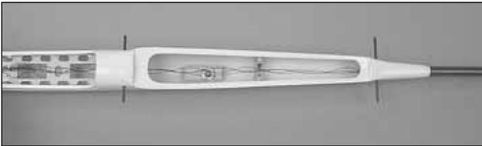
❑ 6. Glue the carbon fiber **wing dowels** into the fuse with a small amount of thin CA.
