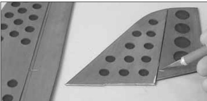
❑ 1. Remove the covering from the control horn slots in the rudder and elevator.
