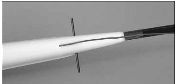
6. Drill a 1/16" [1.5mm] hole in the bottom of the fuse in the rear of the wing opening. Route the antenna through the forward wing former and out the hole in the bottom of the fuse. Tape the antenna to the bottom of the fuse.
