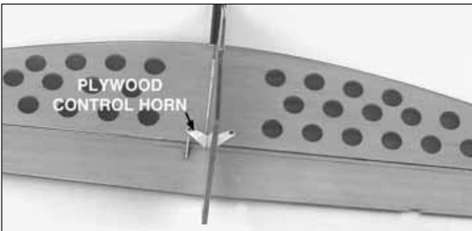
❑ 1. Slide the plywood **control horns** into the rudder and elevator, center, then glue with thin CA.
