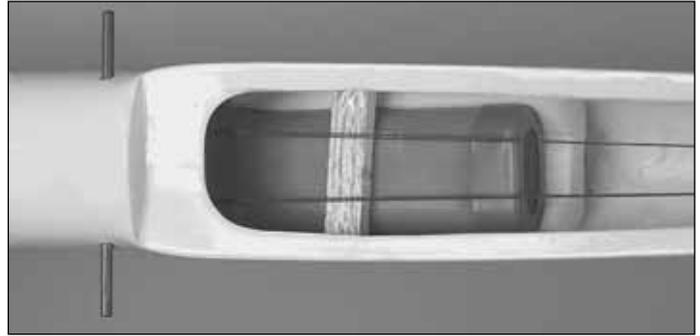
4. Place a piece of 1/4" [6mm] foam in the bottom of the fuse under the location of the battery. Slide the battery wire forward in the fuse under the servos. Hold the battery in place with a leftover piece of balsa and glue using medium CA.
