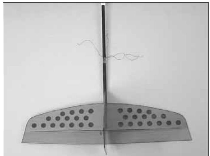
❑ 4. The center of the fin needs to be aligned with the center of the fuse.
