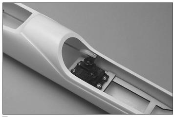
$\blacksquare$  18. Attach the pushrod to the servo using a Faslink connector.
