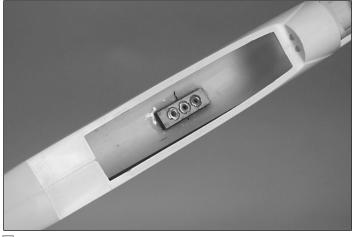
□ 5. Gently tap the three 4-40 blind nuts into the holes. Place a couple of drops of CA around the blind nut flanges to hold them in place. Do not get glue on the threads.
