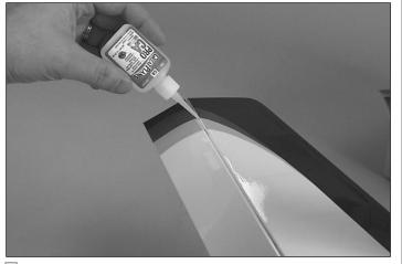
□ 2. Deflect the elevator completely one direction and place three to four drops of thin CA onto each hinge (not too much or it will run down the hinge line).
