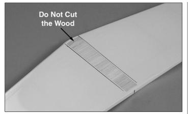
□ 5. Remove the covering inside of the marks. IMPORTANT!!! Do not cut into the wood or you will seriously weaken the structure.
