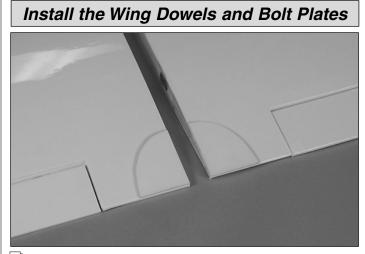
□ 1. Glue the two precovered wing bolt plates to the top of the wing at the trailing edge. *Hint: Remove the covering underneath for a good glue bond.*
