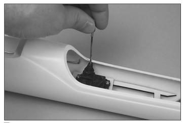
17. Enlarge the holes in the servo arm with a 5/64" [2mm] (or a #48 drill bit).
