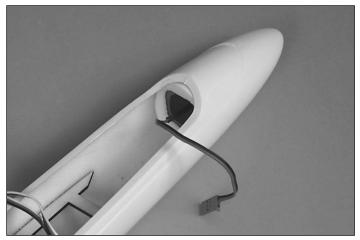
□ 1. Wrap the receiver battery with 1/4" foam rubber and install it as far forward in the nose as possible.
