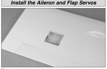
□ 1. Locate the openings for the flap and aileron servos in the bottom of each wing panel. Trim out the covering and seal the edges using a sealing iron.
