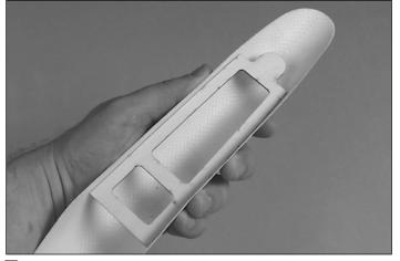
□ 5. Being careful not to move the canopy frame, tack glue the frame to the canopy with thin or medium CA. Recheck the fit onto the fuselage. Adjust its position as needed for a good fit.
