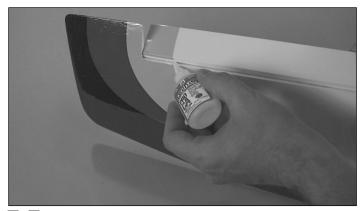
□ □ 3. Hold the aileron to full deflection and place three drops of thin CA onto each hinge. Flip the wing over and place three drops onto the other side of each hinge. Be careful not to use too much CA or it may run down the hinge line. Exercise the aileron several times to loosen it up.
