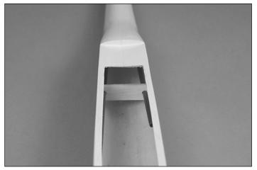
□ 7. Slide the plywood support over the guide tubes and position it where shown. Do not glue this yet.
