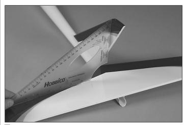
□ 6. Glue the fin in place using epoxy. Use a triangle to make sure the fin is exactly perpendicular to the stab. Check and double check this until the epoxy is completely cured.
