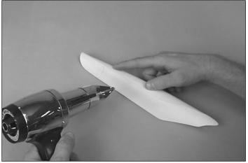
□ 1. Trial fit the canopy onto the fuselage. If the canopy does not fit snugly, use a heat gun to warm it up slightly and squeeze the sides closer together. Hold until completely cool. Repeat until the canopy fits perfectly. You may need to sand the edges slightly so it aligns perfectly with the canopy outlines on the fuselage.
