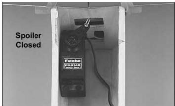
■ 8. Mount the wing onto the fuselage and pull the ends of the spoiler strings up to the spoiler servo. Position the spoiler servo horn at the rearward end of its swing and wrap one spoiler string around the screw in the horn. With the spoilers held closed, apply a drop of CA to glue the string to itself, forming a small loop. Remove that string and do the same steps to the other string. The two strings should be the same
