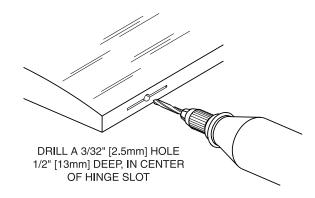
A. Drill a 3/32" [2.5mm] hole, 1/2" [13mm] deep, in the center of the hinge slot. If you use a Dremel® MultiPro™ for this task, it will result in a cleaner hole than if you use a slower speed drill. Drilling the hole will twist some of the wood fibers into the slot, making it difficult to insert the hinge, so you should reinsert the knife blade, working it back and forth a few times to clean out the slot.
