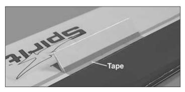
4. Tape the spoiler in position in the wing using a strip of cellophane or vinyl tape or a strip of covering. The tape should be flexible enough to allow the spoiler to close on its own. The tape should also be replaced occasionally as it will eventually rip.
