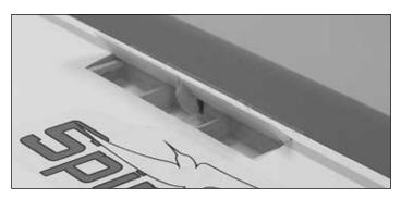
☐ 3. Cut the covering all around the edge of the **spoiler** and remove it from the wing panel.
