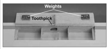
□ □ 6. Thread one end of the line through the small hole in the spoiler horn and use a piece of a round toothpick to hold the line in the horn. Allow about 1/2" [13mm] to hang out the other side of the horn for fine adjustments. It may be necessary to drill out the spoiler control horn using a 3/32" [2.5mm] drill bit. Trim the shear web to allow the toothpick to pass through without interference.
