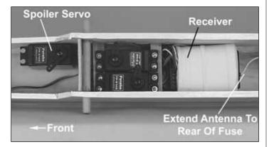
**Note:** If you are installing spoilers, mount the spoiler servo where the receiver is shown in the photo. It can be mounted on servo rails, or with servo tape. The receiver is then placed behind the servos used for the rudder and elevator. Cut three arms off an X-type servo horn and mount a small screw in the outer hole. Adjust the servo and your transmitter so the horn is almost pointing toward the rear of the plane when your transmitter stick is in the "spoilers closed"
