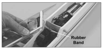
☑ 2. The canopy is held in place with a rubber band. Loop a medium size rubber band through the cut-out in the canopy back. Thread the rubber band through itself and then hook it on the little extension on the former. To remove the canopy, pick up on the back until the dowel is clear of the fuselage. To re-install the canopy just do the opposite.
