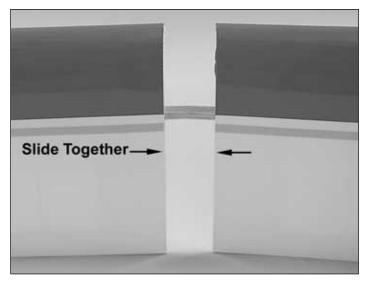
☐ 2. Check the fit of the wing joiner in the **wing panels**. Remove any excess material from the joiner to allow the panels to fit together. The joiner does not have to be glued into the wing. This will allow the wing panels to be separated for easier transportation.
