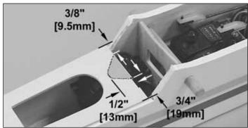
2. Place a piece of wax paper between the **bottom** canopy brace and fuselage. Glue the bottom canopy brace to the front canopy brace with CA. The wax paper will prevent the braces from accidentally being glued to the fuselage. **Note:** If you are planning on using the optional spoilers, you must remove the shaded area to allow for servo movement.
