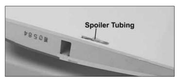
□ □ 2. Pull the end of the spoiler tubing out of the wing just far enough to glue it in place using thick CA.
