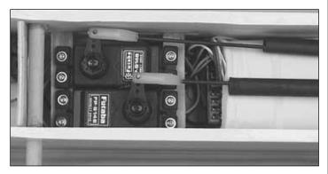
□ 11. Center the rudder and servo arm. Mark the pushrod wire at the servo arm. Bend the wire up at the mark. Cut the wire 5/16" [8mm] below the bend. Secure the pushrod to the servo arm with a nylon FasLink. Make sure the wire will not bind against the servo case. Repeat the process for the elevator pushrod.
