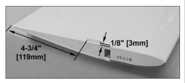
☐ 1. Use a hobby knife to cut a hole in the bottom of the wing sheeting for the **spoiler tubing** to exit the wing as shown.
