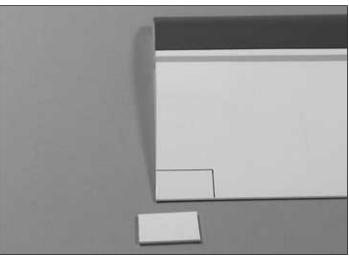
□ 3. Mark and remove a small area of the covering on both wings for the 1/8" x 1" x 1-5/8" [3mm x 25mm x 41mm] plywood **trailing edge plates**. Glue the plates onto the wing with thick CA.
