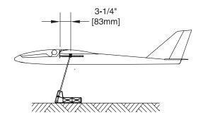
Accurately mark the balance point on the bottom of the wing on both sides of the fuselage. The balance point is located
