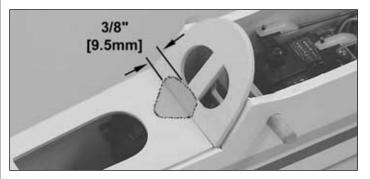
□ 3. With the wax paper still in place, glue the **rear canopy brace** to the bottom canopy brace with CA. **Note:** If you are planning on using the optional spoilers, you must remove the shaded area to allow for servo movement.
