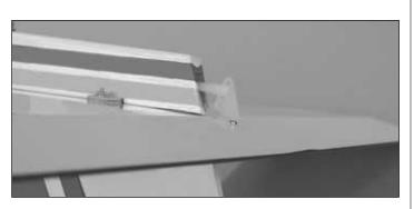
10. Install the elevator pushrod. Thread the clevis onto the pushrod. Attach the clevis to the control horn. Trim the opening at the rear of the fuselage as necessary to allow the pushrod to move freely.
