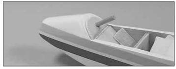
1. Place the small **hardwood dowel** into the **front canopy brace**. Remove the covering for the dowel in the front of the fuselage. Install the dowel into the hole.
