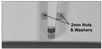
☐ 1. Find and open the holes in the **stabilizer** covering for the attachment screws. Attach the stabilizer to the **fuselage** using two **2mm x 15mm screws**, two **2mm nuts** and four **2mm washers**. Use thread lock on the nuts to prevent loosening.
