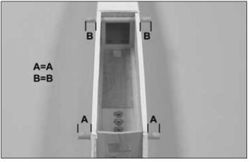
3. Install the **wing dowels** using medium or thick CA. Center the dowels in the fuselage before gluing.
