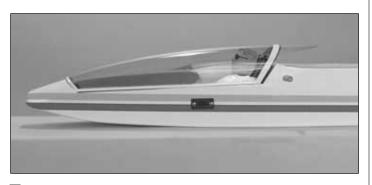
☐ 7. Test fit the canopy onto the fuselage. Trim the canopy flush with the base and the front but **do not trim the back yet!** Curved tip scissors works well for trimming the canopy. Temporarily mount the wing in place on the fuselage. **VERY CAREFULLY** trim the back of the canopy, **A LITTLE AT A TIME**, to fit over the wing. Take your time and use the outlines and the wing for guides.
