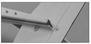
☐ 7. Position the remaining control horn in line with the center of the fuselage on the bottom of the elevator. Attach the control horn to the elevator using two 2mm x 15mm screws.
