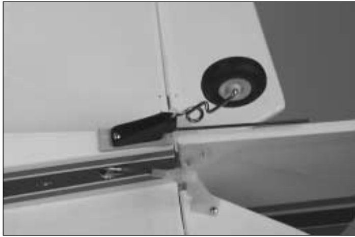
11. Screw the tailwheel assembly to the plate.
