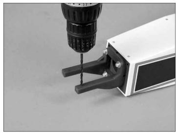
$\Box$  3. Remove the engine and drill the four mounting holes with a 9/64" (3.5mm) drill bit.
