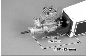
□ 1. Place the engine on the mount so that the propeller washer is 4.88" (124 mm) from the firewall and so the mounting flanges on the engine are within 1.25" (32 mm) from the ends of the mount.
