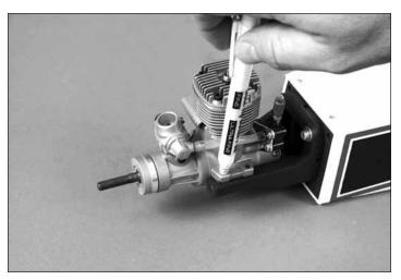
□ 2. Mark the position of the four mounting holes on the engine mount through the engine mounting flanges with a felt tip pen.
