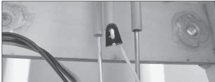
4. Install a strain relief onto the receiver antenna to protect the solder joint that secures it inside the receiver. A strain relief can be made by cutting off the end of an unused servo arm and stitching the antenna through two holes in the arm as shown. Route the antenna through the antenna tube and out the aft end of the fuselage.
