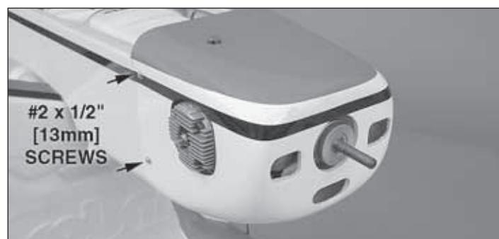
4. Drill 1/16" [1.6mm] holes at the marks you made on the cowl through the cowl mounting blocks. Remove the cowl and thread a #2 x 1/2" [13mm] self-tapping screw into each hole in the cowl mounting blocks and back it out. Apply a couple drops of thin CA to each hole in the blocks. Enlarge the four holes in the cowl with a 3/32" [2.4mm] bit. Install the cowl onto the fuselage using four #2 x 1/2" [13mm] self-tapping screws and four #2 flat washers.
