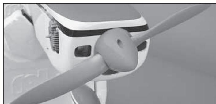
5. If necessary, ream or drill the spinner backplate to fit the crankshaft of your engine (or brushless motor prop adapter). Install the backplate onto the crankshaft followed by the propeller. Install the prop washer and prop nut. Depending on the size propeller you are using, you may need to enlarge the propeller blade cutouts in the spinner cone. When a good fit is achieved, use the screws included with the spinner to install the spinner cone onto the backplate.
