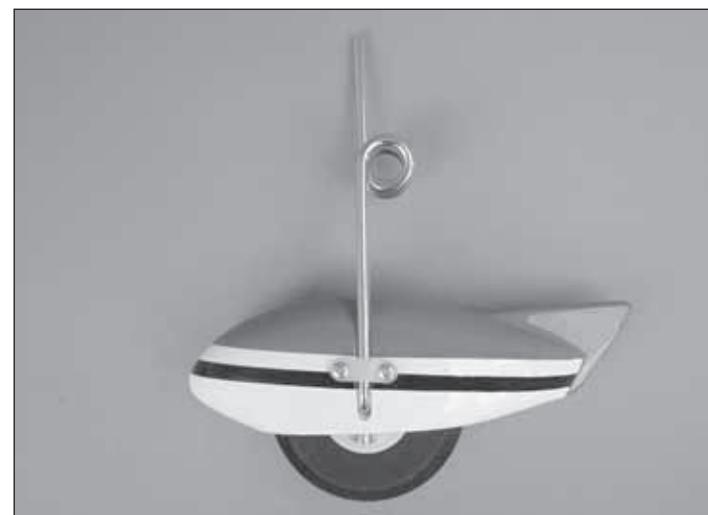
5. Install the nose wheel pant and wheel onto the nose gear wire in the same manner as you did the main landing gear.
