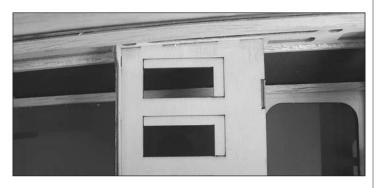
5. Page 14, Step 3 right column Install the Elevator Servo: If you intend to use standard sized servos for the Elevator and Rudder as in the manual it is necessary to cut away the tray tabs.
