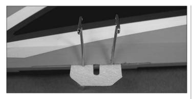
1. Install the CA Hinges: The hinges included with the model may be different than shown in the manual. Please follow these additional instructions to hinge the control surfaces.
