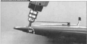
■ 5. Drill a 1/4" hole at each paint mark. The drill should be held perpendicular to the bottom surface of the wing. The bolts must thread into the blind nuts squarely.
