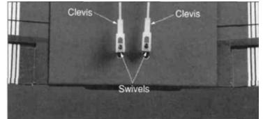
■ 3. Locate the nylon swivels and thread them onto the aileron torque rods until approximately 1/8" of threaded rod is showing above the swivel. Thread the clevises onto the control rods 15 full turns. Using the grooves on one side of the clevis as a guide, snap the clevis onto the swivel. (It may be necessary to use pliers to hold the control rod while threading on the clevises.)
