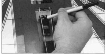
■ 4. Mark the control rod at the point that it crosses the control horn holes, 1/2" from the center of the servo control horn. Cut the control rod 1/4" past the mark and make a L-bend at that mark. Center the servo and insert the L-bend through the servo horn. Place a Nylon Faslink Pushrod Connector on the L-bend and servo horn to secure the pushrod. It may be necessary to enlarge the holes in the servo horn using a 5/64" drill bit.
