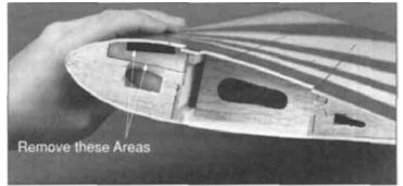
3. Using a hobby knife, remove the precut areas of the wing ribs on the two closest ribs to the wing root in both wing halves.
