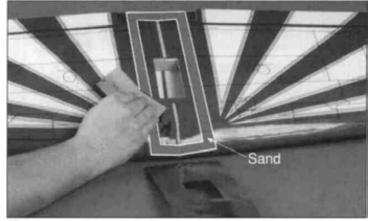
■ 9. Use medium grit sandpaper to lightly roughen the inside of each fairing where it will be glued to the wing. The area to be sanded is shown as a lightened area in the photograph. This will insure better adhesion of the fairing to the wing.
