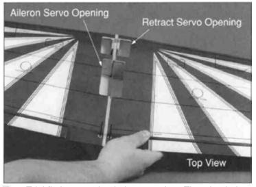
□ 7. Trial fit the two wing halves together. The wing halves should seat together without any gaps and the front and back edges of each wing should lineup with each other. Completely, cover the wing joiners, spars and center ribs.with 30-minute epoxy. Slide the two wing halves together, using masking tape to hold the wing in proper alignment until the epoxy cures.
