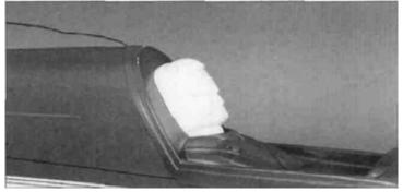
□ 5. Paint the pilot as you wish and glue it into the cockpit using CA. Let the CA cure completely before attaching the canopy to prevent fogging.
