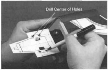
2. The front of the drive washer should be 4-13/16" from the firewall on all two cycle engines. Trial fit the cowling and spinner and strive for approximately 3/32" clearance between the spinner backplate and the cowling. If your engine includes a template, tape the template on the mount and mark the mounting holes. If your engine does not include a template, place the engine on the mount and make a mark through the lug holes. Drill a hole using a 7/64" drill bit at each mark.
