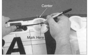
2. Using a pen, mark the landing gear wire at the center of the wheel well when the retracts are folded into the wing.
