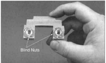
■ 2. Install the blind nuts into the holes from the bottom side of the mounting plate. Gently press the blind nuts into place with pliers or a vise. The holes may need to be enlarged slightly with a 5/16" drill bit. Glue the blind nuts into place with a drop of CA on the flange of the nuts. Care must be taken not to get CA into the threads of the blind nuts.
