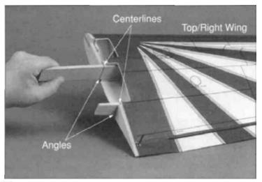
■ 4. Draw a centerline on both of the wing joiner pieces. Trial fit the wing joiners into both wing halves. A snug fit is desirable. If the joiners do not fit properly, lightly sand the excess epoxy and uneven surface joints from the joiner edges and sides. **Note:** The plywood and balsa wing joiners have a slight dihedral angle on one edge. This angle should be on the bottom of the wing.
