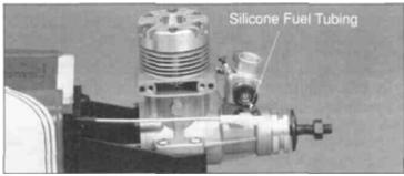
■ 2. (2-stroke Linkage) Thread a clevis onto the throttle pushrod. Place the clevis in the outermost hole on the throttle arm and secure with 1/4" of silicone fuel tubing. Place the throttle in the half open position and place a mark above the servo arm hole in the radio compartment. Cut the pushrod 1/4" past the mark. Make an L-bend in the pushrod at the mark and insert it into the servo arm, securing it with a pushrod keeper.
