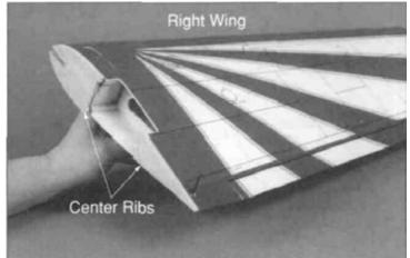
■ 3. Trial fit the center ribs on both wing halves, the ribs should not protrude beyond the outer covering of the wing. Lightly sand the ribs until they are flush with the wing covering. Use 6-minute epoxy to glue the plywood center ribs to the right wing half.
