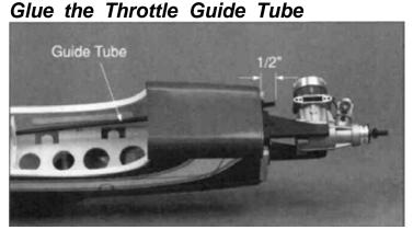
■ 1. Note: Read Steps 1-3 before proceeding. There is a throttle pushrod exit hole predrilled in the firewall to accommodate two cycle engines and four cycle engines if
