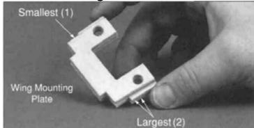
■ 1. Locate the three plywood wing mounting **plates.** Remove them from the die cut sheet and sand off any rough edges left from the die cutting. Glue the three mounting plates together in a stack with the shortest on the top. Make sure the holes are lined up with one another and wipe off any excess epoxy. Use clothespins to clamp the wing hold down plate together while the epoxy cures.
