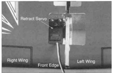
□ 6. Glue the retract servo tray mounting blocks into **the** wing as shown in the line illustration above. The servo tray should be glued to the servo tray mounting blocks. Mount the servo into place using the screws supplied with the servo. Trial fit the retract servo in the servo tray. Enlarge if necessary.
