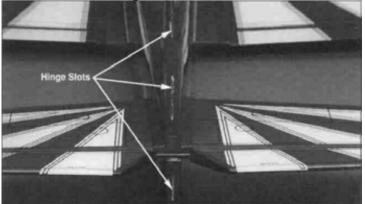
❑ 3. Check the rudder hinge slots to make sure they are open and receptive to the CA hinges. Clean the slots out with a hobby knife if necessary.
