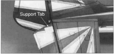
■ 1. Glue a support tab on each side of the elevator and rudder in the location where the control horns will be mounted. **NOTE:** *The support tabs are white in the photographs for better identification, but clear tabs are supplied in the kit.* Again place the control horns on the support tabs and mark their location and remove. Drill each mark with a 3/32" drill bit.
