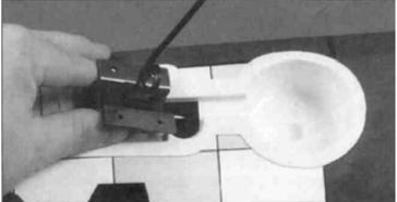
1. Insert the retract into the wing with the main landing gear wire facing toward the root of the wing when it is folded down.
