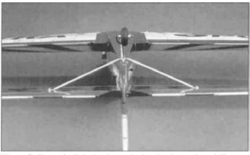
■ 2. Drill a 5/64" hole through the horizontal stabilizer at the point where the brace touches the stabilizer. Insert the 2x15mm machine screw from the top side of the stabilizer through the 2mm washer, 12mm clear plastic disc, horizontal stabilizer, 12mm clear disc, 2mm washer, brace and 2mm nut in that sequence. The nut should be secured using thread locking compound.
