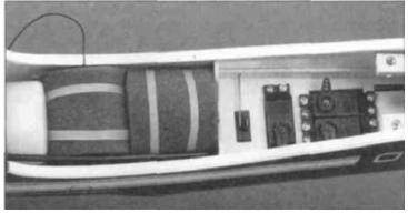
■ 1. Wrap the radio receiver and battery in protective foam. Using #64 rubber bands secure the receiver and battery in the radio compartment. There are four radio hold down tabs in the radio compartment to attach the rubber bands to.
