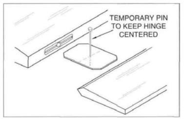
■ 4. Insert the hinges and install the rudder leaving a 1/32" gap between the rudder and fin. It is best to leave a very slight gap, rather than closing it up tight, to help prevent the CA from wicking along the hinge line. Make sure the rudder will deflect to the recommended throws without binding. Remove the rudder and insert a small pin through the center of each hinge. This pin will keep the hinge centered while installing the rudder. Insert the hinges into the fin.
