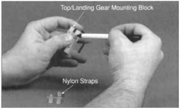
□ 2. Using a pen, place marks on the mounting blocks using the flat nylon straps as templates. Predrill the screw holes using a 1/16" drill bit and secure the strut with two nylon straps and four #2 x 3/8" sheet metal screws.
