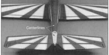
■ 3. Mix 30-minute epoxy to securely glue the horizontal stabilizer into place. Adjust the alignment of the stabilizer as described in Steps #1 and #2. Use T-pins to hold the proper alignment until the epoxy has firmly set. Wipe off the excess epoxy using rubbing alcohol and a paper towel. Set the fuselage aside to cure before proceeding.
