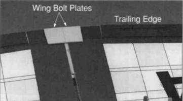
7. Using 6-minute epoxy, glue the plywood wing bolt plates to the bottom of the wing aligned with the trailing edge.
