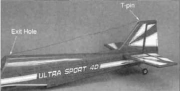
2. Route the antenna under the servo tray and up through an exit hole made with a T-pin behind the pilot in
