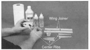
■ 2. Carefully glue the plywood center ribs and wing joiners together using 6-minute epoxy. The plywood joiner has a slight angle on one edge. Place these angles adjacent with each other. Use clothespins to clamp the joiner and ribs together. Remove the excess epoxy on the edge of the ribs and joiner using a paper towel and rubbing alcohol.
