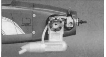
3. Install the muffler according to the manufacturer's recommendations. Attach the fill/pressure line to the muffler. Notice how the exhaust is pointed down and away from the fuselage and wing to help keep the aircraft clean.
