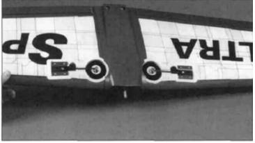
■ 13. Use 6-minute epoxy to glue the hardwood wing dowel into the leading edge of the wing. Work epoxy into the dowel hole using a sliver of wood. Apply epoxy to the dowel and insert the dowel. Leave 1/2" of dowel protruding from the wing. Apply the foam rubber seal to the front edge of the wing fairing (see Step 11, page 10). Clean the excess epoxy from the dowel using a paper towel and rubbing alcohol.
