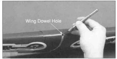
□ 10. Use thick CA+ to glue the top fairing to the top of the wing. Remove the plastic that is covering the wing dowel hole on the leading edge of the wing. Proceed to glue the bottom fairing to the bottom side of the wing and remove the remaining plastic covering the dowel hole.
