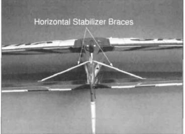
■ 1. Locate the two aluminum tubes that will be used to brace the horizontal stabilizer. Attach one end of each brace in the remaining hole in the tail gear bracket using a #4 x 1/2" sheet metal screw. (Also, see the photo at Step 5, Page 20).
