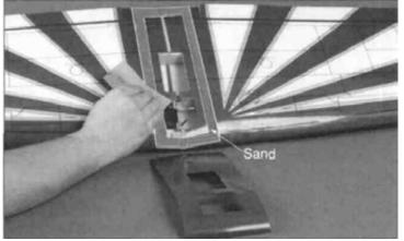
■ 11. Use medium grit sandpaper to lightly roughen the inside of each fairing where it will be glued to the wing. The area to be sanded is shown as a lightened area in the photograph. This will insure better adhesion of the fairing to the wing.
