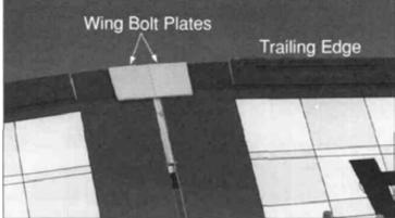
9. Using 6-minute epoxy, glue the plywood wing bolt plates to the bottom of the wing aligned with the trailing edge.
