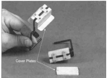
3. Use 6-minute epoxy to glue the plywood landing gear cover plate to the mounting block.
