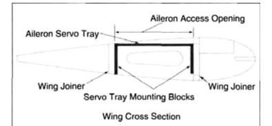
■ 1. Trial fit the servo into the servo tray. Locate the plywood servo tray mounting blocks and glue them into the aileron servo tray opening using 6-minute epoxy. The tray should be flush with the top of the wing joiners installed earlier in Step 6, Page 7.
