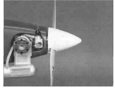
■ 4. Place the spinner backplate onto the engine shaft followed by the propeller. Secure the propeller in place with the engine driver washer. Snap the spinner into place onto the backplate. Check the area on the spinner around the propeller for contact between the spinner and the propeller. If there is contact, trim the spinner a little at a time until it is eliminated.
