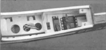
3. Cut three of the arms off the "cross" servo horn and mount to the servos as shown.
