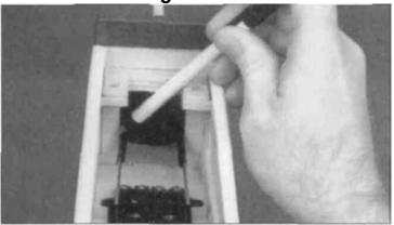
3. Temporarily insert the pushrods into the guide tubes. Lay the pushrods on top of the servo horns. Mark the fuselage formers next to the pushrod guide tubes. **Note:** The pushrod guide tubes are intentionally installed so the tube exits the fuselage on the opposite sides of the controlling servo. They cross inside the fuselage allowing the pushrods to run nearly straight, from the servos to the control horns, for maximum rigidity. Remove the control rods.
