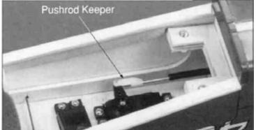
□ 4. Install the pushrod keeper over the L-bend and servo horn, and snap it onto the rod.
