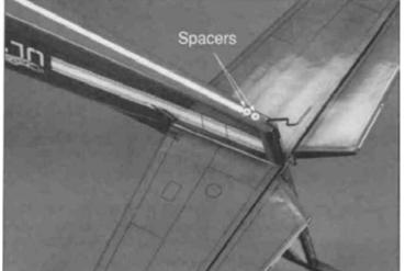
2. Locate and glue the two aluminum spacers into the bottom tail section of the fuselage.
