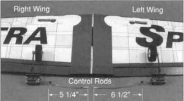
4. Bend the pushrods to match the line drawing on page 5. The pushrods should look like the assembled retracts shown in the photograph above, if you are using Hobbico Main Retracts (HCAP4010).
