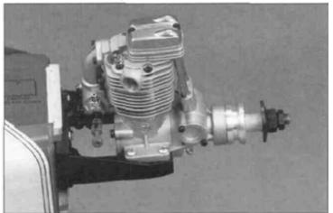
2. Put a drop of oil in each hole and install the engine using the four #6 x 3/4" sheet metal screws provided.
