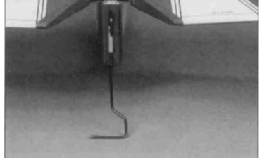
■ 1. Apply petroleum jelly to the tail gear to prevent glue lock up. Use 30-minute epoxy to glue the tail gear guide tab into the fuselage. Complete the next two steps before the epoxy is allowed to completely set up.
