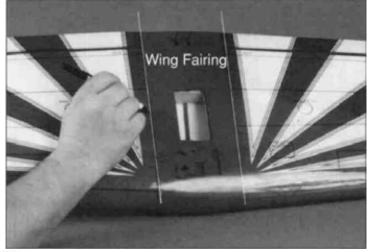
8. Individually place the top and bottom plastic wing fairings on the wing and lightly trace its outline onto the wing.
