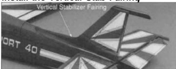
■ 2. Locate the plastic vertical stabilizer fairing and lightly sand the underneath side of the fairing. Slide the fairing over the vertical stab and lightly trace its outline onto the fuselage. Remove the fairing. Lightly sand the fuselage on the inside of the line. Using thick CA+, apply a bead of glue to the fuselage and slide the fairing into place, holding firmly until the glue dries. The vertical stabilizer relies on this fairing for structural support; therefore a good bond is essential.
