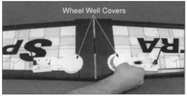
5. Locate and glue the two white plastic retract wheel well covers in place using medium CA.
