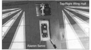
■ 2. Mount the aileron servo in the servo tray using the screws, grommets and rubber mounts supplied with servo. Place the control horn on the aileron servo in the neutral position.
