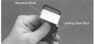
I. Place the landing gear mounting block between the U-bend on the top portion of the main landing gear strut.
