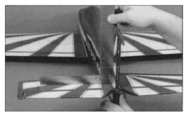
■ 1. Carefully align the vertical stabilizer on the horizontal stabilizer. The vertical stabilizer must be perpendicular to the horizontal stabilizer and **must line up with the fuselage centerline exactly.** Using 30-minute epoxy, glue the vertical stabilizer into place. A square should be used to assure a perfect 90° angle between the horizontal and vertical stabilizer. Pin the vertical stabilizer in place and keep checking its alignment by measuring and sighting until the epoxy sets up.
