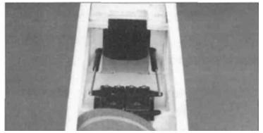
■ 4. Remove a small portion of the fuselage former using a hobby knife or round file. The guide tube should fit into the former flush to the edge. **Do not** remove any more former than necessary or it will be weakened. Use medium CA to glue the guide tubes into place.
