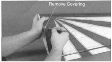
□ 1. Remove the foam covering from the aileron servo opening. The covering has been partially precut for exact location.
