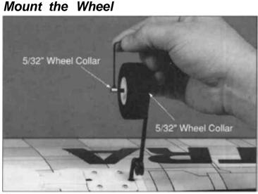
❑ 6. Mount the wheels using the four 5/32" wheel collars.
