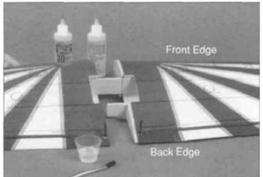
6. Trial fit the two wing halves together. The wing halves should seat together without any gaps and the front and back edges of each wing should line up with each other. Completely cover the wing joiners, spars and center ribs with 30-minute epoxy. Slide the two wing halves together, using masking tape to hold the wing in proper alignment until the epoxy cures.
