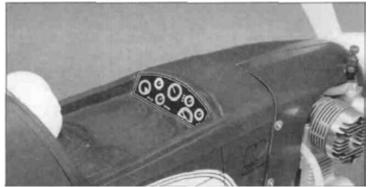
6. Place the instrument panel decal into the cockpit.
