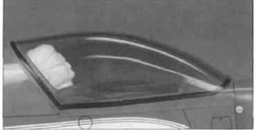
■ 7. Glue the canopy in place on the fuselage. We have had good luck using RC-56 glue when installing canopies. It takes a few hours to dry, but it is very clear and looks good in the end. To hide the canopy glue joint and to seal out fuel residue, you can use 1/8"-1/4" wide striping tape as a border around the canopy.
