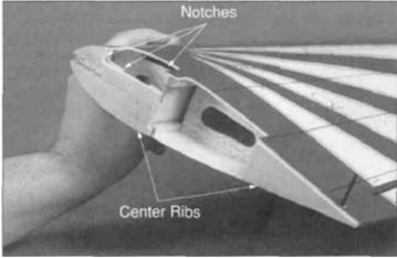
for a proper fit. The ribs should not protrude past the outer skin of the wing. Lightly sand the edges of the center ribs until they are flush with the wing covering. Glue the plywood center ribs to the right wing half. Note: Notice the positions of the notches removed from the center and wing ribs for the retract pushrods when aluing the plywood rib onto the wing.
