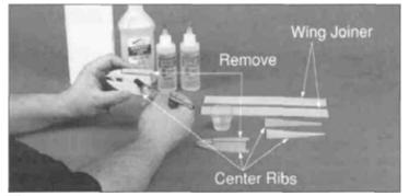
2. Remove the precut area from the front center rib before gluing. Carefully glue the plywood center ribs and wing joiner together using 6-minute epoxy. The plywood joiner has a slight angle on one edge. Place these angles adjacent with each other. Use clothespins to clamp the joiners and ribs together. Remove the excess epoxy on the edge of the ribs and joiner using a paper towel and rubbing alcohol.
