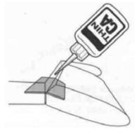
□ 1. Check each of the ailerons and the elevator to be sure that they are secure. If any of them seem loose, apply a few drops of thin CA glue to both sides of the hinge as shown above. Do not remove the hinge to do this. The glue will wick into the wood and provide a strong joint.
