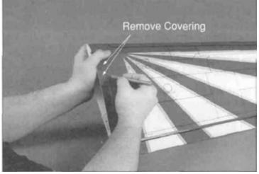
1. Remove the foam covering from the aileron and retract servo openings. The skin has been partially precut for exact location.
