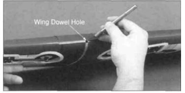
■ 12. Use thick CA+ to glue the top fairing to the top of the wing. Remove the plastic that is covering the wing dowel hole on the leading edge of the wing. Proceed to glue the bottom fairing to the bottom side of the wing and remove the remaining plastic covering the dowel hole.
