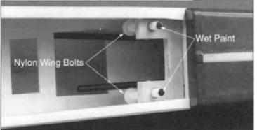
■ 4. Insert the nylon wing bolts from the underneath side of the wing mounting plate. The bolts should be even with the wing seating tape. They should touch the wing lightly when the wing is fully seated in the wing saddle. Paint the tip of the bolts with a slow drying paint. Before the paint dries, place the wing into the wing saddle. The wet paint will mark the locations that will be drilled for the wing bolts.
