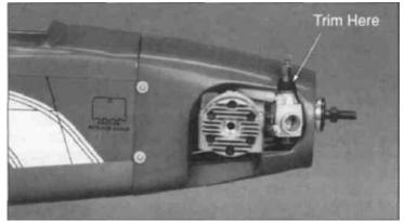
□ 1. Trial fit the cowling into place on the fuselage and mark the cowl where it interferes with the needle valve and any part of the engine or muffler. Cut an undersized hole in the marked areas on the cowl and trial fit it again. Continue to carefully cut and fit the cowl until it fits properly without touching the engine. Only a small portion of the cowl should need to be removed for a proper fit.
