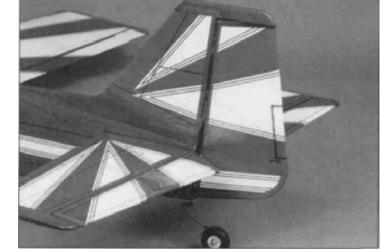
□ 2. Before mounting the rudder, use a hobby knife to enlarge the slot in the leading edge of the rudder to provide plenty of clearance for the tail gear wire. Clean the tail gear wire off with rubbing alcohol.
