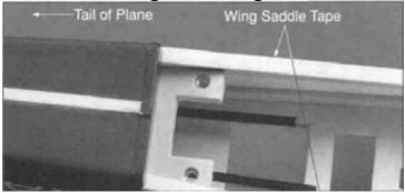
■ 3. Install the wing mounting plate into the cut-outs in the sides of the fuselage. The tabs created by the two longest plates fit into the notch in the lightening holes in both sides of the fuselage. The back of the block fits into the bulkhead. Use 6-minute epoxy to securely install the wing mounting block into the fuselage. Apply 1/8" wing seating tape to each side of the wing saddle to prevent exhaust residue from entering the fuselage.
