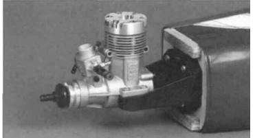
3. Put a drop of oil in each hole and install the engine using the four #6 x 3/4" sheet metal screws provided.
