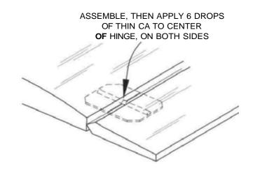
■ 6. After the epoxy cures, apply 6 drops of thin CA to both sides of each hinge, allowing a few seconds between drops for the CA to wick into the slot. **Note:** The small "tunnels" you created by drilling the 3/32" holes allow the CA to freely travel in to the entire surface of the hinge, producing an extremely secure bond.
