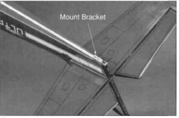
□ 3. Locate the metal tail gear mount bracket and slide it over the tail gear wire. Secure the bracket to the fuselage with one  $#4 \times 1/2$ " sheet metal screw. Use the hole closest to the tail gear at this time.
