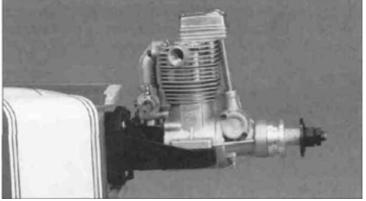
1. Trial fit the cowling and spinner. Strive for approximately 3/32" clearance between the spinner backplate and the cowling. If your engine includes a template, tape the template on the mount and mark the mounting holes. If your engine does not include a template, place the engine on the mount and make a mark through the lug holes. Drill a hole using a 7/64" drill bit at each mark.
