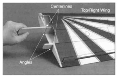
■ 5. Draw a centerline on both of the wing joiner pieces. Trial fit the wing joiners in both wing halves. A snug fit is desirable. If the joiners do not fit properly, lightly sand the excess epoxy and uneven surface joints from the joiner edges and sides. The plywood joiner has a slight angle on one side, which should face the bottom of the wing.
