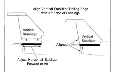
**Note:** When mounting the horizontal stabilizer do not slide the stabilizer fully forward in the saddle. Instead, position the stabilizer in the location where the trailing edge of the vertical stabilizer will line up with the aft edge of the fuselage, thus providing a straight hinge line for the rudder. Trial fit the vertical stabilizer before mounting the horizontal stabilizer to make sure you are locating the horizontal stabilizer correctly.
