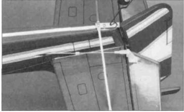
□ 5. Thread the nylon clevises onto the pushrods 15 full turns. Pliers may be required to hold the rod while threading the clevis onto the rod. Use a piece of cloth to keep from scratching the pushrod. Install the pushrods into the guide tubes with the clevises at the elevator and rudder. Connect the clevises to the control horns and use the pushrods as guides to mark the control horn locations
