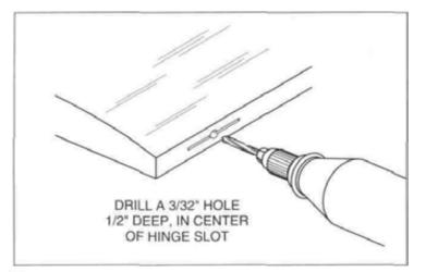
□ 3. Drill a 3/32" hole, 1/2" deep, in the center of the hinge slot. If you use a Dremel" Moto-Tool for this task, it will result in a cleaner hole than if you use a slower speed power or hand drill. Drilling the hole will twist some of the wood fibers into the slot, making it difficult to insert the hinge. Insert a standard #11 hobby knife into the slot, working it back and forth a few times to clean out the slot.
