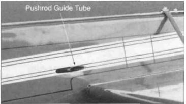
■ 2. Apply masking tape to the fuselage next to the guide tubes to protect the fuselage skin while cutting. Roughen the end of each tube with medium sandpaper. Using 6-minute epoxy glue the tubes in place. Trim the guide tubes flush with the edge of the fuselage.
