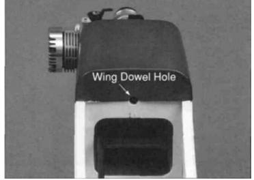
6. Trim away the plastic that covers the wing dowel hole in the front of the radio compartment.
