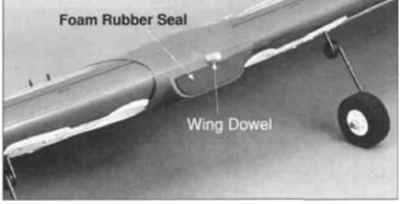
■ 11. Use 6-minute epoxy to glue the hardwood wing dowel into the leading edge of the wing. Work epoxy into the dowel hole. Apply epoxy to the dowel itself and insert the dowel. Leave 1/2" of dowel protruding from the wing. Clean the excess epoxy from the dowel using a paper towel and rubbing alcohol. Apply the foam rubber seal to the front edge of the wing fairing. It will help prevent exhaust residue from leaking into the fuselage.
