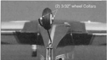
4. Mount the tail wheel using two 3/32" wheel collars.
