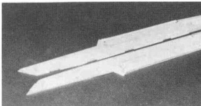
D 6. Go back to step 2 and assemble the **RIGHT** fuselage side. The easiest way to do this is to pin the other fuselage side upside down above the one you just built as shown in the photo. **MAKE SURE YOU ARE NOT BUILDING TWO IDENTICAL SIDES, THEY SHOULD BE THE OPPOSITE OF EACH OTHER.**
