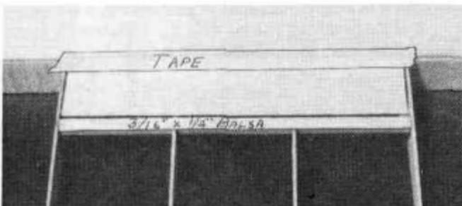
D 22. Test fit the spoiler in its bay and sand it if necessary to achieve a 1/32" gap around the sides and trailing edge. Use a strip of masking tape to temporarily hinge the spoiler in place.
