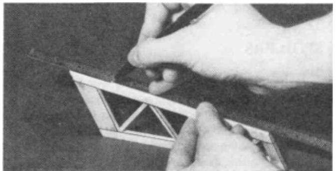
D 6. Carefully draw a **centerline** all around the edges of the rudder and fin (this will help to maintain symmetry when sanding).
