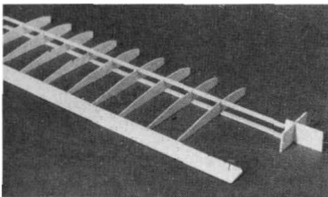
DD 10. Trial fit the top 1/8" x 5/16" x 23-1/2" Basswood **Inner Spar** (SPRTW13) into the notches in the ribs by carefully pushing the spar completely down into the notches. Make sure the top spar is lined up lengthwise with the bottom spar. Remove the spar and glue it in place by applying thick CA to the notches before the spar is put back in place.
