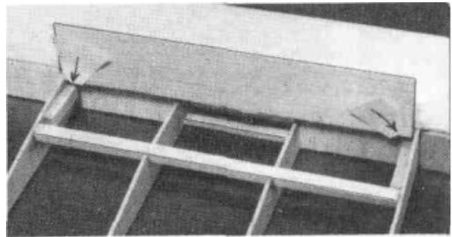
D 23. With the spoiler in place, glue the 3/16" x 1/4" x 1-1/4" pieces of balsa to ribs W2. These are the spoiler rests and should be positioned so they hold the spoiler flush with the top surface of the wing. **NOTE: It is important that the spoiler sit flush with the top of the wing or it will unnecessarily disrupt the airflow over the wing.**
