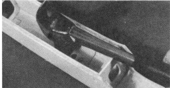
inside of the fuselage) with a hammer and put a drop of thick CA around the outside edge of each blind nut (be careful not to get glue inside the blind nut!).
