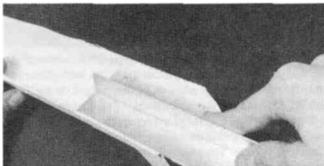
D 2. Sand the bottom edges of the canopy front and back flush with the bottom of the cockpit. Be careful not to sand through the cockpit. A small flat file works well for the front former.
