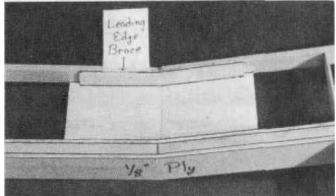
D 9. Locate one of the 1/16" x 3" x 24" **Balsa Sheets** (SPRTW17) and cut it into 6 pieces 2-3/8" long. Slide one of the sheets in place in front of the dihedral brace, trim it to fit and glue it to the LE and the dihedral brace with thick CA.
