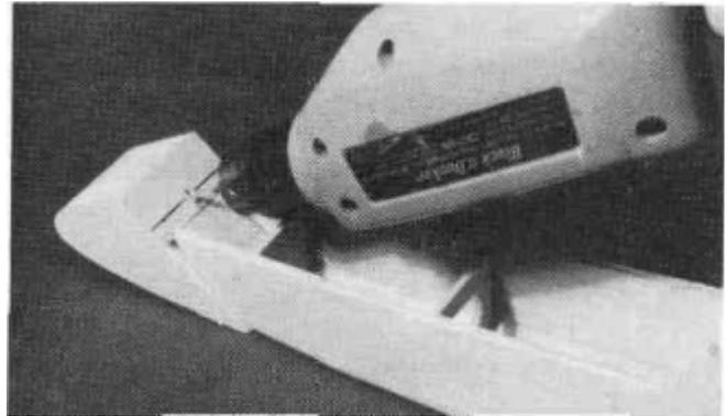
D 10. Measure up along the nose block 1/4" from the fuselage side and make a mark. Do this on both sides of the nose block and then draw a line across between the two marks. Measure to the middle of this line and make another mark. Drill a 1/8" diameter hole about 1" deep at approximately the angle shown on the plans right where you made the last mark.
