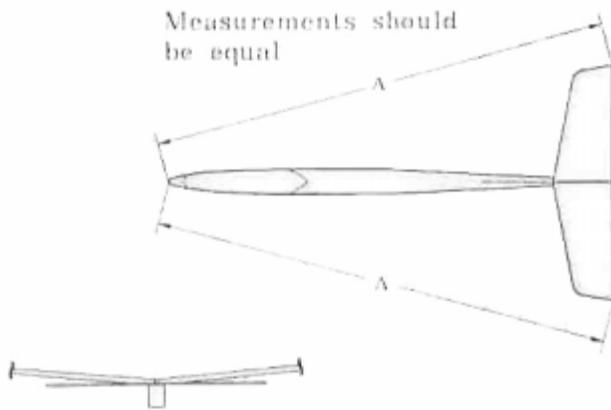
D 3. Position the stabilizer on the fuselage and measure to get it centered and properly aligned. Glue the stabilizer to the fuselage with either thick CA or epoxy. Check its alignment with the wing while the glue is curing to make sure they are level with each other.
