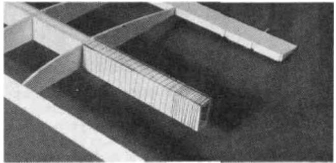
DD 19. Tightly wrap the joiner box with a strong thin thread and then soak it with thin C/A. This will add a lot of strength to the joiner box. Do not overlap the thread or allow it to build up too thick.
