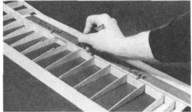
and act as a lunge for the gluing process. Press the sheeting into place and trim it flush with the back edge of the spar using a modeling knife and straightedge.
