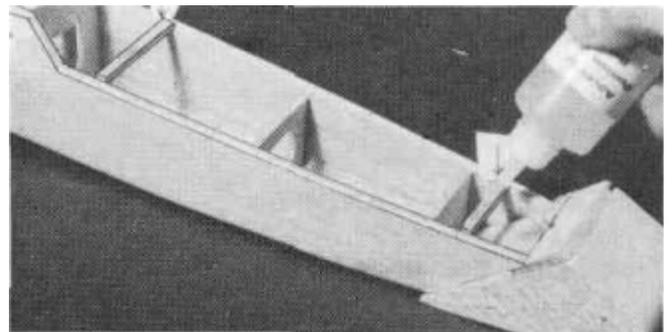
D 12. Cut two pieces of 1/8 x 3/16" balsa (from SPRTS03), one 1-7/8" long and the other 1-1/4" long. Wedge the longer piece between the fuselage sides above the receiver compart-
