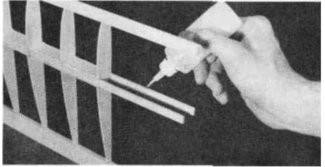
DD 18. Remove the clamps and apply a bead of epoxy along the spar edges (thick CA will also work but be very careful to get things aligned properly before the glue cures). Install the braces and hold in place with the C1 clamps. A good glue joint is important here but be careful not to get any excess glue inside the box formed by these braces or the wing joiner will not fit inside. Also test the size of the joiner box with the joiner lamination while the glue is curing.
