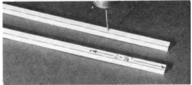
D 5. Drill a 5/64" hole 2-1/4" in from both ends of each pushrod.
