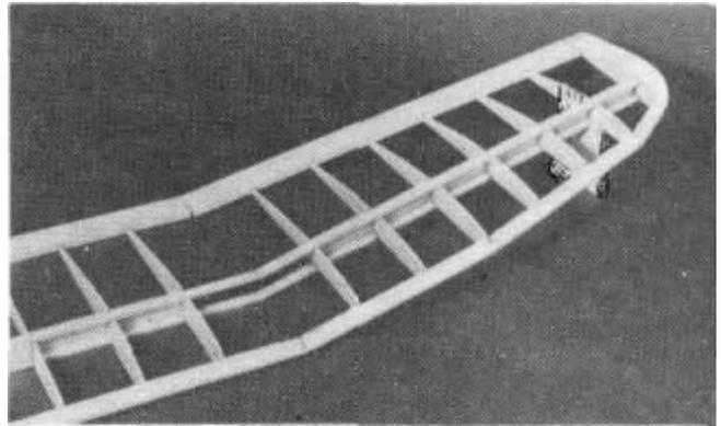
DD 3. Test fit the inner and outer panels together over the plan to make sure the leading edges, spars, and trailing edges all meet up nicely when the tip panel is blocked up the required 2-5/8" at the bottom of rib W 10 (Use the **lower** notch of the dihedral gauge at W9 as shown on the plans to obtain the correct angle). Sand any ends if needed to make everything fit well.
