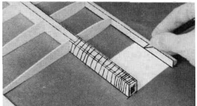
DD 20. Locate one of the 1/16" x 3" x 30" **Balsa Sheets** (SPRTW 17) and cut it into 6 pieces 2-3/8" long. Slide one of the sheets in place in front of the joiner box and trim to fit. Use another sheet to shim up the front edge (See sketch nextpage). **Glue** it in place with thick CA.
