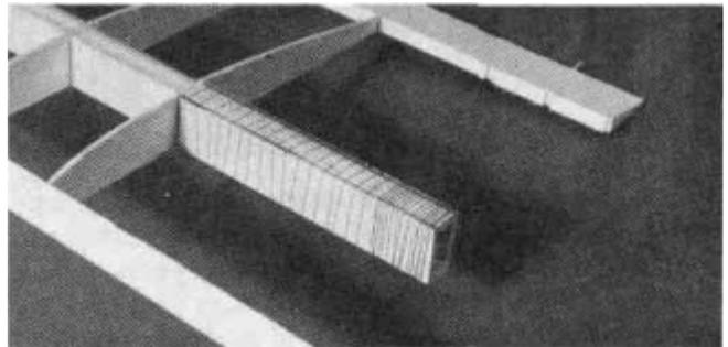
DD 19. Tightly wrap the joiner box with a strong thin thread and then soak it with thin C/A. This will add a lot of strength to the joiner box. Do not overlap the thread or allow it to build up too thick.
