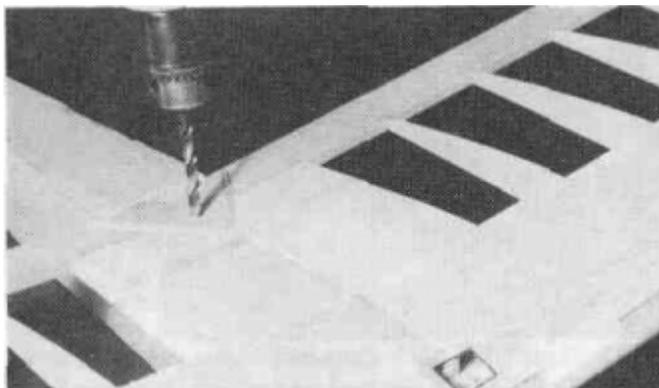
D 15. Drill a 13/64" hole through the wing and 1/4" ply plate in the fuse approximately 1" behind the front of the leading edge. Drill another 13/64" hole approximately 1-1/4" in front of the rear of the trailing edge as shown on the FUSELAGE SIDE VIEW of the plans.
