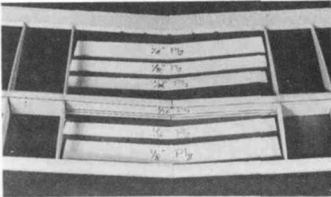
D 6. Punch out all four of the **Wing Joiner Laminations**, the **Dihedral Braces** and the **Leading Edge Brace** from the die-cut sheets SPRTW04 and SPRTW05. Test fit all of the pieces in place and sand them if necessary to make them fit nicely. The wing joiner laminations are installed between the spars and arc sandwiched in place by the dihedral braces. The C1 clamps can be used to hold everything in place.
