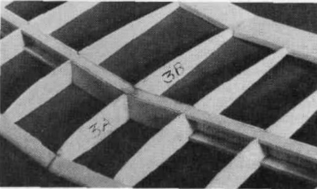
DD 7. Glue the 1/32" Plywood Polyhedral LE Brace (from SPRTW06) in place against the leading edges. Install ribs **W3A** and **W3B** between the inner and outer panels using thick CA as shown in the photo. A little sanding may be necessary to achieve a good fit. Use the rib gauge to tilt the ribs to the proper angle.
