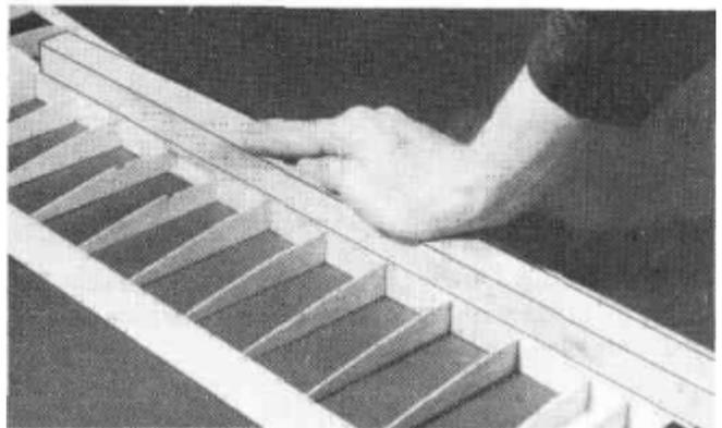
D 17. Lift the sheeting up and apply a bead of thick CA along the top spar. Quickly press the sheeting down into place and hold until the glue has cured. A **straight** strip of wood the length of the panel can be a big help when trying to hold the sheeting down evenly.
