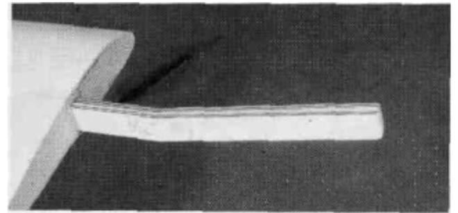
D 3. Sand the edges of the finished "wing joiner" to remove any glue globs and test fit it in the wing joiner box. Some sanding may be required to get a nice smooth **but not** loose fit.
