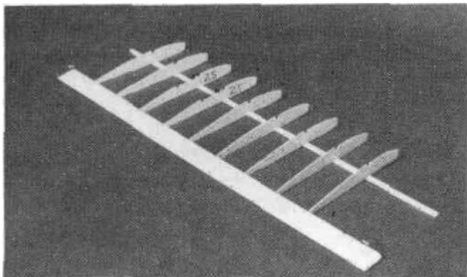
DD 9. Make sure the ribs are properly positioned according to the plans and glue them in place using thick CA at the spar joint and a drop of thin CA at the trailing edge joint. Use the square end of the rib gauge to keep the ribs perpendicular to the work surface. **NOTE: if you are installing spoilers, cut out the embossed area on the two W2S ribs and make sure you install these ribs in the proper locations.**
