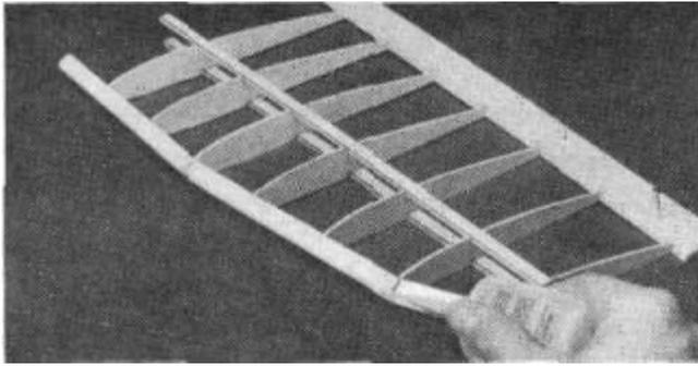
DD 6. Carefully bend the leading edge to the angle shown on the plans and position it against the ribs. The bends should be at ribs W6 and W9. Align the leading edge with the top and bottom edges of the ribs and glue it in place starting at ribs W6 and W9.
