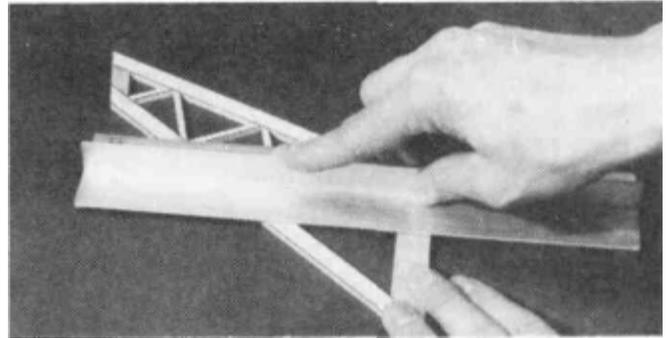
D 4. Remove the fin and rudder assemblies from the plan and examine them for any open or bad joints. Fill any gaps with thick CA, then use your sanding block with medium grit sandpaper to sand both sides of the framework smooth.
