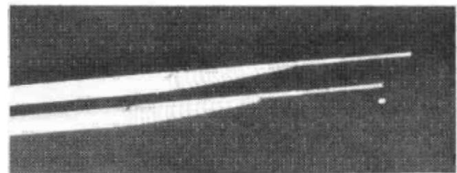
D 7. Insert one threaded piece of wire into each pushrod. Insert the 12" pieces of wire into the other end of each
