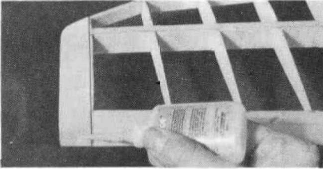
DD 13. Apply several drops of thin CA to the rear portion of the balsa wing tip. Allow the glue to soak into the wood and cure. The glue will help harden the wood and protect it from damage.
