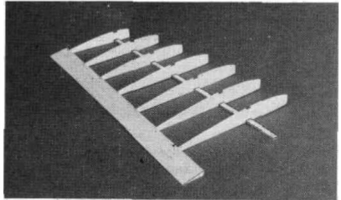
DD 3. Punch out the 1/16" (W4-W10) Tip Ribs out of one of the SPRTW03 die-cut sheets. Glue the ribs in place with a thick CA at the spar joint and a drop of thin CA at the trailing edge joint. Use the rib gauge to keep the ribs perpendicular.
