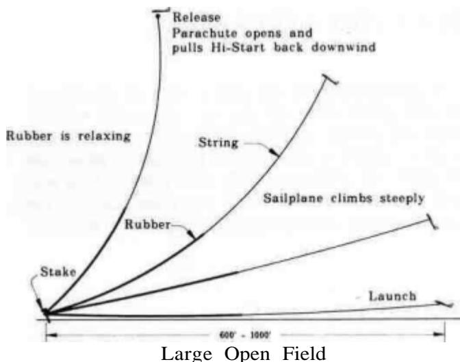
Follow the directions that came with the hi-start and lay it out directly into the wind. Place the stake at the far **upwind** edge of the flying field so the parachute will blow back onto the flying field.
