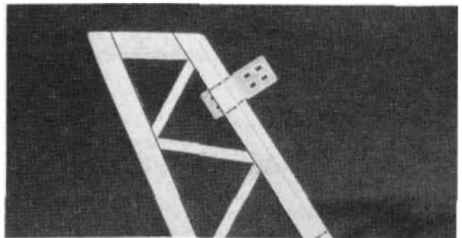
D 4. Insert the hinges into the slots and trial fit the rudder and elevator in place on the fin and stab. **Do not glue the hinges until after you have covered the model.**
