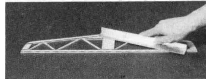
D 4. Remove the stab from the plan and examine it for any open or bad joints. Fill any gaps with thick CA, then use your sanding block with medium grit sandpaper to sand both sides smooth. Draw a centerline around the stab edges.
