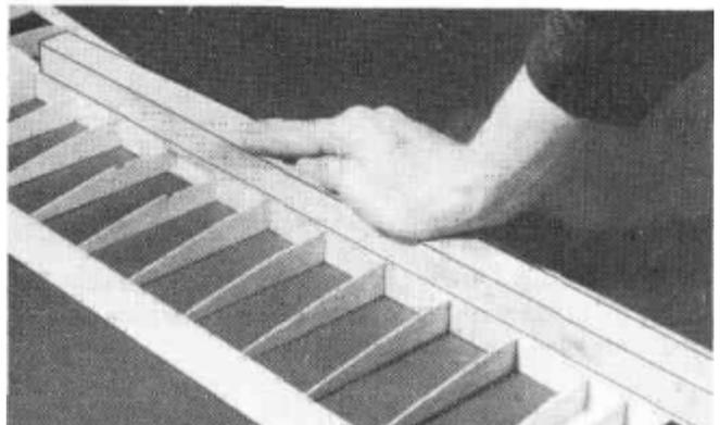
D 17. Lift the sheeting up and apply a bead of thick CA along the top spar. Quickly press the sheeting down into place and hold until the glue has cured. A **straight** strip of wood the length of the panel can be a big help when trying to hold the sheeting down evenly.
