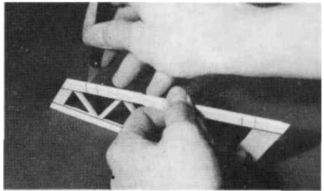
D 2. Draw accurate centerlines down the trailing edge of the stab and the fin. Cut the hinge slots **on these lines** using a hobby knife or a slotting fork and slotting hook. (The recommended hinge slotting technique is listed below).
