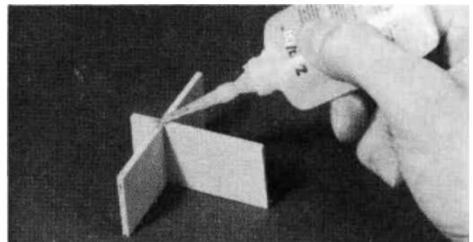
DD 8. Punch out the two **Rib Gauge Pieces** from the 1/8" die-cut plywood sheet (SPRTW08) and assemble them using CA. Notice that one end of the gauge is slanted at a 5 degree angle for positioning the end ribs. The other 3 ends are perpendicular and can be used to keep parts 90 degrees to the work surface.
