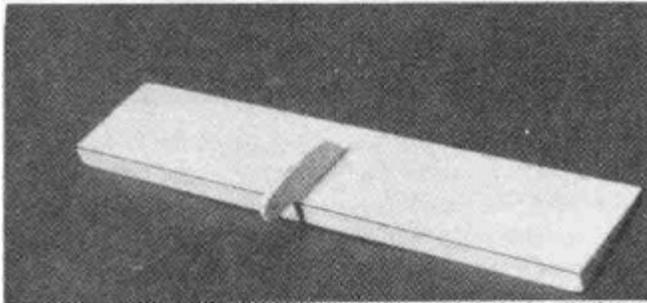
D 26. Drill a 1/16" hole in each **1/16" Die-Cut Plywood Spoiler Horn** (SPRTW05) at the indentation. Cut a 1/16" wide slot in the spoiler for the spoiler horn using a razor saw (a hack saw blade will also work fine) and glue the horn in place. It should be flush with the top surface of the spoiler as shown on the plans. This completes the assembly of the spoilers until after the wing is covered.
