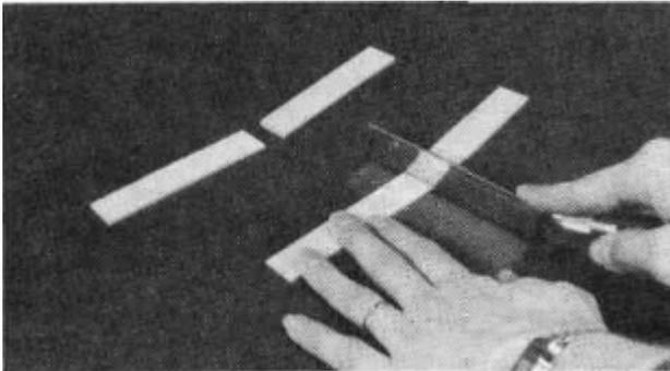
DD 16. Punch out the two dihedral braces and cut them in half with a razor saw along the lines you just drew. **Note: these braces are supplied in one piece for the bolt on wing option.** Also punch out the wing joiner lamination from that sheet and set it aside for the next step. The leading edge brace is not used in a two-piece wing.
