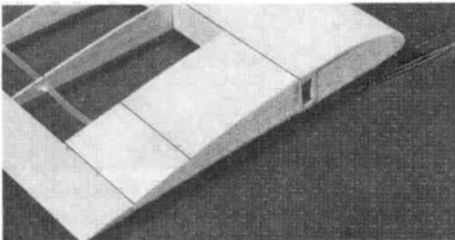
D 28. Use the remaining piece of 1/16" balsa sheeting to sheet the top inboard center section out past rib **W1B** as shown in the photo. Thick CA should be used for this step. Pre-cut the sheeting to fit first near the spars, and cut a second piece to fit between the first piece and the trailing edge. Glue these in place and if you built a two-piece wing, sand the sheeting flush with the **W1A** and **W1B** ribs at the wing root.
