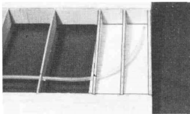
D 25. If you are using the spoiler setup shown on the plans, the spoiler tube should exit the bottom of the wing just behind the wing joiner box and the nylon tube should protrude approximately 4" to help the spoiler string clear the servos in the fuselage. Drill a 1/8" hole in the bottom center section sheeting for the tube, insert the tube in place and glue the tube to every rib and the sheeting using thick CA.
