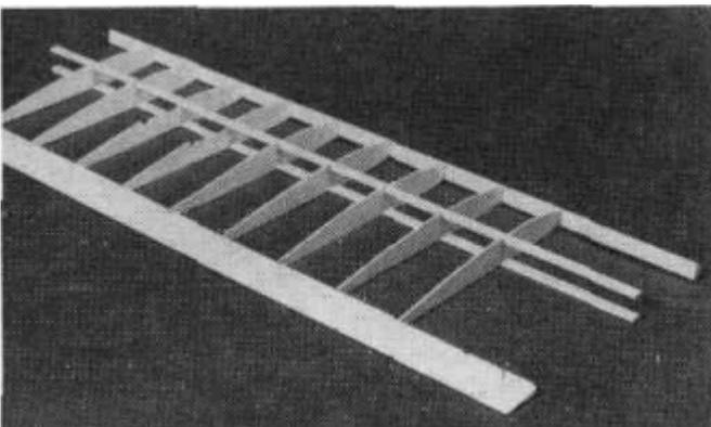
DD 11. Position a **Pre-shaped Leading Edge** (SPRTW10) in place over the plans. **NOTE: These leading**
