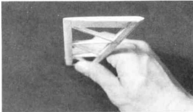
**\* MAXIMUM PERFORMANCE TIP -** Sand both sides of the rudder to a taper as shown on the plans. This requires a little more work but will help to reduce drag and thus increase performance of the sailplane.
