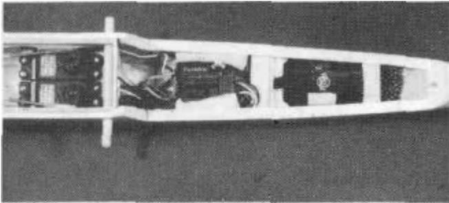
D 10. The battery pack should be wrapped in 1/4" of foam also and it should be positioned between formers F2 and F3.
