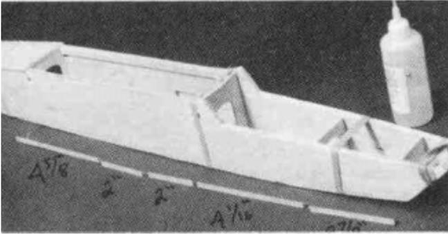
These pieces should be glued with thick CA. They are pressed into the corner between the fuselage bottom and the fuselage doubler in the following places:
