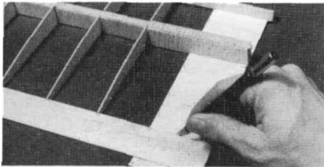
DD 20. Glue another piece to the rear of the joiner box and then cut a third piece to fit behind the second and glue it in place.
