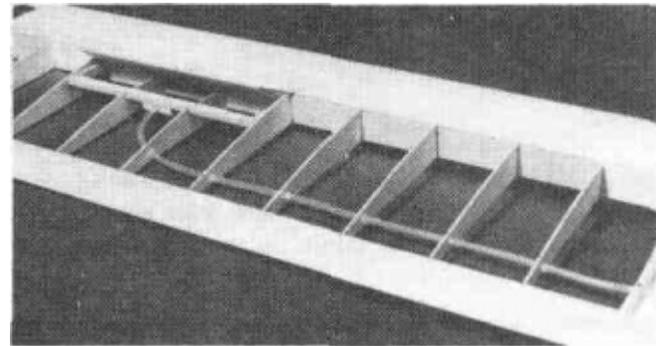
D 24. Drill 1/8" holes in the ribs as indicated on the plans and snake a 1/8" diameter nylon tubing (Inner pushrod tube or antenna tube, not included) through the ribs. Cut a 1/8" wide, 1/8" deep notch in the middle of the 3/16" x 1/4" x 1" piece of balsa and glue it to the bottom of the 3/16" x 1/4" x 6-9/32" piece trapping the end of the spoiler tube in the notch as shown in the photo.
