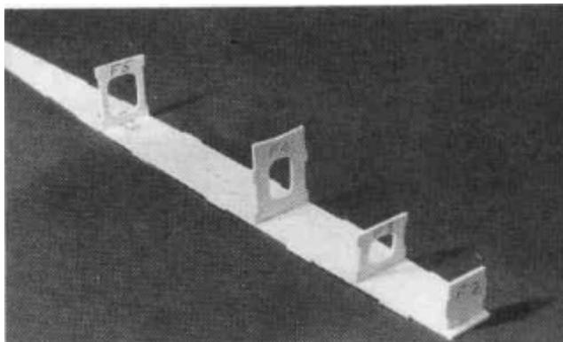
D 2. Trial fit all of the 1/8" **Plywood** Formers (except F1) in the respective notches in the fuselage bottom and sand them if needed to make them fit properly. Use thick CA to "Tack" glue the formers in place. The notches in the fuselage sides will align the formers correctly.
