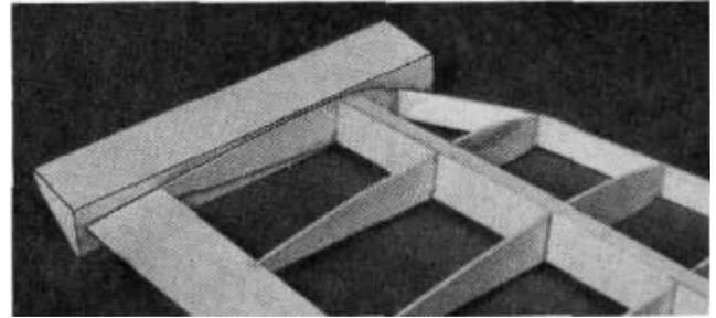
DD 11. Glue the 7/8" x 1-1/4" x 6-1/4" Tapered Wing Tip Blocks (SPRTW15) to W10 with thick CA. The sketch below and the cross sections on the plan shows how the block should be attached to get the correct tip shape.
