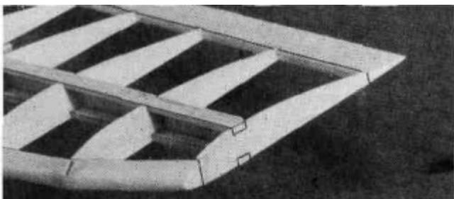
DD 10. Cut and sand the trailing edge, spars and leading edge flush with rib W10. Also cut these to the correct length at the other end using the plans as a guide.
