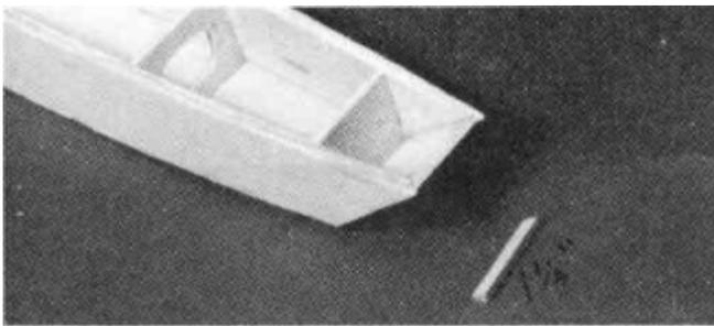
And glue the 1-1/4" long piece along the bottom between formers F1 and F2 to seal the gap there.
