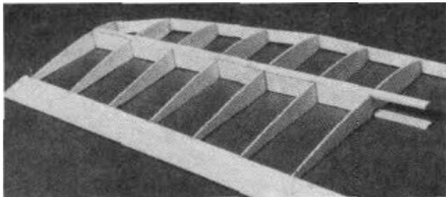
DD 9. Glue the webs into their respective places using thick CA. The thinnest end of each web goes towards the tip of the panel. The C-2 clamps can be used to help hold the webs in place while the glue cures.
