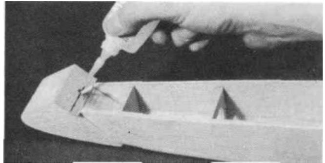
D 11. Insert the 1/8" diameter Canopy Hold Down Dowel (DOWEL033) into the hole and slide the canopy into place to make sure it fits nicely. The dowel should hold the canopy down against the fuselage. If it is too loose you can either enlarge the hole slightly and move the dowel down or you can build up the top surface of the canopy base with thin plywood and/or thick CA. Glue the dowel in place with at least 1/4" extending.
