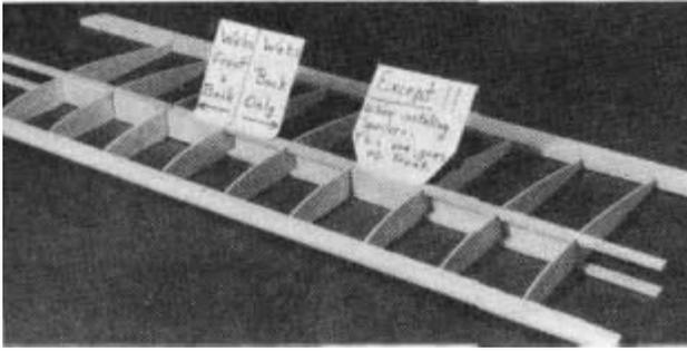
in the first three rib "bays". NOTE: if you are installing spoilers in the wing or may add them in the future, install the web between the two W2S ribs on the FRONT of the spars to make room for the spoiler horn.
