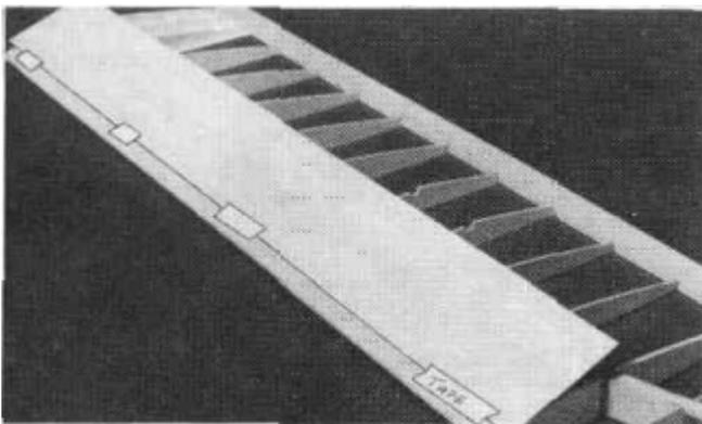
D 15. Set the 1/16" x 3" x 24" **Balsa Leading Edge Sheeting** (SPRTW17) in place on the inner panel. The outer end of the sheeting should cover rib W3A. Cut off the excess sheeting even with rib W1A. Sand the top L.E. of the ribs if necessary to allow the sheeting to be flush with the L.E.
