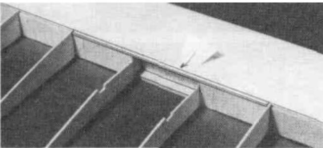
D 20. Glue the 1/16" x 1/8" x 6-9/32" piece of balsa to the back edge of the sheeting between the W2 ribs as shown on the plans and in the photo.
