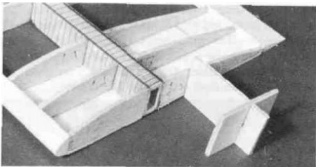
DD 21. Punch out three W1A ribs and three W1B ribs from the 1/8" die-cut balsa rib sheet (SPRTW01). Test fit these ribs into position. A little sanding may be necessary to make them fit properly. Glue these ribs into place using thick CA. The end rib should be tilted in at the top using the slanted end of the rib gauge to give it the correct angle.
