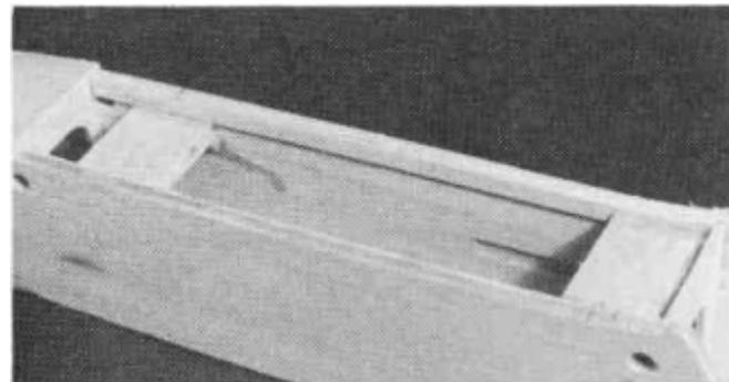
D 12. Cut two pieces of 1/4" birch plywood (not included) which will be drilled and tapped for the wing bolts. The front piece should be approximately 2-1/32" x 1" and the rear piece should be approximately 2" x 1". You will want to measure your fuselage to make the parts fit properly. You should cut the wing saddle tripler away so the blocks can glue directly to the fuselage doubler. Securely glue these in place with thick CA or epoxy. Glue triangle stock around each one for extra strength.
