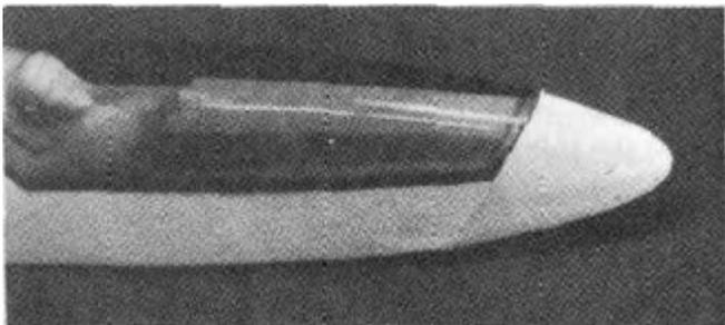
D 14. Use your sanding block with medium and then fine grit sandpaper to smooth out the nose block and fair it in with the canopy and the fuselage.
