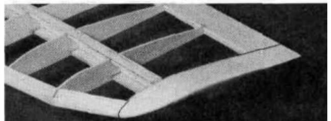
DD 12. Carve and sand the wing tip to blend in with rib W10. Be careful not to change the shape of W10 while sanding the tip. There are three section views on the left wing plan to show you the desired shape.
