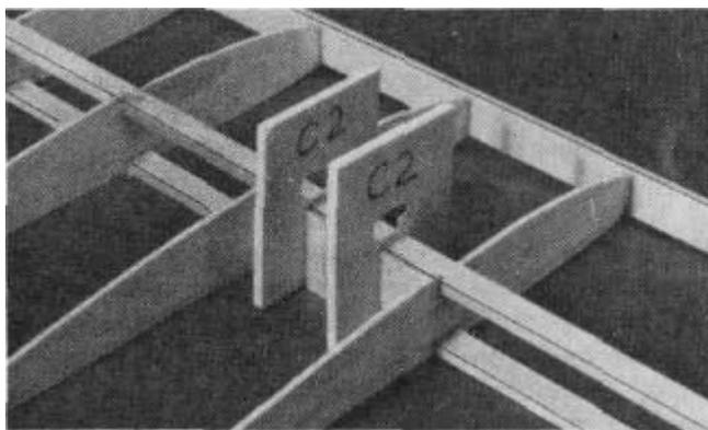
DD 13. Trial fit one of the webs in place between the first two W-2 ribs. You may have to sand it slightly to get it to fit. Glue the shear web in place on the back of the spars using thick CA. The webs should be centered (up and down) between the spars. It is important to do a good job of gluing these in place as they are responsible for most of the wing's strength. C-2 Clamps from the 1/8" Die-Cut Plywood Sheet SPRTW08 can be used to help hold the webs in place while the glue cures.
