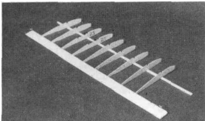
DD 9. Make sure the ribs are properly positioned according to the plans and glue them in place using thick CA at the spar joint and a drop of thin CA at the trailing edge joint. Use the square end of the rib gauge to keep the ribs perpendicular to the work surface. **NOTE: if you are installing spoilers, cut out the embossed area on the two W2S ribs and make sure you install these ribs in the proper locations.**
