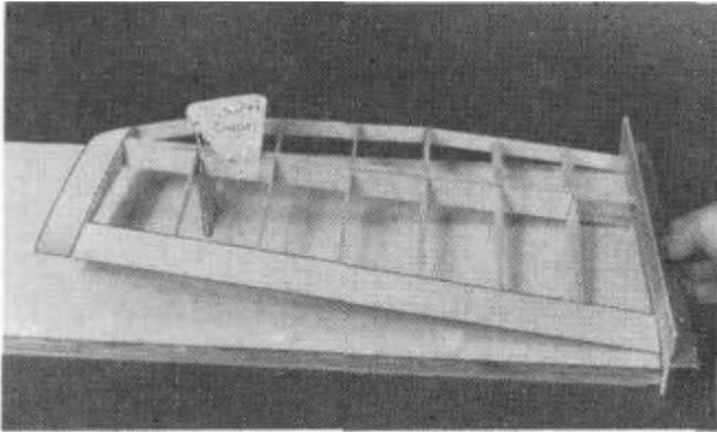
DD 1. Prop up the **outer panel** 2-5/8" (from the work surface to the bottom of W10) using the **lower** notch of the **Dihedral Gauge** (from SPRTW08) next to rib W9. Use a sanding block to carefully sand the leading edge, spars and trailing edge to achieve vertical surfaces on each. Check your progress by occasionally setting the panel on the plans to make sure you are not sanding any "sweep" (forward or backward tilt) into the wing.
