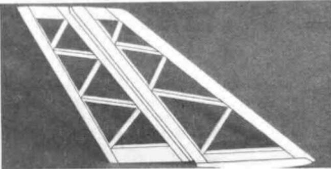
**FIN must remain square, do not sand it!** Sand the triangle stock to blend with the leading and trailing edges of the fin. Also, cut or sand the bottom of the triangle stock to match the contour of the 3/16" die-cut fin bottom.
