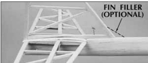
❑ 4. If you're building the straight-tail, trim the bottom of the fin to fit the fuse and stab mount. Glue the fin in position. Make the small fin filler from leftover 1/8" balsa. Glue the **fin filler** to the front of the fin and the fuse top. Blend to the fin by sanding.
