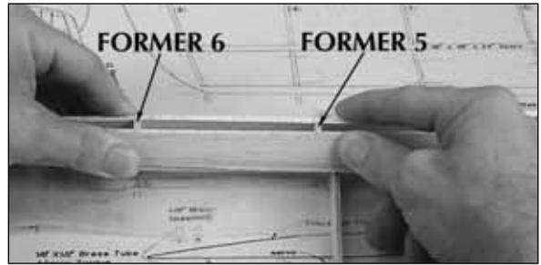
❑ 13. Temporarily hold the upper fuse sides to formers 2 and 3 with T-pins. Pull the aft end of the upper fuse sides to formers 5 and 6 and check alignment. Adjust the position of the upper fuse sides on formers 2 and 3 until they align near the aft end when you pull them to formers 5 and 6.
