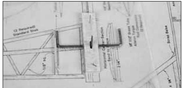
8. Return to step 2 and build the other stab half the same way. When you position the edge of the stab mount/joiner wire 1/16" from the end of the stab, you'll have to turn it around so you get the correct spacing for the **other side** of the joiner.
