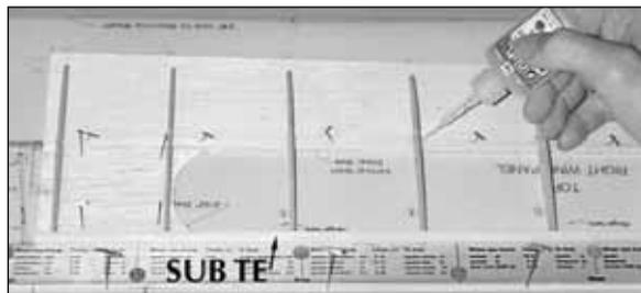
12. One at a time, glue ribs 3 through 9 to the sub trailing edge and the bottom spar. As you proceed, make **certain** the sub TE and the ribs are contacting your building board.
