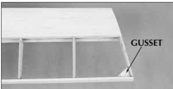
*(For clarity, the wing panel is not shown on the building board in this photo, but yours should still be pinned down).*
