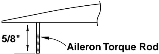
❑ 1. Cut both aileron torque rods to a length of 5/8".
