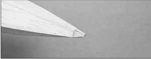
❑ 11. Cut the front of the fuse until the 1/2" x 1/2" x 1/2" hardwood **nose block** will fit. Glue the nose block to the fuse, then carve and sand it to the shape shown on the plan. Note that the grain direction of the nose block runs **parallel** with the length of the fuse.
