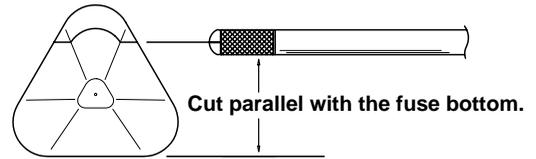
❑ 3. Use a fresh #11 blade to cut the bottom of the hatch along the lines you marked on both sides of the fuselage. Note how the knife in the photo is inserted at an angle, allowing the tip of the blade to trail behind. This provides more stability, allowing **you** to steer the blade, **not** the wood grain. Also note that the cut should be parallel with the **bottom** of the fuse.
