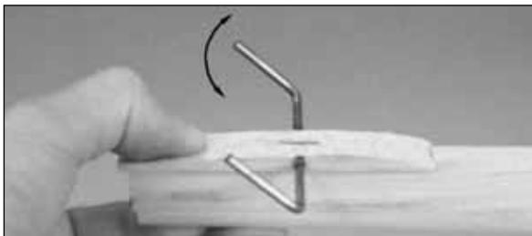
8. Connect the clevis to the bottom hole on the joiner wire. Slip the cable through the elevator pushrod guide tube in the fuse and position **but do not glue** the stab mount on the fuse as shown in the photo and on the plan. Move the cable back and forth to actuate the joiner wire. Make adjustments as necessary so the system operates smoothly.
