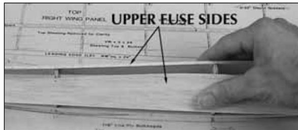
❑ 16. Pull the upper fuse sides to each other and to the fuse bottom. Use medium CA to glue the upper fuse sides to the fuse bottom and to former 1. Refrain from gluing the fuse to the balsa block. But, if you do, it's no problem because you can just break the balsa block free and sand later.
