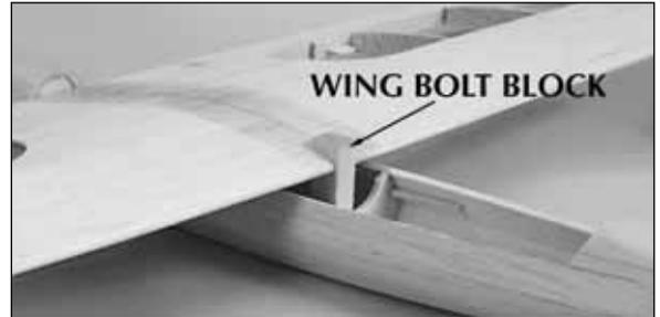
❑ 7. Similar to the way you did the trailing edge of the wing, notch the leading edge of the wing to accommodate the 3/8" x 1/2" x 1-3/4" **wing bolt block** when it is in position against the aft edge of former 2. Test fit the wing with the wing bolt block.
