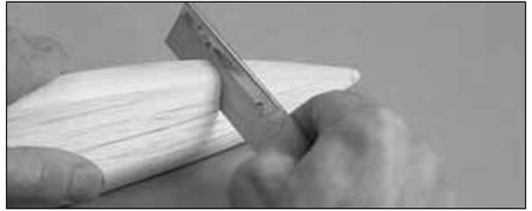
❑ 2. Use a razor saw to cut the aft end of the hatch along the lines you previously marked. Cut the front of the hatch at an angle 11" from the aft end of the hatch.
