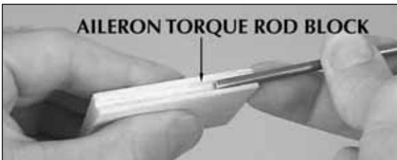
□ □ 6. Cut 2-1/2" from one of the ailerons you shaped earlier to make an **aileron torque rod block**. Cut a 5/32" groove through the center of the leading edge of the block to accommodate the nylon **bearing tube** on the **right aileron torque rod**. **Hint:** Use a 5/32" brass tube sharpened at one end to cut the groove.
