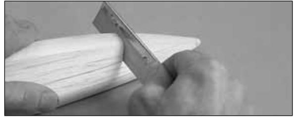
❑ 2. Use a razor saw to cut the aft end of the hatch along the lines you previously marked. Cut the front of the hatch at an angle 11" from the aft end of the hatch.
