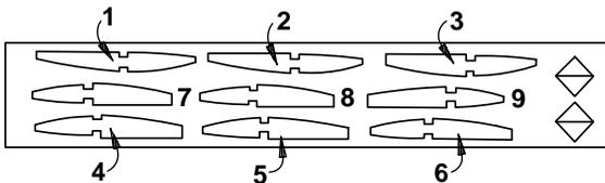
8. Label both sets of die-cut 3/32" **wing ribs** as shown in the sketch and carefully remove them from their die sheets. If any of the ribs are difficult to remove, cut around them first. Remove any die-cutting irregularities or slivers with a hobby knife or sandpaper.
