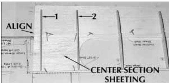
10. Cut the bottom **center section sheeting** from a 1/16" x 3" x 24" balsa sheet (if you're building your second wing panel—the left one—use the remainder of the same 1/16" x 3" x 24" piece you used when you built the right wing panel). Accurately align the edge of the sheet with the end of the wing where shown on the plan and pin it in position. Place ribs 1 & 2 over the sheeting where shown on the plan.
