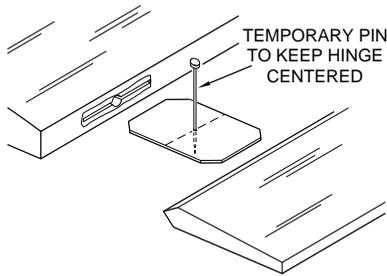
2. Join the aileron to the wing with the hinges. If you cannot get the hinges to remain centered, stick a pin through the center of the hinges and rejoin the aileron to the wing. Remove the pins after you join the aileron to the wing.
