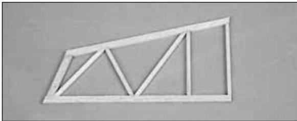
4. Remove the stab mount/joiner wire assembly from the plan and finish building the stab using the remainder of the 1/8" x 1/4" x 24" balsa stick and an 1/8" x 1/8" x 24" balsa stick.
