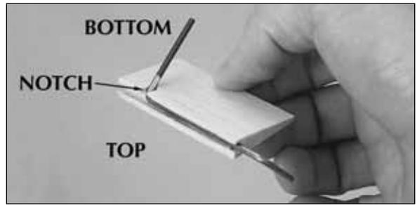
□ □ 7. Test fit the pre-bent wire **right aileron torque rod** (or the **left aileron torque rod** if this is your second time through and you are building the **left** wing panel) in the torque rod block. If necessary, enlarge the groove you cut so the torque rod will fit all the way in. Cut a notch in the **bottom** of the torque rod block to allow for control throw.
