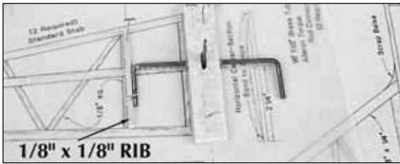
3. Note the location of the **arm** portion of the joiner wire. This determines the **true** location of the 1/8" x 1/8" balsa **rib**—not necessarily where it is shown on the plan. (You can see in the photo how the rib on our model needed to be moved inward a bit). Cut the rib from a 1/8" x 1/8" x 24" balsa stick and pin it to the plan so it is contacting the arm of the joiner wire.
