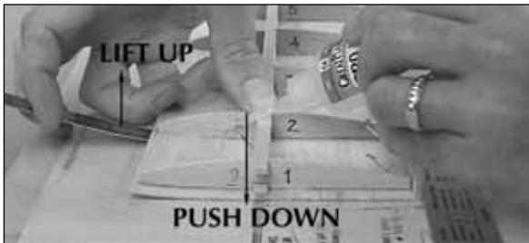
☐☐ 16. One rib at a time, simultaneously **lift up** on the bottom LE skin at each rib as you **push down** on the rib. Add a few drops of thin CA to glue the skin to the rib. **Hint:** Use a thin metal ruler or something similar as a *pry bar* to lift the skin to the rib.
