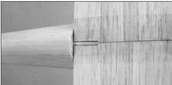
❑ 4. Fit the wing to the fuselage using the dowel. Make adjustments where necessary for a good fit.
