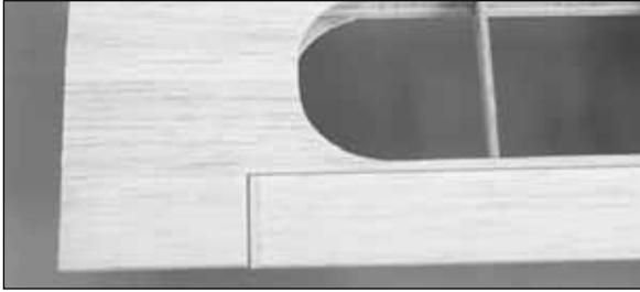
11. Cut a groove and drill a 7/64" (or 3/32") hole in the leading edge of the aileron to accommodate the aileron torque rod. Test fit the aileron to the wing.
