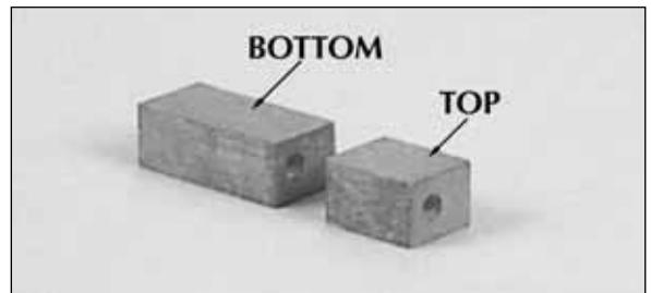
❑ 9. Cut 11/16" from the top of the wing bolt block. You now have a **bottom** and a **top** wing bolt block.
