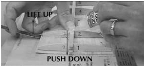
☐☐ 16. One rib at a time, simultaneously **lift up** on the bottom LE skin at each rib as you **push down** on the rib. Add a few drops of thin CA to glue the skin to the rib. **Hint:** Use a thin metal ruler or something similar as a *pry bar* to lift the skin to the rib.
