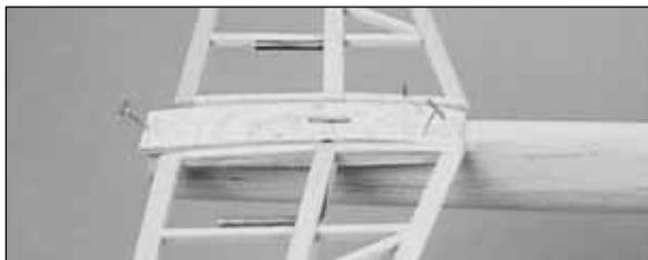
❑ 2. After you have achieved the alignment described above, connect the elevator cable to the elevator joiner wire. Route the cable through the guide tube and securely glue the stab mount to the fuse with 30-minute epoxy. Hold the stab mount in position with T-pins until the epoxy is fully cured.
