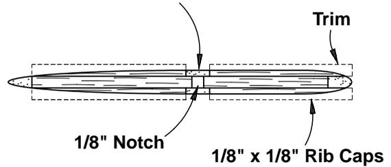
7. Glue an additional 1/16" x 1/4" balsa stab spar to the other side of the stab the same as the first. Use the remainder of your 1/8" x 1/8" x 24" balsa stick to make the **rib caps** that fit on the front and back of the stab spars on the top and bottom of the stab. Blend the rib caps and the tip of both stab spars to the stab by sanding.
