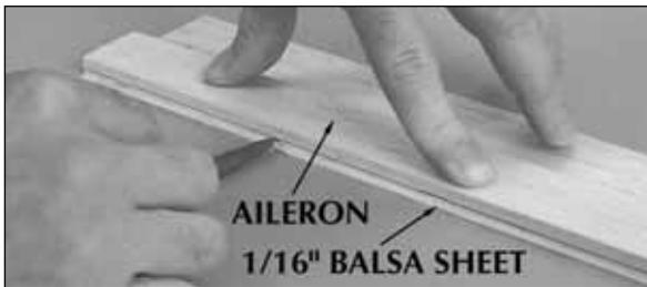
1. Use a ballpoint pen to draw a **guideline**  $3/32$ " from the bottom of one of the  $5/16$ " x  $1-1/4$ " x  $24$ " balsa **ailerons**. This guideline indicates the
