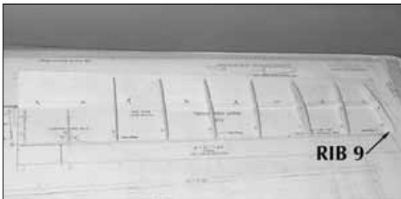
9. Place ribs 3 through 9 on the bottom spar. If necessary, trim the notch in rib 9 so it will fit the bottom spar at the angle on the plan.
