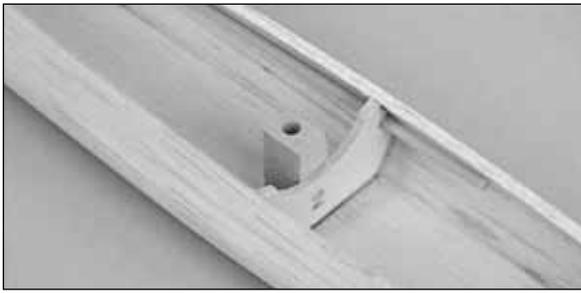
❑ 10. Securely glue the bottom wing bolt block to the aft edge of former 2 and the bottom of the fuse. Enlarge the hole in the bottom wing bolt block and drill through the bottom of the fuse with a #12 (or 3/16") drill bit.
