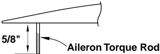
❑ 1. Cut both aileron torque rods to a length of 5/8".
