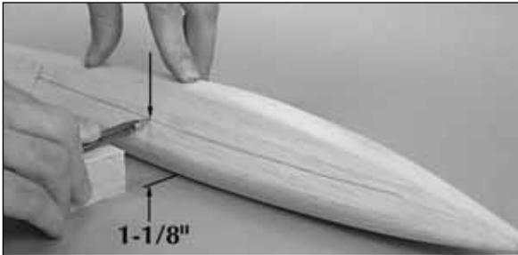
❑ 1. Use a balsa block or something similar to support a ballpoint pen so the tip will be 1-1/8" above your building table. Mark the bottom of the hatch on both sides of the fuse extending from the lines you marked earlier 11" forward. As you proceed, press down on the fuselage over the area where the bottom is flat as shown in the photo.
