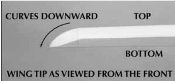
□ □ 5. Glue a shaped triangular balsa **wing tip block** to the end of the wing. Note that the flat side of the tip block is on the bottom of the wing so the tip curves **downward**. Carve, then sand the wing tip block to match the shape of the wing and the plan.
