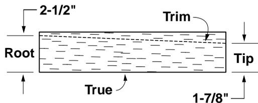
5. Use a fresh #11 blade and a straightedge to true one edge of a  $1/16$ " x  $3$ " x  $24$ " balsa sheet. Trim the other edge of the sheet as indicated in the sketch. From now on this sheet will be called the **bottom leading edge skin**.
