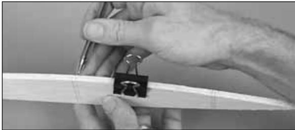
❑ 10. Transfer the lines from the left fuse side to the right fuse side.
