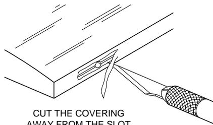
1. Use your hobby knife and a sharp #11 blade to remove a small strip of covering from the hinge slots of one of the ailerons and the matching half of the wing.
