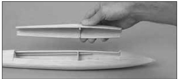
❑ 4. Use a fine razor saw to cut former 2 as shown in the cross section on the plan so you can remove the hatch. *Neato!*
