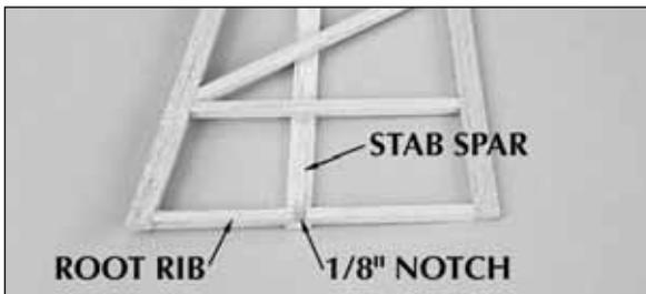
6. Cut a **stab spar** from the 1/16" x 1/4" x 36" balsa stick, then glue it to one side of the stab where shown on the plan. Turn the stab half over and cut an 1/8" notch in the 1/8" x 1/8" **root rib** to accommodate the elevator joiner wire.
