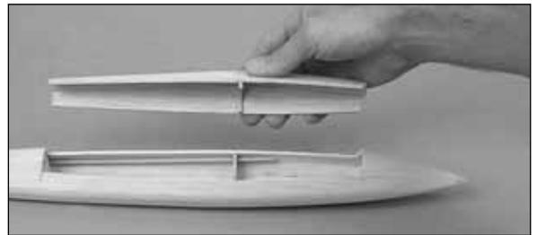
❑ 4. Use a fine razor saw to cut former 2 as shown in the cross section on the plan so you can remove the hatch. *Neato!*
