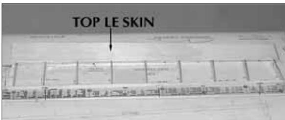
☐☐ 18. Reposition any T-pins in the bottom spar that will be concealed when you position the top leading edge skin and the top center section sheeting. Apply a bead of medium or thick CA **to the top spar only** and glue the top leading edge skin in position.
