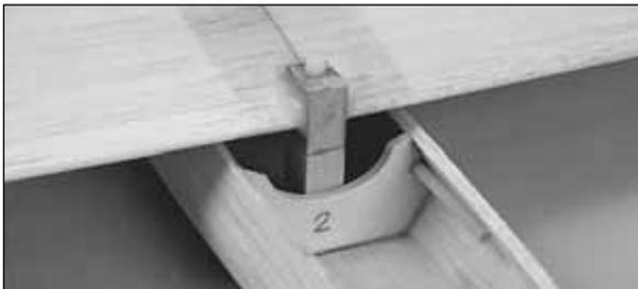
❑ 12. Secure the top wing bolt block to the bottom wing bolt block with the 10-32 x 2" nylon **wing bolt**. Position the wing on the fuselage with the top wing bolt block in the notch in the leading edge.
