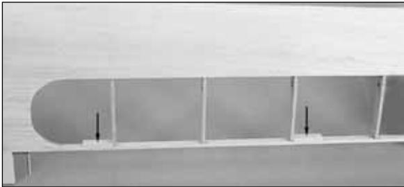
12. Cut three 1/8" x 5/16" x 1" **hinge blocks** from leftover 1/8" balsa and glue them to the front of the sub trailing edge where the hinges are shown on the plan. The hinge blocks are not shown on the plan but you can see two of them in the photo.
