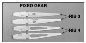
□ 1b. If you will be installing fixed gear, glue the four diecut 1/8" ply rib doublers with one slot to the pair of die-cut 3/32" balsa **ribs 3 and 4**, being careful to make a left and right rib 3 and 4. **Note:** Make sure the slot in the doubler going on rib 3 is in the same direction of the servo tray slot in rib 3.
