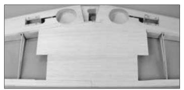
■ 8. Use two 1/16" x 3" x 30" balsa sheets to sheet the bottom center section of the wing. **Note:** Using a straightedge aligned with the LE sheeting makes cutting the forward piece of center sheeting easy.
