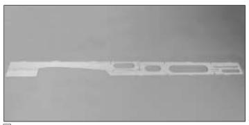
■ 8. Cover the fuse side view of the plans with Great Planes Plan Protector. Fit and glue the die-cut 1/8" balsa **forward, center and fuse sides** together over the plan as shown in the photo.
