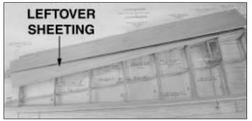
$\Box$  23. Being careful not to cut into the spar, use a straightedge as a guide and cut the sheeting along the center of the spar.
