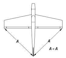
□ 3. Stick a T-pin through the center of the aft end of the fuselage bottom. Tie a string to the T-pin. Pull the string to the TE of the wing tip and put a piece of masking tape on
