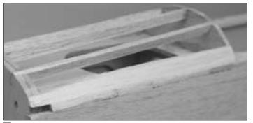
4. Round the side stringers to match the firewall and the instrument panel.
