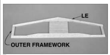
$\Box$  5. From a 3/16" x 1/2" x 24" balsa stick, cut, fit and glue the stab LE and remaining outer framework.
