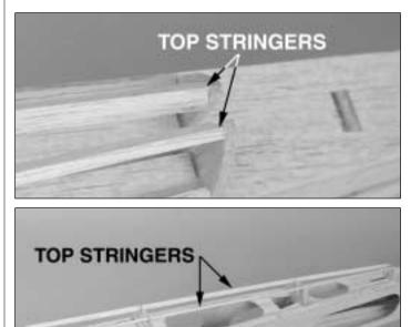
□ 10. Fit the two 1/8" x 1/4" x 24" balsa **turtle deck top stringers** in the slots in F3B, F4B and F5B. Glue the aft end to the front edge of F6B as shown. Glue the stringers to F3B, F4B and F5B. Trim the front end flush with the front of former F3B.
