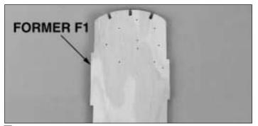
□ 1. Place one die-cut 1/8" ply former F1 on the work surface with the front (punch marked) side facing up. Epoxy the second F-1 to the first with 6-minute epoxy, again with the punch marked side facing up. Make sure the edges all the way around are aligned. Wipe away any excess epoxy before it cures. Note: If the firewall formers are warped, simply clamping them together may not "cancel out" the warps. It is best to clamp the formers to a table or a flat board until the epoxy cures.
