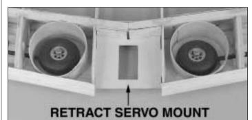
□ 4. Fit the wing panels to the wing joiner and the die-cut 1/8" ply **retract servo tray. Note:** The retract servo tray will be installed whether you are using retracts or fixed landing gear.
