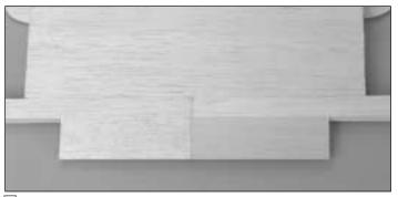
□ 21. Glue the two 4" pieces to the inboard TE of each wing panel, with the inboard ends aligned at the centerline of the wing.
