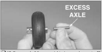
□ 18. If you are building your right wing panel, mount a 2" wheel (GPMQ4221) to each of the two adjustable axles
