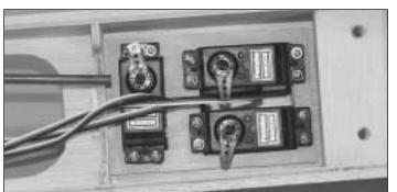
□ 3. Mount the throttle, elevator and rudder servos, using the hardware supplied with the radio.
