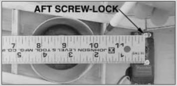
$\Box$  6. On the right wing half, mark on the wheel well and rib 2A where a line from the **aft** screw-lock to the control link on the right retract intersects the wheel well and rib 2A.
