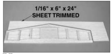
□ □ 9. Glue the stab framework to the sheeting, aligning the TE and the left outer edge of the framework with the edges of the sheeting. Trim the sheeting around the stab framework. **NOTE:** It is important to glue the sheeting securely to the stab center.
