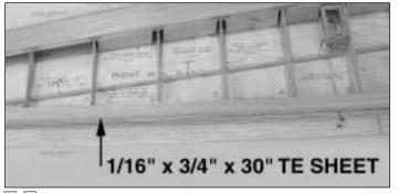
□ □ 26. Sand the TE so that it is flush with the ribs. Glue a TE sheet to the TE and the ribs, aligning it along the TE of the 3/8" TE stick.
