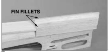
$\Box$  21. Cut the 3/4" x 1-1/4" x 15" balsa stick in half, making two 7-1/2" **fin fillets**. Tack glue these fillets to the fuse top and the fin filler block.
