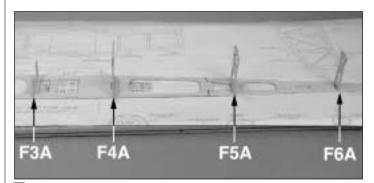
□ 14. Glue the die-cut 1/8" ply formers **F3A, F4A, F5A** and **F6A** vertically in the **rear** of the slots in the fuse top.
