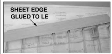
$\Box$  22. Edge glue a 1/16" x 3" x 30" balsa sheet to the shaped LE, letting it contact the front edge of each rib.
