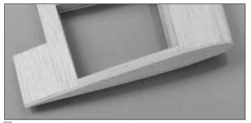
□ 23. Cap both wing tips with leftover 1/16" balsa sheet. Sand to the shape of the wing.
