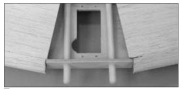
□ 16. Trim the ends of the shaped LE so the forward dowel support will fit flush against the inboard ends of the LE and tight against the retract servo tray.
