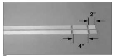
□ 20. From one piece of 30" tapered balsa aileron stock, cut a 4" and a 2" length. Cut 4" and 2" lengths from the other 30" aileron stock.
