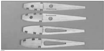
□ 2. Trim the balsa ribs as shown, using the openings in the rib doublers as a guide. **Note:** The ribs in the photo are for retracts. If you are using fixed gear, trim your ribs in the same manner but with only one landing gear rail cutout.
