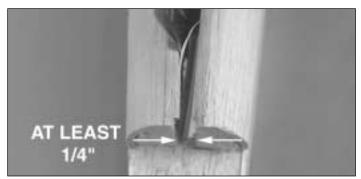
$\Box$  17. Trim the aft end of the 1/8" x 1/4" top stringers so there is at least a 1/4" gap between them, allowing sufficient space for the fin.
