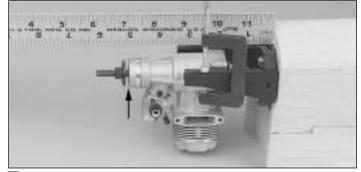
□ 4. Position the engine on the mount so the drive washer (or the back of the spinner) is 5" away from the firewall and clamp in place.
