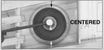
□ □ 19. Mount the axle on the end of the strut, centering the wheel between the ribs. Bend the strut forward or aft as required to center the wheel between the LE and the spar.
