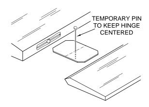
□ 3. Without using any glue, fit the hinges in the elevators or stab. **Do not glue the hinges yet.** As you join the elevators to the stab, confirm that the hinges are equally inserted in the elevators and the stab. Insert a small pin in the center of the hinges to keep them centered.
