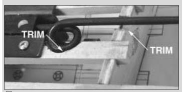
☐ 17. Remove the area of the rear landing gear rail that makes contact with the coil of the retract. Do the same where the strut makes contact with rib 3. **Hint:** Your rotary tool works well for both these tasks. Just be careful not to accidentally over trim.
