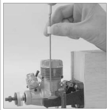
□ 5. Use the **Great Planes Dead Center**<sup>™</sup> **Engine Mount Hole Locator** (GPMR8130) to mark the locations of the bolt holes. Remove the engine from the mount and drill four 7/64" holes. Tap the four holes with a 6-32 tap. Mount the engine with the four 6-32 x 1" socket head bolts.
