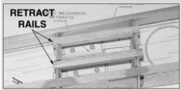
□ □ 14. Epoxy the two 1/4" x 3/8" x 4" basswood **retract rails** to ribs 3 and 4.
