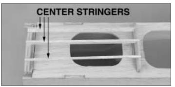
$\Box$  2. From a 1/8" x 1/4" x 24" balsa stick, cut, fit and glue the three **front deck center stringers** into the firewall and IP.
