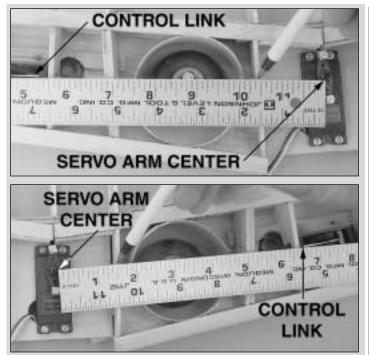
□ 5. Use a straightedge to mark a line from the **center of the servo arm** to the **control link** on the right retract on the right wheel well and rib 2A. Repeat for the left retract.
