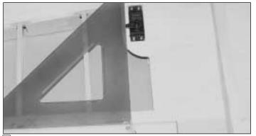
$\Box$  20. Locate the control horn on the aileron using a square so that the pushrod will be perpendicular to the hinge line. Mount the control horn and back plate with the 2-56 x 5/8" screws.
