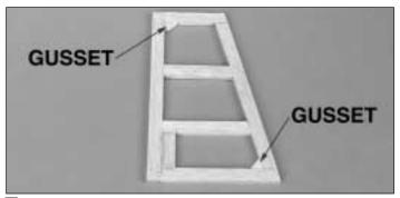
□ 4. Using a 1/4" x 1/2" x 24" balsa stick, cut, fit and glue the rudder framework and ribs. It may be necessary to use the leftover 1/4" x 1/2" balsa from the fin. Don't forget the control horn support and the corner gussets.
