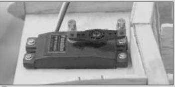
□ 2. Find a servo horn with the outer holes at 1-1/16" to 1-1/8" from each other. Mount a **Screw-Lock Pushrod Connector** (GPMQ3870, not included) in both outer holes. **Hint:** The standard S6-arm Futaba servo horn works well — just trim off the 4 arms that are not needed.
