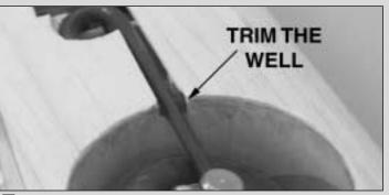
□ 1. Trim the wheel wells where the struts make contact so the retracts can lock in the "up" position.
