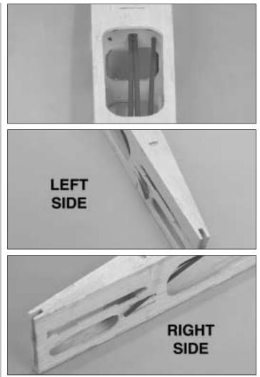
□ 5. Fit the two elevator pushrod tubes in the upper holes in F4A, F5A, F6A and the fuse sides, leaving a small amount of excess extending out the fuse sides. Fit the rudder pushrod similarly into the lower right hole.
