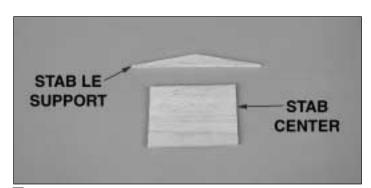
□ 2. Laminate the stab centers and the LE supports together with medium CA, making a 3/16" stab center and a 3/16" LE support.
