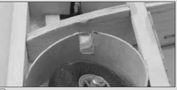
■ 8. Cut 3/8" wide by 5/8" deep slots in the outside edges of both wheel wells centered on the marks you made in steps 5-7.
