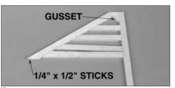
$\Box$  2. Using two 1/4" x 1/2" x 24" balsa sticks, cut, fit and glue the fin framework and ribs. Don't forget the gusset at the top of the fin. **Note:** The fin tail post goes all the way down to the bottom of the fuse.
