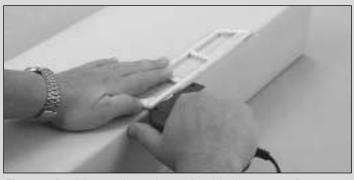
To cut the hinge slot, place the blades onto the wood where you want the slot. Lightly press the teeth into the wood. When you are satisfied with the location, press the button on the handle and the blades will cut easily into the balsa wood. Go to step 3 to complete hinging your stab.
