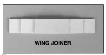
□ 1. Using medium CA, laminate the three die-cut 1/8" ply center spar joiners. This complete assembly is now called the wing joiner.
