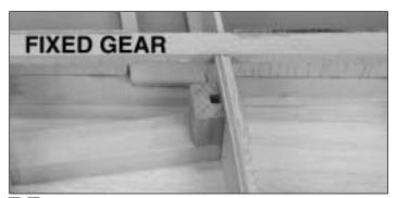
□ □ 38. If you are installing fixed gear, turn your wing rightside-up and epoxy the 7/16" x 5/8" x 3/4" maple grooved **torque block** to the rib 3 doubler and the landing gear rail, with the groove facing the doubler as shown in the photo.
