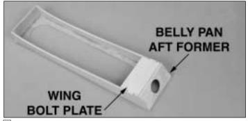
□ 2. Glue the die-cut 1/8" ply **belly pan aft former** and **wing bolt plate** in place as shown in the photo. **NOTE:** The punch marks in the wing bolt plate must be facing down so that they will be visible through the belly pan bottom when the belly pan is upside-down.
