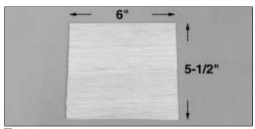
□ 5. From a 3/32" x 2-3/4" x 24" balsa sheet, cut two 6" sheets. Edge glue these two sheets together, making one 3/32" x 5-1/2" x 6" sheet. Set the remaining 12" piece aside.
