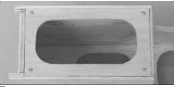
$\Box$  15. Temporarily mount the tank hatch to the fuse with four #2 x 3/8" sheet metal screws.
