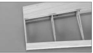
$\hfill \square$  28. Trim the TE sheet, TE, LE, LE sheet and the spars flush with rib 9.
