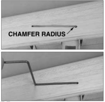
$\Box$  40. Turn the wing upside-down. Using the slot in the landing gear rail as a guide, cut the opening for the gear to fit. Chamfer the torque block opening to allow the radius in the landing gear leg to fit properly in the rail.
