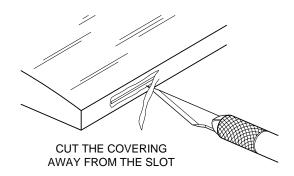
$\Box$  1. Start with the elevators and stab. Cut the covering from the hinge slots – don't just slit the covering but remove a small strip the size of the hinge slot.
