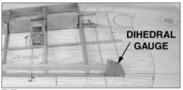
□ □ 13. Use the dihedral gauge to position the  $3/8" \times 3/8" \times 30"$  balsa **TE** at the centerline of the TE of the ribs. Glue the TE to the ribs.
