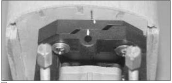
□ 3. Place the engine on the mount and slide the halves in or out until the engine fits properly. Position the mount so the molded-in "tick marks" are equally spaced from the horizontal centerline you drew on the firewall. When the engine mount is adjusted and positioned, tighten the mounting screws.
