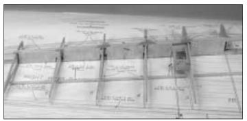
□ □ 9. From a 1/16" x 3" x 24" balsa sheet, cut, fit and glue the five **shear webs** in place. **Note:** You may have to move a T-pin or two to glue the webs in place. Just replace them behind the shear webs after the shear webs are glued in place.
