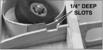
□ 9. Cut a 1/4" deep slot between the marks on both ribs 2A and the inside of both wheel wells.
