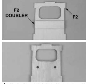
□ 6. Glue the die-cut 1/8" ply **F2 doubler** to the **front** side of die-cut 1/8" ply **F2** as shown on the plans.
