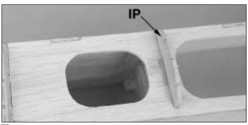
□ 1. Glue the die-cut 1/8" balsa **instrument panel (IP)** vertically to the fuse top.
