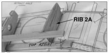
□ □ 7. Using a square to keep it perpendicular to the work surface, glue the die-cut 3/32" balsa **rib 2A** to the spars.
