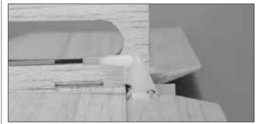
□ 8. Insert both elevator pushrods into the upper pushrod tubes. Position the control horns on the elevators as shown
