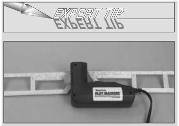
We have simplified the task of cutting hinge slots with the introduction of the **Great Planes Slot Machine**<sup>™</sup>. This simple electric tool cuts a perfect width slot for use with CA hinges.
