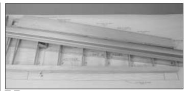
□ □ 4. Lift the LE sheeting away from the ribs and put thick CA on the ribs and the front half of the spar. Roll the sheeting down and weight it in place until the glue has dried.
