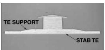
$\Box$  4. Using two 3/16" x 1/2" x 24" balsa sticks, cut, fit and glue the stab TE support and stab TE in place. **NOTE:** Be sure to cut the angle on the ends of the TE support as shown on the plans.
