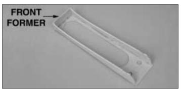
□ 1. Glue the die-cut 1/8" ply belly pan sides and belly pan front former perpendicular to the belly pan bottom.
