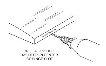
□ 2. Drill a 3/32" hole 1/2" deep in the center of each hinge slot. A high speed Moto-Tool works best for this. If you use a regular drill, clean out the hinge slots with your #11 blade.
