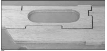
■ 9. Cover the first fuse side with Great Planes Plan Protector and fit and glue the second side together over the first, making two identical fuse sides.
