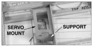
□ □ 8. Glue the die-cut 1/8" ply **servo mount** and the diecut 1/8" ply **servo mount support** in place.
