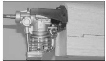
**Note:** If you are using a larger engine than the .46 it may be necessary to sand the left fuse side flush with the firewall, so that the mount fits.
