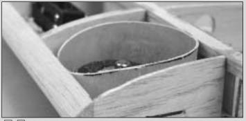
□ 35. Double-check the shaping of the well by looking at it from the inboard end of the wing. When satisfied with the fit, glue it to the sheeting, centering it between ribs 3 and 4. **Note:** Leaving the can in the well will help the well hold its shape as it is being glued.
