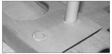
□ 12. Repeat steps 10 and 11 to mount the paper tube over the other wing bolt. Sand the paper tubes flush with the belly pan bottom.
