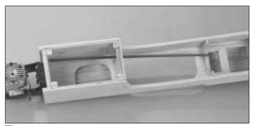
□ 2. Select one of the remaining grey outer pushrod tubes. Use coarse sandpaper to roughen the outside of the tube so glue will stick. Slide it through its hole in the firewall, until it protrudes 1/8" past F3A. Glue it into the firewall. Cut the pushrod outer tube 1/4" in front of the firewall.
