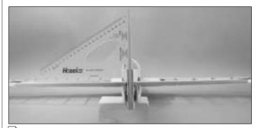
□ 5. Fit the fin in place and check that it is perpendicular to the stab with a square. If it is not perpendicular, small adjustments can be made by sanding a taper on the fin post,
