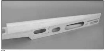
□ 22. Shape the turtle deck top to the round shape of the turtle deck, using the cross sections as a reference. Do the same for the fin fillets and the fin filler block, blending everything smoothly. **Hint:** Start your shaping with a razor plane, then use a course sand paper (around 100 grit), then gradually work with finer paper until you are using 400 grit to get a really nice final shape that's cleanly sanded.
