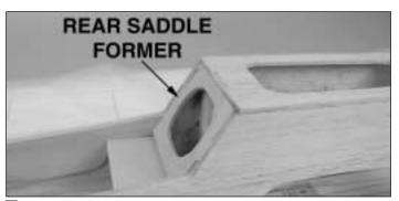
□ 20. Sand a taper on the bottom edge of the die-cut 1/8" ply **rear saddle former**. Fit it in place, adjusting the taper until a good fit is achieved. Glue the former in place.
