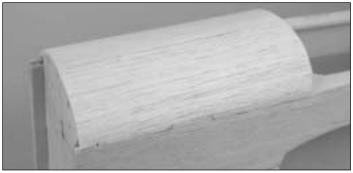
□ 7. Shape the sides of the sheeting so it blends with the fuse side. Sand the front edge flush with the firewall. Sand the TE flush with the instrument panel.
