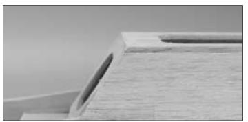
□ 21. Sand the front of the aft fuse bottom to the angle of the rear wing saddle former.
