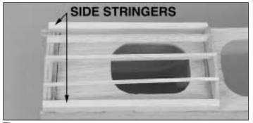
$\Box$  3. From a 1/4" x 3/8" x 18" balsa stick, cut, fit and glue the two **front deck side stringers**.
