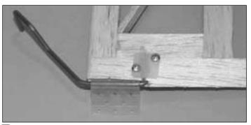
□ 15. Mount the control horn to the rudder, trapping the tail gear wire between the screws.
