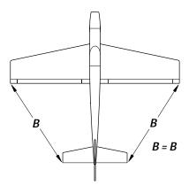
□ 2. Mount the wing to the fuselage. Center the stab in the stab slot. Use a string from the center of the firewall to align the stab the same as was done with the wing.
