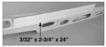
$\Box$  11. Edge glue a 3/32" x 2-3/4" x 24" balsa sheet to the fuse top, with the forward edge extending beyond F3B and the aft edge extending past F6B.
