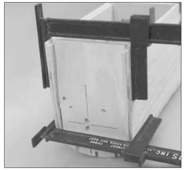
$\Box$  2. Fit the firewall tabs into the slots in the fuse sides. When satisfied that the firewall can be put in place easily, epoxy it in place. **Hint:** Note the right thrust built into the firewall installation.
