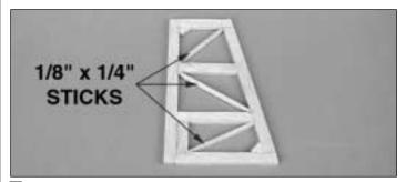
$\Box$  5. From a 1/8" x 1/4" x 12" balsa stick, cut, fit and glue the three cross braces in place.
