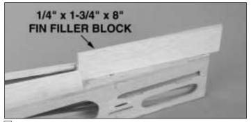
□ 18. From a 1/4" x 1-3/4" x 36" balsa stick, cut one 8" fin filler block. Tack glue the fin filler block where the fin will be located, aligning the TE of F6B and centered on the slot in the middle of F6B.
