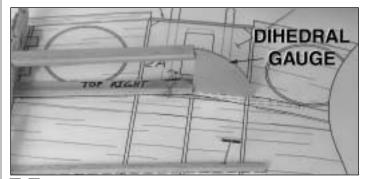
□ □ 6. Use the die-cut 1/8" ply **dihedral gauge** to locate the inboard end of the bottom spar, then position the bottom spar in the ribs. Being careful not to twist the ribs, glue the bottom spar in place.
