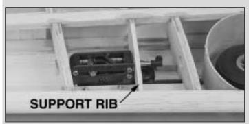
□ □ 37. Epoxy the die-cut 1/8" ply retract support rib in place.
