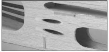
□ 11. After the epoxy has cured, use a bar sander and 150-grit sandpaper to sand the outer pushrod tubes and filler flush with the fuselage sides.
