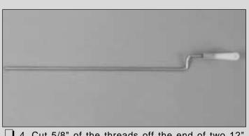
□ 4. Cut 5/8" of the threads off the end of two 12" pushrods with clevises attached (GPMQ3772, not included). Bend to the shape as shown on the plans.
