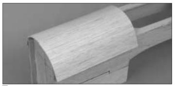
$\Box$  6. Wet the outside of the 5-1/2" x 6" sheet with water or a water/ammonia mix. Glue it to the firewall, instrument panel and stringers.
