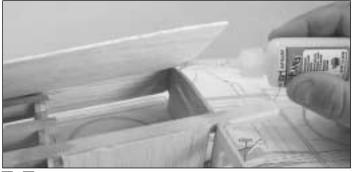
□ □ 24. Being careful to keep the spar against the building surface and the ribs on the wing jig, use medium or thick CA to glue the sheeting to the ribs and the front half of the spar.
