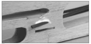
■ 9. Mix the remaining epoxy with microballoons and epoxy the pushrod tubes to the slots in the fuse sides. Completely fill the slots with the microballoons/epoxy mix.
