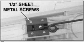
□ 16. Place your retract in place on the rails. Drill four 5/64" pilot holes through the bass rails, using the mounting holes as a guide. Mount the retract with four #4 x 1/2" sheet metal screws (not provided).
