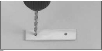
□ 15. Drill two 1/4" holes, at the punch marks, in the diecut 1/8" ply **forward dowel support**.
