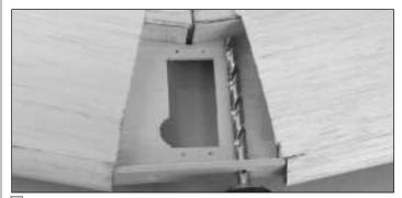
□ 18. Remove the dowels and drill 1/4" holes through the 1/16" balsa shear webs.
