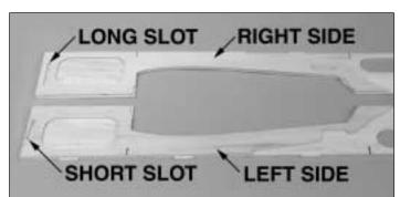
□ 10. Position the fuse sides exactly as shown. Glue the die-cut 1/8" ply left fuselage side doubler (L) to the left fuse side. Glue the die-cut 1/8" ply right fuselage side doubler (R) to the right fuse side. Note: The left fuse side doubler is the one with the short slot and the right side fuse doubler is the one with the long slot.
