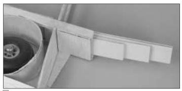
□ 3. Temporarily fit the wing joiner into one wing half. From the remaining piece of 1/16" x 3" balsa used to make the shear webs, make a LE shear web that goes to the inboard end of the spars. Glue the web to the spars. Do the same for the other wing half. **Note:** Do not glue the joiner in yet.
