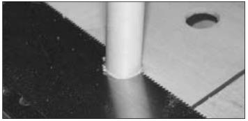
$\Box$  11. Using a razor saw, cut off the paper tube flush with the belly pan bottom.
