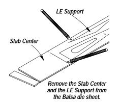
□ 1. Remove the two die-cut 3/32" balsa **stab centers** and the two die-cut 3/32" balsa stab **LE supports** from the die sheet as shown in the sketch.
