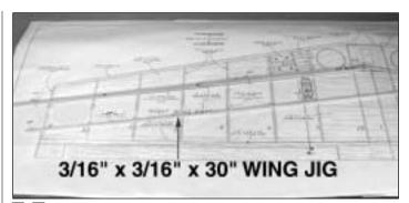
$\Box$  2. Pin a 3/16" x 3/16" x 30" balsa wing jig stick over the wing jig position shown on the plan. Note: Do not pin at the rib positions.
