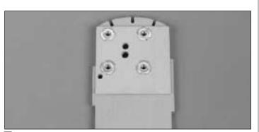
□ 5. Press the four supplied 6-32 blind nuts into the holes on the back of the firewall. Gently tap the blind nuts with a hammer to fully seat them into the firewall, then add a few drops of thin CA around the blind nuts to secure them.
