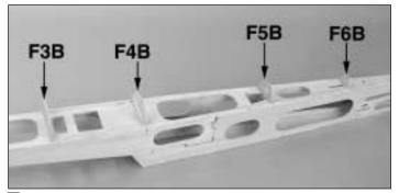
■ 8. Glue the die-cut 1/8" balsa formers **F3B**, **F4B**, **F5B** and **F6B** vertically to the fuse top.
