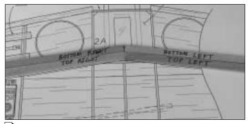
↓ 4. Position 2 spars on top of each other with the spar doublers against one another. Position the other 2 spars similarly. Sand the inboard end of all four spars to match the centerline of the wing, labeling each one as you do so. **Note:** Make sure you make a **bottom left, bottom right, top left and top right spar**. The top spars shown in the photo have been turned upside-down and the label is written on the bottom of the spar doubler.
