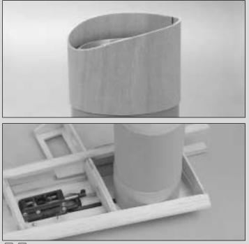
□ □ 33. Shape one end of the wheel well so that when slid in place it makes contact with the sheeting all the way around.
