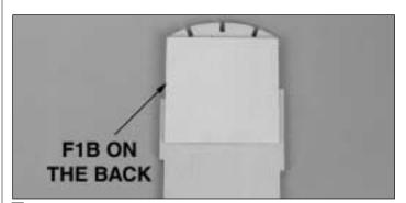
□ 2. Glue the die-cut 1/8" ply **F1B** to the back of the F1 formers with medium CA. From now on this assembly will be referred to as the **firewall**.
