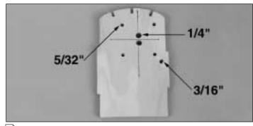
□ 3. Using a straightedge and a pen, draw a line horizontally across the firewall from the left outer punch mark to the right outer punch mark. Draw a line vertically from the top punch mark to the bottom punch mark. The intersection of these two lines is the center of the engine mount. **Note:** The center of the engine mount is offset to compensate for the built-in right and down thrust so that the crankshaft will exit the cowl dead center on the fuselage centerline.
