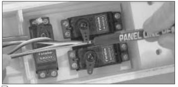
□ 9. With the elevator servo in place, the servo arm perpendicular to the pushrod and the control surfaces in neutral position, use a felt tip pen to mark where one pushrod crosses the mounting holes in the servo arm.
