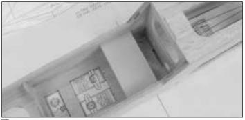
19. Epoxy the bolt block securely in place in the fuse.
