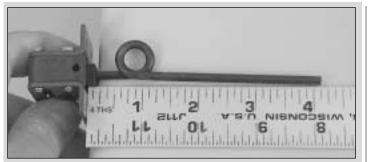
□ 15. Using a rotary tool and a cutoff wheel, cut both retract struts so they are 4-1/8" long, measuring from the mounting plate on the retract body.
