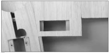
□ 10. Cut openings in the bottom sheeting for the aileron servos.
