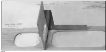
□ 12. Glue former F2 vertically in the **front** of its slot in the fuse top. Be sure the F2 doubler you installed in step 6 is facing forward.
