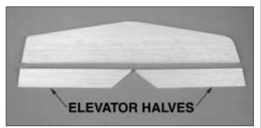
$\Box$  12. From the 1-3/4" x 24" tapered balsa elevator stock, cut two **elevator halves** to the shape shown on the plans.
