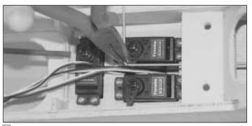
□ 10. Disconnect the clevis from the control horn on the wire you marked. Make a 90-degree bend at the mark you made. Temporarily install a nylon Faslink on this pushrod, then cut the wire so it slightly protrudes out of the Faslink. **Hint:** If you prefer to bend and cut the pushrod outside the fuselage, remove the pushrod, then make the 90-degree bends and cut the wire. Unscrew the clevis and reinstall the pushrod in the guide tube from the front, then screw the clevis back on.
