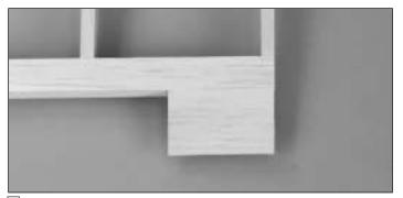
□ 22. Glue the 2" pieces to each wing tip, aligning them with the outboard edge.
