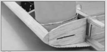
□ □ 34. While holding the well in place, mark a cut line around it so that the top sheeting will just touch the well when it is glued in place. Remove the well from the can and cut around the line.
