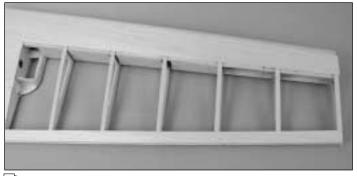
$\Box$  12. Using the 1/16" x 1/4" x 30" balsa sticks, cut, fit and glue **cap strips** to all of the exposed ribs, both top and bottom.
