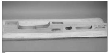
$\Box$  15. Fit the fuse sides and die-cut 1/8" balsa **fuse bottom** in place.
