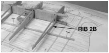
□ □ 10. Position the die-cut 3/32" balsa rib **2B** perpendicular to the work surface and glue it to the spars.
