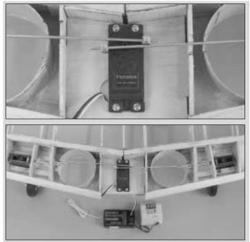
□ 11. Hook up the pushrods with the gear in the "down" position and the arm as shown. Pull the pushrods until the gear locks down, then tighten the set screws on the screw-lock connectors.
