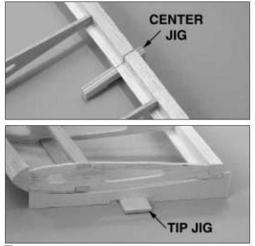
□ 5. Position the wing on the jigs. When satisfied that the wing is joining properly, lift it off the work surface and liberally coat the wing joiner and spars with epoxy and position in place. Place the wing back on the jigs and glue the retract servo tray in and the TEs of the wing panels together with thin CA. Weight the wing and leave it undisturbed until the epoxy has fully cured.
