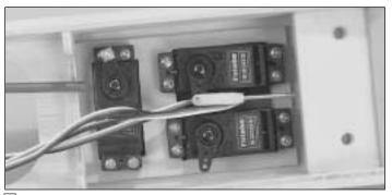
☐ 11. Connect the bent pushrod to the servo with the Faslink. If necessary, enlarge the hole in the servo arm with a 5/64" drill bit (or a #48 bit for precision). Cut the second pushrod 1/8" behind the Faslink (being sure the elevator half is neutral).
