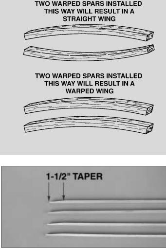
$\Box$  2. Sand a 1-1/2" taper on one end of each spar doubler as shown.
