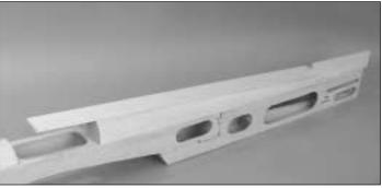
□ 19. Glue the remaining 1/4" x 1-3/4" x 28" balsa turtle deck top to the top of the turtle deck sheeting and the tops of the formers. Note: Do not glue it to the fin filler block.
