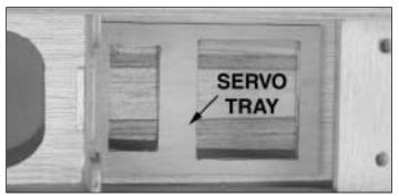
1. Glue the die-cut 1/8" ply servo tray in place in the fuse.
