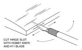
□ 2. Cut the hinge slots in the elevator and stabilizer using a #11 blade. Begin by **carefully** cutting a very shallow slit at
