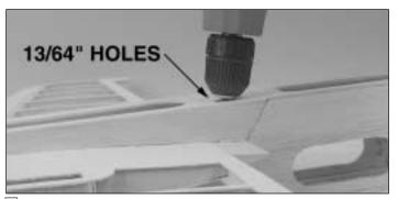
□ 6. Position the wing back on the fuse after all CA is fully cured. Holding the wing firmly in place on the fuse and using the punch marks in the wing bolt plate as a guide, drill two 13/64" holes through the wing bolt plates, the wing and the bolt block (in the fuselage), keeping the drill perpendicular to the wing bolt plates and centered in the holes in the belly pan bottom.
