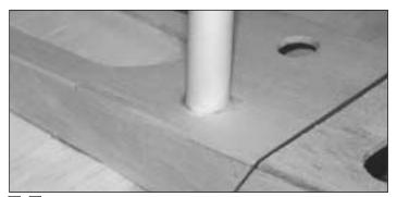
□ □ 10. Mount the wing to the fuse with both wing bolts. Fit the **paper tube** through the belly pan bottom and around the head of the right wing bolt, flush against the wing bolt plates. Glue the paper tube to the belly pan bottom and wing bolt plate with medium CA. **NOTE:** Be careful not to glue the wing bolts to the wing.
