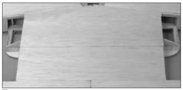
$\Box$  11. Use two 1/16" x 3" x 30" balsa sheets to sheet the top center section of the wing.
