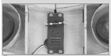
□ 10. Plug your retract servo into your receiver. Set it so that the servo arm, in the "up" position, is positioned rotated slightly as shown in the photo. Make sure it rotates clockwise to move the gear down.
