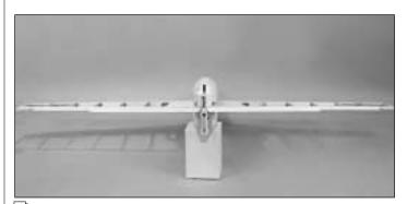
□ 3. Stand about six to ten feet behind the model and see if the stab is parallel with the wing. If necessary, sand the stab base with a thin sanding block until the stab is parallel with the wing.
