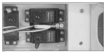
□ 12. While keeping both elevators centered, connect the two elevator pushrods to each other with two 5/32" wheel collars and  $6-32 \times 1/4$ " hex head cap screws as shown in the photo. We recommend using thread locking compound on the cap screw threads.
