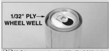
□ 32. Select or cut a piece of 1/32" x 2" x 8-3/4" ply (not included) with the grain running the short way. Wrap it around a soda can of your choice, allow the sheet to overlap and glue the sheet to itself. This will be the wheel well.
