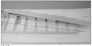
$\Box$  2. Edge glue a 1/16" x 3" x 30" sheet to the LE the same as you did for the bottom of the wing.
