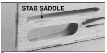
☐ 7. You're about to mix epoxy to work on the aft end of the fuselage. Before you do so, test fit the die-cut 1/8" ply **stab saddle**. Lightly sand as needed for a perfect fit. Temporarily remove the stab saddle.
