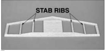
$\Box$  6. From a 3/16" x 1/4" x 12" balsa stick, cut, fit and glue the stab ribs in place.
