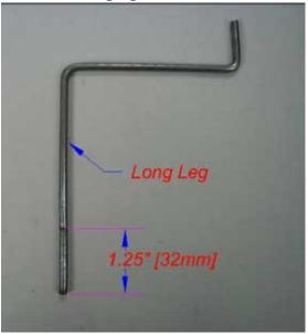
□ 2. Draw a line 1-1/4" [32mm] away from the end of the long leg as indicated above on both main landing gear wires.
