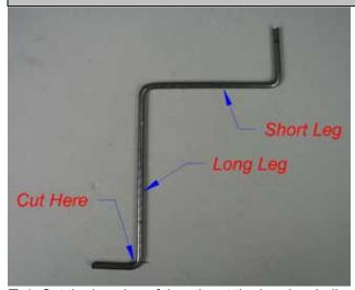
☐ 1. Cut the long leg of the wire at the bend as indicated above on both landing gear wires.
