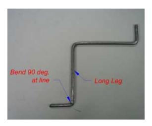
$\square$  3. Bend each wire 90 degrees at the line as shown above. Install the wire as per instructions. The bend just made goes into the wing mounting blocks.
