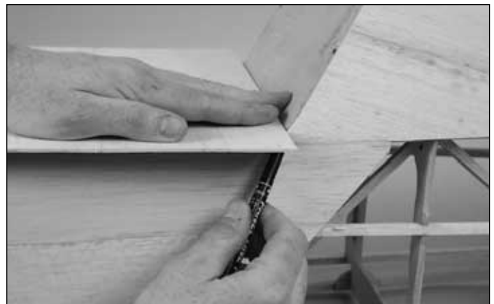
□ 20. Rough cut a slot for the fin approximately 8-5/8" long, 3/4" wide at the trailing edge. Removing a little material at a time, cut the slot in the turtle deck sheeting until it properly fits the fin. Note: Take your time and be patient, fitting the fin as you go.
