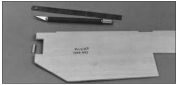
☐ 2. Use a straightedge and a ballpoint pen to draw a line across the *tab* connecting the notches in the front of **one** of the **fuselage sides**. Use the line as a guide to remove the tab with a #11 knife blade. As shown in the photo, label this as the **RIGHT** (inside) fuselage side.
