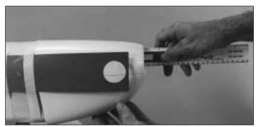
☐ 7. Place the backplate of your spinner on the engine and measure the distance between the firewall and the backplate (it should be 4-3/4"). Remove the engine from the fuselage, then position the cowl on the fuselage so the forward edge is 1/8" aft of the measurement you just made. Use a ballpoint pen to lightly mark the location of the rear of the cowl on the fuselage top.
