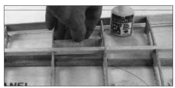
□ □ 10. Starting at ribs R-8 & R-7 test fit, then glue the die-cut 3/32" cross grain balsa **shear webs** to the front of the spars. Note that the shear webs increase in height as they get closer to the root and there are two shear webs that are the same height between ribs 2 & 3 and 3 & 4.
