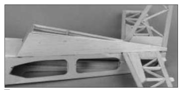
4. Test fit, then use medium CA to glue the bottom of the left side turtle deck only to the aft fuselage top, the bottom stringer and the stab.
