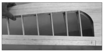
☐ ☐ 16. Mark the location of the hinges on the aileron and the wing. Cut the hinge slots, then test fit the aileron to the wing with the hinges.
