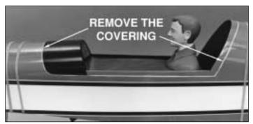
☐ 3. Use a sharp #11 blade to *carefully* cut the covering about 1/32" inside of the line you marked **without cutting into the balsa**. Wipe away the ink line with a paper towel lightly dampened with alcohol.
