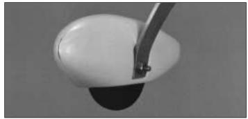
☐ ☐ 11. Temporarily mount the wheel pant to the landing gear with another 8-32 nut on the axle.
