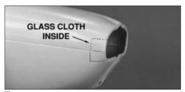
☐ 5. Use 30-minute epoxy to glue a 1" strip of glass cloth across the glue joint inside the front of the cowl on both sides.
