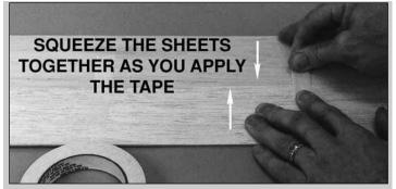
B. Use masking tape to tightly tape the two sheets together joining the trimmed edges.
