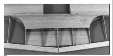
11. Use the 18-3/4" balsa sheet left over from step 7 to sheet the front portion of the bottom center section. Use your pattern to cut the curve at each end.
