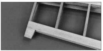
■ 8. Use your bar sander to sand the ends of the wing flat and even with ribs R-10.
