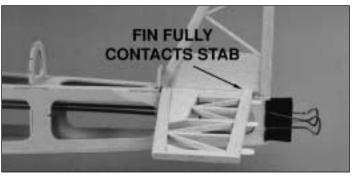
9. If you haven't already done so, final sand the fin. Test fit the fin on the stab with the trailing edge of the fin between the fuselage sides. Adjust the length of the fin trailing edge so the base of the fin fully contacts the stab.
