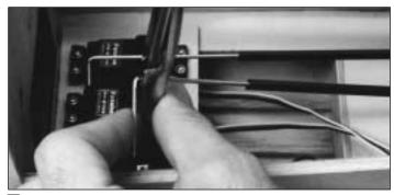
☐ 11. Disconnect the clevises from the control horns, then make a 90 degree bend at the marks you made. Temporarily install a nylon Faslink on each pushrod, then cut the wire so it slightly protrudes out of the Faslink.
