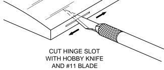
☐ 3. Cut the hinge slots in the elevator and stabilizer using a #11 blade. Begin by **carefully** cutting a very shallow slit at the hinge location to accurately establish the hinge slot.
