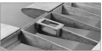
☐ 6. Use medium CA to glue the aileron servo tray and supports in position, then glue the die-cut 1/8" plywood aileron servo tray doublers to the bottom of the aileron servo tray.
