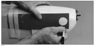
8. Align the cowl with the mark you made on the fuselage, then use a felt-tip pen to transfer the hole in the template onto the cowl.
