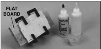
☐ 1. Use 30-minute epoxy to glue the **firewall formers** F-1A, F-1B and F-1C together. Make sure the **embossed label** on each former is facing **forward** and the top edges and notches of each former are aligned. Wipe away excess epoxy before it cures. From now on this assembly will be referred to as the **firewall**.
