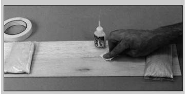
C. Turn the sheet over and place weights on top of the sheet to hold it flat. Apply thin CA sparingly to the seam between the two pieces quickly wiping away excess CA with a paper towel as you proceed.
