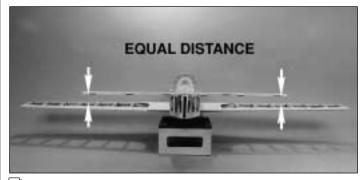
☐ 2. Mount the wing to the fuselage, then position the stab on the fuselage. Stand about six to ten feet behind the model and see if the stab is parallel to the wing. If necessary, use your bar sander to make adjustments by sanding the stab base until the stab is in alignment with the wing.
