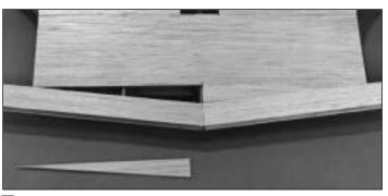
☐ 15. Fit, then glue the four 1-1/2" x 6" sheets to the aft portion of the top and bottom center section of the wing. Save the two 1-1/2" x 12" sheets for the wing belly pan which will be built after the wing is mounted to the fuse.
