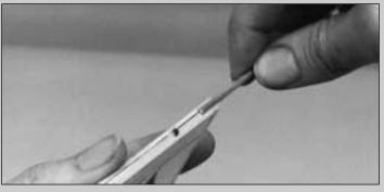
B. Use the sharpened tube to *carefully* gouge the leading edge of the elevators. You'll have to make a few cuts to make the recess deep enough for the joiner wire.
