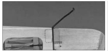
☐ 17. Cut a slot in the trailing edge of the fin at the marks you made for the nylon tail gear bearing. Without using any glue join the rudder to the fin with the tail gear wire.
