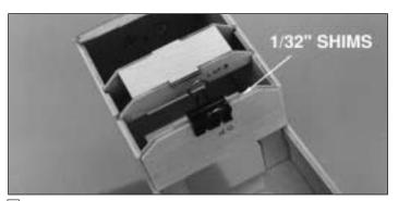
☐ 1. With the punch marks facing forward, temporarily clamp the dowel plate (DP) to F2-B so the edges align, with an approximately 1/32" shim in between. You may use playing cards, business cards or similar thin card stock for the shim. Place the wing in the fuselage. The wing should be nearly final sanded at this point.
