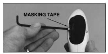
C. Use a 9/64" hex wrench to screw the axle through the wheel and the wheel pant until the wheel goes all the way in and the axle goes through the pant mount.
