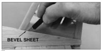
☐ 6. Once you can bend the sheet all the way around the formers and to the top stringer, use a sharp #11 blade to shave a bevel to the top edge of the sheet where it meets the fin. Notice that the angle of the bevel becomes more vertical toward the rear of the fin.
