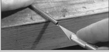
A. Use a #11 knife blade to sharpen the end of a piece of 1/8" brass tube. Roll the tube as you *carve* the end. If you have a file or a cut-off wheel it helps to sharpen the outside of the end of the tube as well.
