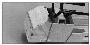
☐ 22. Use 30-minute epoxy to glue the landing gear plates to LGF-A and B and LGF-A and B to the fuselage sides. Without using any glue, **temporarily** install the tank floor to set the position of LGF-A.
