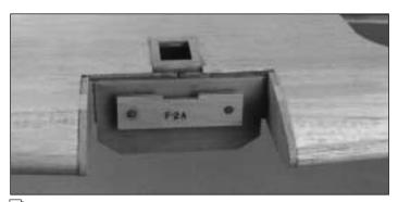
☐ 12. Drill a 1/4" hole through the punch marks in F-2A. After the epoxy from the previous step has fully cured, test fit F-2A on the wing dowels (it doesn't matter which way the notch faces). Make adjustments to the holes in F-2A if needed.
