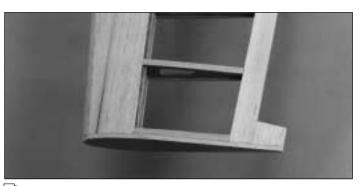
☐ 10. Cut the wing tips from the sheet slightly oversize, then use medium CA to glue them to the wing. Use your bar sander to shape the wing tips to match the contour of the wing.
