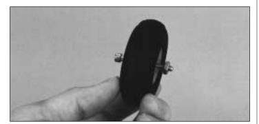
A. Install an axle in a wheel, then thread an 8-32 nut on the axle about 1/8".
