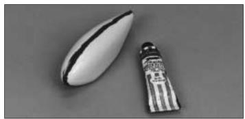
☐ 13. Before painting the wheel pants fill the seams with putty filler such as Squadron White Putty or resin filler such as Bondo. We use Bondo most of the time as it cures quickly and is easy to sand but usually it must be purchased in large quantities. Squadron putty works well but it takes overnight to dry and usually requires at least two applications because it shrinks as it dries.
