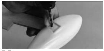
□ □ 8. Drill a 3/16" (11/64" or #18 for precision) hole in the wheel pant at the mark. Back up the wheel pant mount with a piece of plywood so you do not split it as the drill goes through.
