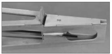
☐ 28. Glue the pushrod tubes to the slots at the end of the fuselage with microballoons and epoxy. Completely fill the
