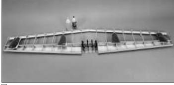
• 6. Glue the spar joiners to the spars with 30-minute epoxy by spreading a film of epoxy on both the spars and the spar joiners. Once the C-clamps are tightened wipe away excess epoxy. Place waxed paper under the center of the wing to catch excess epoxy and place weights on top of your wing to hold the jig tabs down. Glue the TE's together with thin or medium CA. Do not disturb the wing until the epoxy cures.
