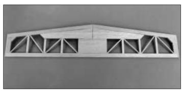
7. Remove the stab from your building board. Inspect all the glue joints and add CA to any joints that don't look strong. Cut the ends of the leading and trailing edges so they extend past the end of the stab by about 1/16". Use your bar sander to finish the job by sanding the ends of the LE's and TE so they are flush with the end of the stab. Cut the 1/8" x 1/4" tips, then glue them to the end of the stab.
