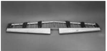
□ 3. Replace the wing on your flat building table so it is resting on the bottom jig tabs. Place weights on top of the wing to hold the jig tabs down. Make the left and right top LE sheets by gluing together two 3/32" x 3" x 30" balsa sheets, then glue them to the top of the wing the same as you did for the bottom.
