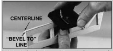
B. Using the bevel to lines and the center line as a guide, make the "V" on the leading edge of the elevators with a razor plane or your bar sander with 150-grit sandpaper.
