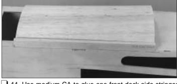
☐ 11. Use medium CA to glue one front deck side stringer to each side of the fuselage. Sand the side stringers so they blend the sheeting and fuse sides together as shown on the fuselage plan.
