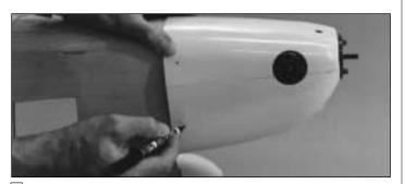
□ 14. Position the cowl on the fuselage using the backplate of the spinner as a guide, then use a felt-tip pen to mark the cowl where to drill the holes for the cowl mounting screws. Drill a 1/16" hole through only the cowl at each mark. Accurately reposition the cowl and use a ballpoint pen to mark the location of the holes in the cowl on the cowl mount blocks.
