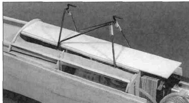
D 5. Test fit the 3/32" x 2-3/8" x 14" balsa top center sheet (SKY6F22) in place between the cabane wires. It should fit from the center of one middle stringer to the center of the other middle stringer. Sand it if necessary to fit between the cabane wires. Glue it in place with CA.
