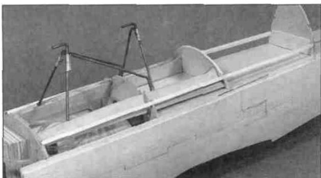
D 3. Install the two outer 3/16" sq. stringers by cutting two 3/16" sq. x 24" balsa sticks (SKY6F26) to fit between F1 and F3 and gluing them in place.
