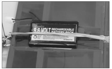
□ 2. With the battery mounted to the fuselage, lift the model upside-down at the balance point. If the **tail** drops, the model is "tail heavy" and you must shift the battery pack forward to balance the model. If the **nose** drops, it is "nose heavy" and you must shift the battery aft to balance the model.
