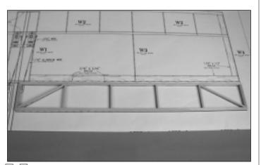
$\Box$  2. Cut the **cross supports** from a 1/8" x 3/16" x 36" [3.2 x 4.8 x 910mm] balsa stick. Glue the cross supports in place using the plan as a guide.
