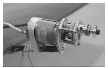
■ 9. Secure the back of the motor to the fuselage with nylon tape or a tie wrap (not included).
