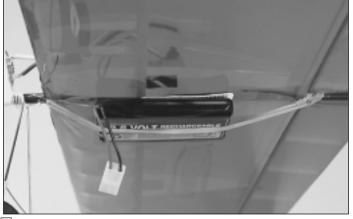
■ 4. Hook two #64 rubber bands around the fuselage tube behind the wing, then connect them to the battery hook. Mount the battery pack between the wing and the rubber bands. Later, the exact location of the battery will be determined to balance the model.
