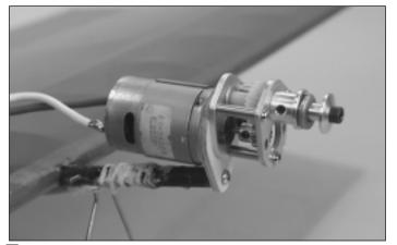
□ 7. Mount the motor and gear box to the motor mount as shown, using the screws included with the system.
