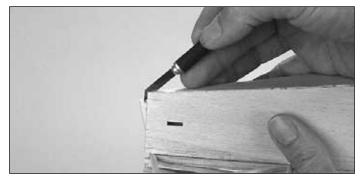
□ 12. Use a thin razor saw to cut a slot in the aft end of the fuse bottom to accommodate the small hinge that will be used to join the bottom of the rudder to the fuse as shown on the plan. Cut a matching slot in the middle of the bottom of the rudder.
