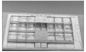
□ 11. Cut the top spars from two more 1/8" x 1/4" x 24" [3.2 x 6.4 x 610mm] balsa sticks and glue them into the notches in the top of the ribs.
