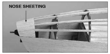
□ 9. Cut and test fit a piece of 1/32" [.8mm] balsa **nose sheeting** to fit over the gearbox. Trim the sheet as necessary for a good fit. Be certain the sheeting is positioned so you will be able to access the top gearbox mounting screw with your screwdriver. Glue the nose sheeting into position. The same as the cockpit sheeting, feather the nose sheeting to the stringers with strips of 1/32" x 1/8" [.8 x 3.2mm] balsa.
