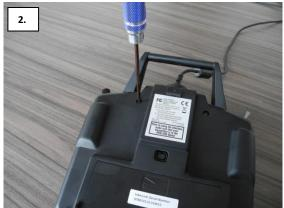
Place the Interlink controller face down (we'd recommend on a cushion or similar to protect the sticks), remove the 4x Philips head screws and carefully remove the controller's rear panel as shown.
