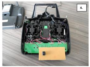
Remove the connector plate
