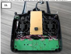
This is how the finished modification should look. Next, carefully replace the controller's rear panel and resecure with the screws. Finally, select the Mode1 option from the drop down menu which is part of the RealFlight software and the conversion is complete.
