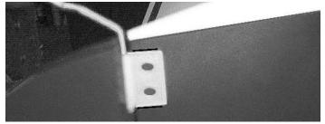
**3.** □ Mark where the tail wheel bracket meets the fuselage
