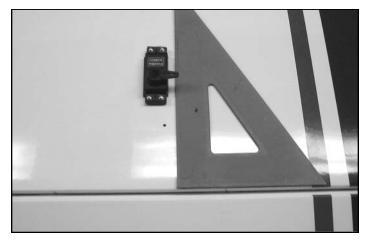
**2.**  $\Box$  With the aileron servo in place, make a mark at a 90° degree angle to the trailing edge and in line with the servo arm.
