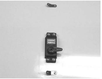
**3.** □ Using #2 x 3/8 sheet metal screw, mount the bracket so that it is pointing to the fuselage.
