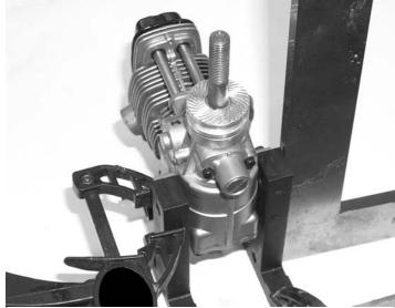
**3.** □ Keeping the engine perpendicular to the table top, clamp the other motor mount to the engine. Mark and drill the second motor mount then screw the mount to the engine.
