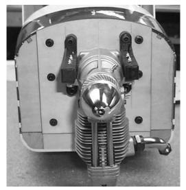
**6.**  $\square$  Mount the firewall plate to the front of the fuselage using the 8-32 x 1/2"
