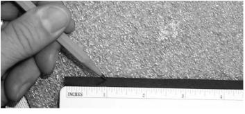
**1.**  $\Box$  Mark 1" up from the bottom of the rudder.
