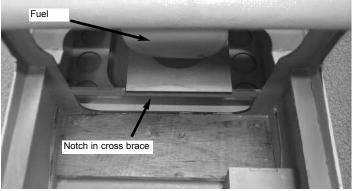
□ Fit the fuel tank into the fuselage
