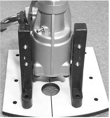
**5.** □ Install the motor mount beams on to the firewall plate using the 8-32 x 3/4" socket head screws and washers and 8-32 blind nuts
