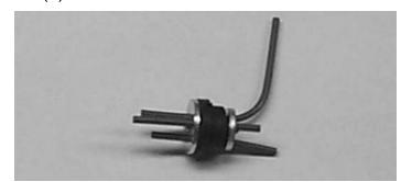
1. □ Insert the 3mm screw through the center hole in the large washer, through the center hole in the rubber washer against the large side, and screw the small washer on the back side.
