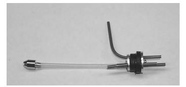
3. □ Install the 4mm silicone tube to the short brass tube and install the clunk to the other end of the silicone tube. This is the fuel pick-up and must be free to "flop" around in the tank so it can pick up fuel in any attitude.
