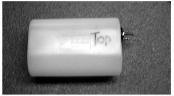
4. □ Install the assembly into the tank so the vent tube is turned up to the top of the tank and is positioned on the right side of the tank. Tighten the screw to expand the rubber cap. Don't over tighten or you could split the tank.
