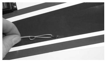
**9.**  $\Box$  Insert the throttle tubing into the rear cable exit hole.
