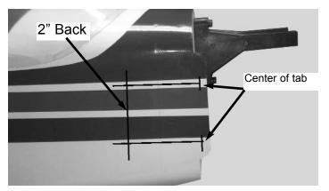
1. □ Make a mark 2" back from the middle front tabs on the fuselage sides in each of the white stripes.
