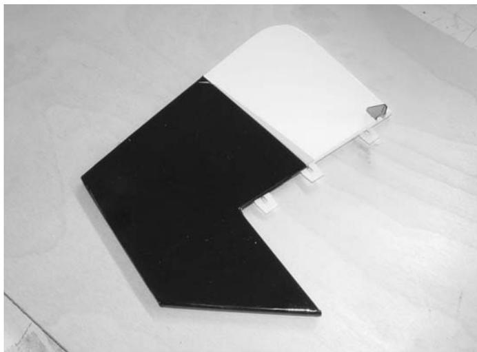
3.  Locate the rudder and install 3 CA hinges, do not glue yet.
