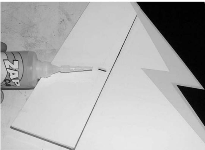
6.  Flip the wing over and glue the aileron horn from the top side of the wing using thin CA.
