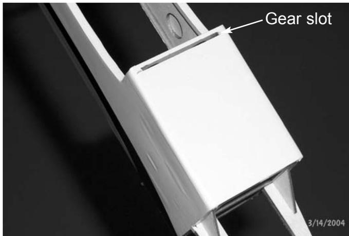
2.  Remove the covering from the landing gear slot at the leading edge of the wing.
