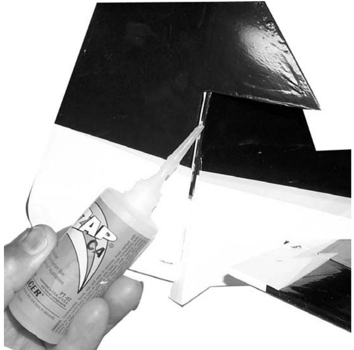
4.  Install the rudder on the plane using straight pins to make sure the hinges stay centered just as we did with the elevators.
