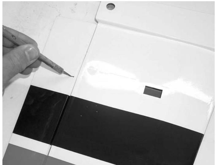
3.  Use an X-acto knife or razor blade and remove the covering over the control horn opening. Do this on both sides of the aileron.
