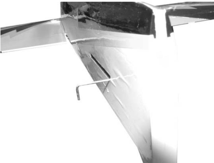
2.  Slide the elevator joiner wire into the slot for the stab. You cannot install it after the stab is in place without cutting the fuselage.
