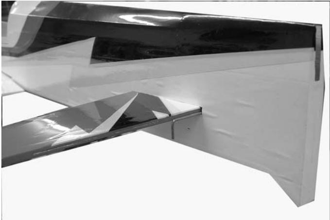
3.  Slide the stab into the precut slot in the fuselage. Measure each side at the trailing edge to make sure it is centered.
