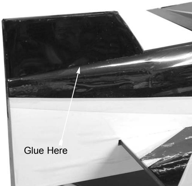
2.  Insert fin in the slot on top of fuselage and glue in place using thin CA.
