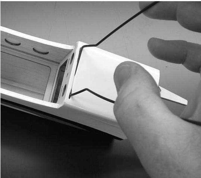
3.  Flex the landing gear legs together slightly and slide in the opening. Push all the way in.
