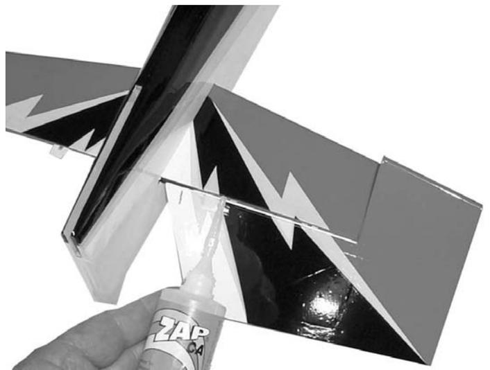
10.  Remove the pin and push elevator tight against the stab. Deflect the elevator to its full travel in the down position. Apply one drop of thin CA on each hinge.
