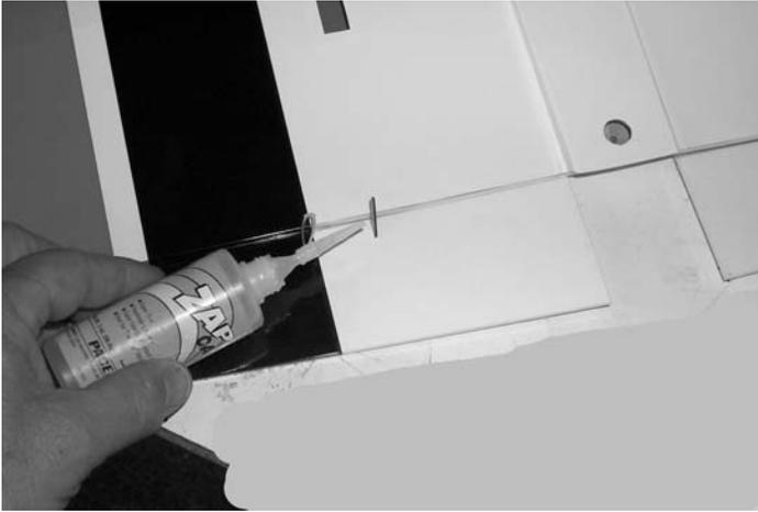
5.  Using thin CA, apply one drop on each side of the control horn.
