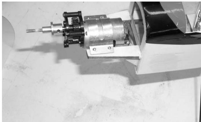
3.  Place the top shell in place and secure using the four #2x1/2" screws.
