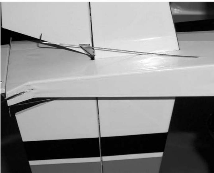
3.  Bend a 90 degree angle 1/4" long in the end of one of the 1/32" x 24" pushrods.
