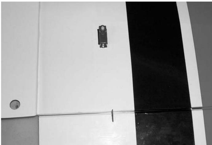
13.  Screw the servo in place using the hardware supplied with the radio.
