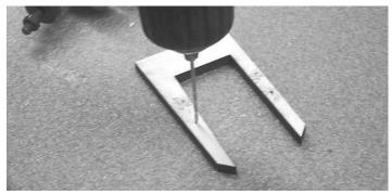
**5.**  $\Box$  Drill the engine mounting holes in the plate.
