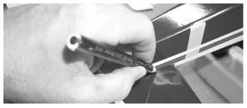
**5.**  $\Box$  Mark the bottom of the stab along the fuse-lage.
