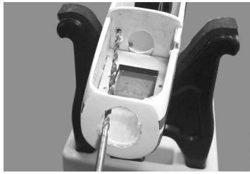
**6.**  $\Box$  Drill the hole for the engine throttle pushrod.
