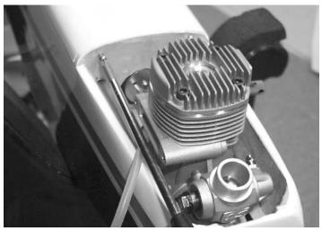
1. □ install the fuel tank hatch on top of the fuselage with 2mm sheet metal screws on both sides of the fuselage.
