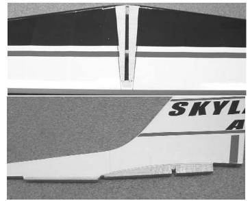
6. □ Remove the stab from the fuse and, working 1/8" inside the drawn lines, carefully remove the covering from the bottom of the stab, both sides of the fin and the top of the fuselage. BE CAREFUL TO AVOID CUTTING THE WOOD
