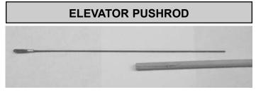
**2.**  $\square$  Remove the metal clevis from the end of a 1.5 x 25cm wire.
