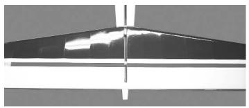
**3.** □ Place the stab on the fuse and align the center slot with the front slot and the rear of the fuselage.
