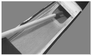
**3.** □ Insert the rudder pushrod into the fuselage through the wing saddle area.
