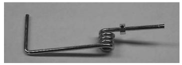
3. □ Slide a wheel collar with a set screw onto the top of the nosegear gear strut.
