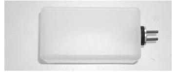
5. □ Install the assembly into the tank so the vent tube is turned up to the top of the tank and is positioned on the right side of the tank. Tighten the screw to expand the rubber cap. Don't over tighten or you could split the tank.
