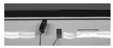
**2.**  $\Box$  Plug the servo extension wire into the servo if required.
