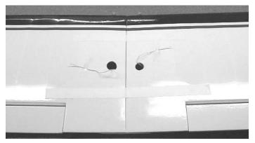
**4.** □ With masking tape, tape the wing halves together at the trailing edge and close to the leading edge, as shown. This will help keep the wing from twisting.
