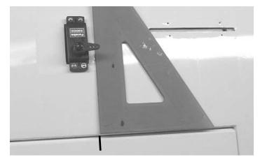
2. 🗆 With the aileron servo arm in place, make a mark at a 90° degree angle to the trailing edge and in line with the servo arm.
