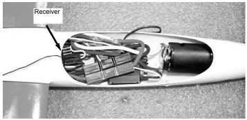
Plug in all the servos into the micro receiver and place the receiver on top or in front of the battery pack.
