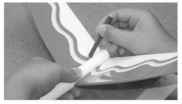
1. □ Using a soft lead pencil, mark the location where the stab meets the fuselage.
