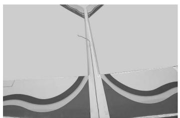
Stretch out the receiver antenna along the top of the fuselage and tape in place. You will also have to tape the wings to the fuselage before flying.
