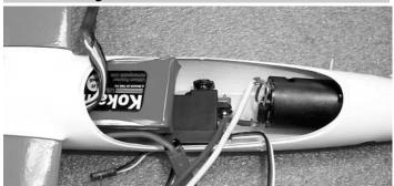
Slide the battery behind the elevator servo. Use foam to help hold the battery in place or glue velcro on the battery and the tray.
