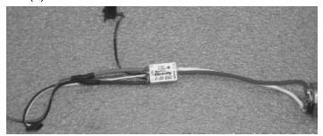
Solder your speed control onto the motor, by following the instructions that came with your speed controller.
