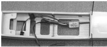
Insert the speed control and motor assembly through the front of the fuselage and into the main cabin of the fuselage.
