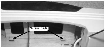
Drill a hole through the canopy and into the rear mounting pad. You could also use the front pads if you do not want to tape the front of the canopy to the fuselage.
