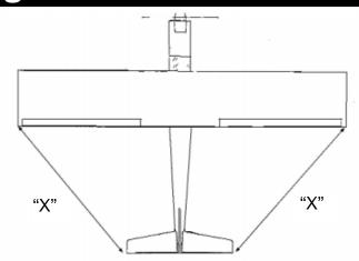
**4.**  $\square$  Measure from the end of the wing to the tip of the stab. This measurement should be the same for both sides.
