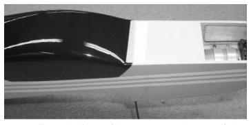
Tape the front of the canopy to the top of the fuselage then tape the rear using a tab on the tape. OR, -
