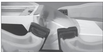
4. Finally, re-mount the windshield and remove any excess adhesive. Secure a clamp or clamps to each side of the windshield and allow glue to cure for at least 3 hours or for best results overnight.
