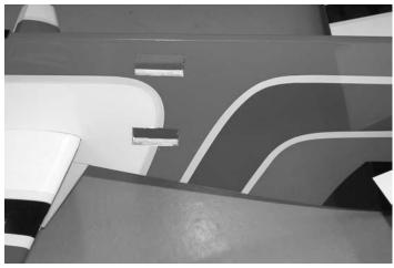
USING A SHARP KNIFE OR RAZOR BLADE, REMOVE THE COVERING FROM THE SERVO CUTOUT JUST AHEAD OF THE STAB ON BOTH SIDES OF THE FUSELAGE.
