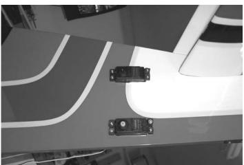
INSTALL THE RUDDER AND ELEVATOR SERVO IN THE CUTOUTS USING THE HARD-WARE SUPPLIED WITH THE RADIO. THEY WILL BE ON THE LEFT SIDE OF THE PLANE.
