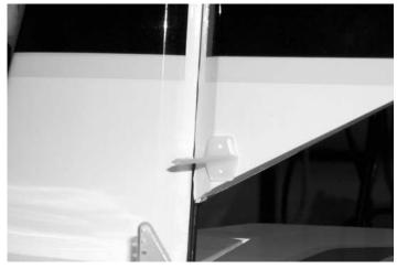
ALIGN THE ELEVATOR HORN ON THE INSIDE EDGE OF THE ELEVATOR AND MOUNT USING THE TWO #2x1" SCREWS AND NYLON PLATE.
