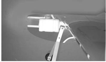
LOCATE THE FUEL TANK AND POSITION IT ON THE LEFT SIDE OF THE FUSELAGE. MARK THE LOCATION OF THE HOLES FOR THE TIE WRAPS AT THE TOP AND BOTTOM OF TANK ALIGNED WITH THE GROVES IN THE TANK. PAY ATTENTION TO THE LIGHTNING HOLES IN THE FRONT OF THE FUSELAGE UNDER THE COVERING AND MAKE SURE YOU ARE NOT OVER ONE OF THEM. DRILL A 3/16" HOLE AT THE FOUR LOCATIONS MARKED. TWO PIECES OF BALSA ARE SUPPLIED TO SPACE THE TANK OUT FROM THE FUSELAGE.
