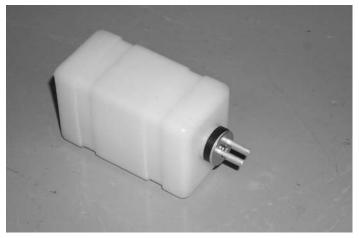
INSTALL STOPPER IN TANK AND TIGHTEN THE BOLT IN THE CENTER UNTIL STOPPER IS SNUG. DON'T OVER TIGHTEN. CLUNK SHOULD MOVE FREELY AND VENT TUBE SHOULD BE TO THE TOP OF THE TANK.
