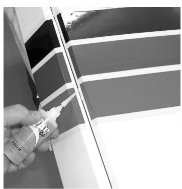
INSTALL THE AILERONS ON THE WING AND GLUE IN PLACE BY DEFLECTING THE AILERON FULLY IN ONE DIRECTION AND APPLY TWO DROPS OF THIN CÅ ON EACH HINGE. TURN THE WING OVER AND REPEAT ON THE OTHER SIDE.
