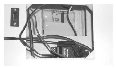
THE BATTERY WILL MOUNT ON THE LEFT SIDE. WRAP WITH FOAM RUBBER(NOT SHOWN FOR CLARITY) AND INSERT INTO OPENING.
