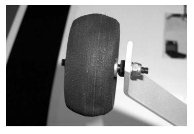
INSTALL THE AXLE IN THE ALUMINUM GEAR AND SECURE WITH A 8MM FLAT WASHER AND LOCK NUT. INSTALL ONE OF THE WHEEL COLLARS, THE MAIN WHEEL AND SECURE ON THE OUTSIDE WITH THE OTHER WHEEL COLLAR.
