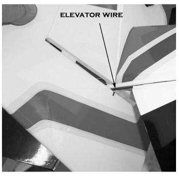
FIT THE RUDDER IN PLACE ON THE FIN AND MARK THE LOCATION OF THE ELEVATOR WIRE.
