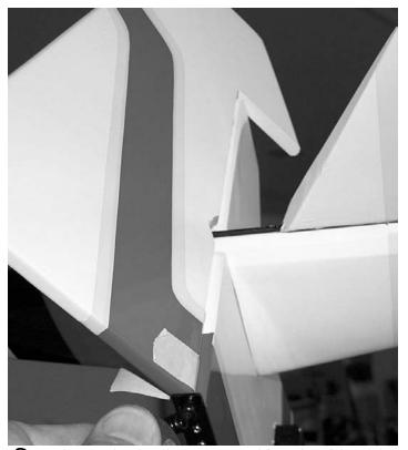
SLIDE A PIECE OF MASKING TAPE BETWEEN THE TAIL WHEEL WIRE AND THE FIN POST. PUT EPOXY GLUE IN THE HOLE AND SLOT ON BOTTOM OF RUDDER WHERE THE TAIL WHEEL WIRE GOES IN. INSTALL THE RUDDER ON THE CA HINGES WITH THE TAIL WHEEL WIRE IN PLACE AND PULL THE MASKING TAPE AROUND TO HOLD THE GLUE IN.
