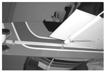
YOU WILL NEED A 12" SERVO EXTENSION FOR BOTH RUDDER AND ELEVATOR SERVOS. FIT THE WIRES INTO THE COVER, AND LEADS INTO THE OPENING IN THE WING. SECURE THE COVER IN PLACE WITH THE TWO METAL BRACKETS AND FOUR 2.5mmx 10mm screws. Drill a 1/16" PILOT HOLE AND HARDEN WITH THIN CA.
