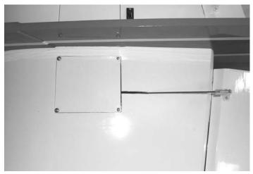
AFTER ALL WIRES ARE PLUGGED INTO RECEIVER AND BATTERY PACK INSTALL THE COVERS BY DRILLING A 1/16" PILOT HOLE THROUGH THE HOLE IN THE COVER AND ATTACH USING THE FOUR 2.5MM X 8MM WASHER HEAD SCREWS.
