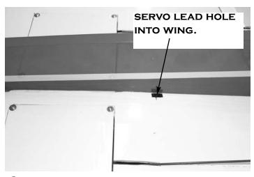
CUT A HOLE NEXT TO FUSELAGE LARGE ENOUGH TO GET THE SERVO PLUGS THROUGH BUT NOT SO WIDE AS THE COVER WILL NOT HIDE IT.
